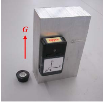
Figure 57 Accelerometer calibration: align one axis of IMU with gravitational reaction force
