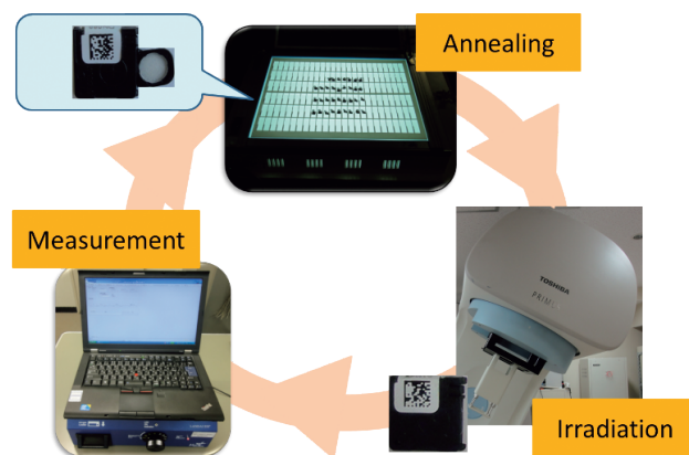
Fig. 2 Measurement cycle. The nanoDot OSLD can be read multiple times; after measurement, annealing can be repeated as many times as necessary.
