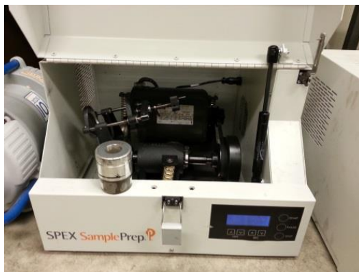
Figure 25: High energy mechanical mill from SPEX CertiPrep.
