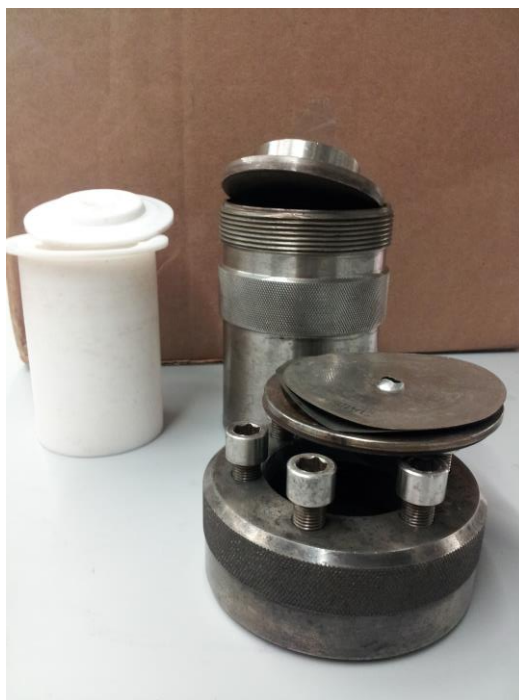
Figure 27: Autoclave used for hydrothermal reactions
