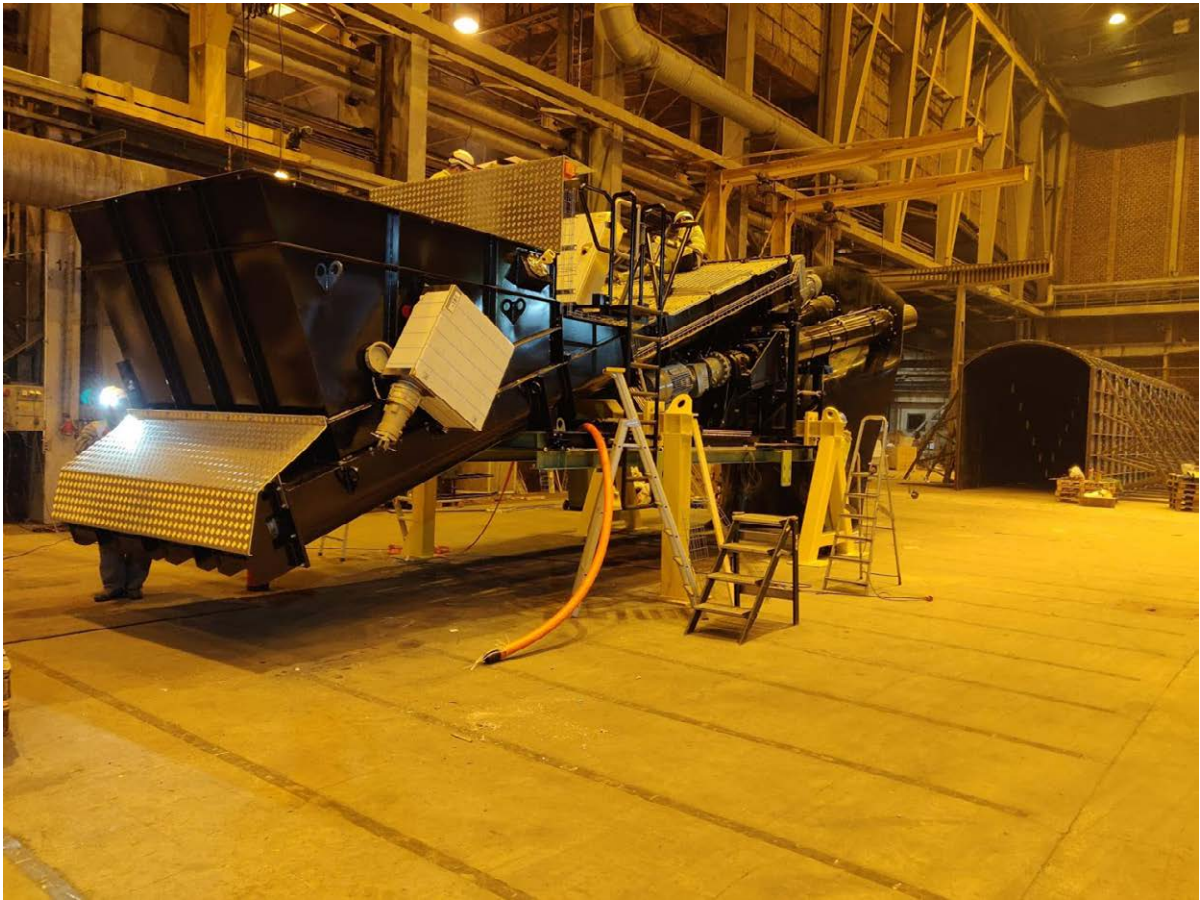
FIGURE L3-6. Granule backfilling test.
