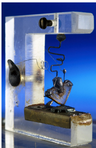
Figure 2.3: First point contact transistor represented by Brattain and Bardeen [44].
