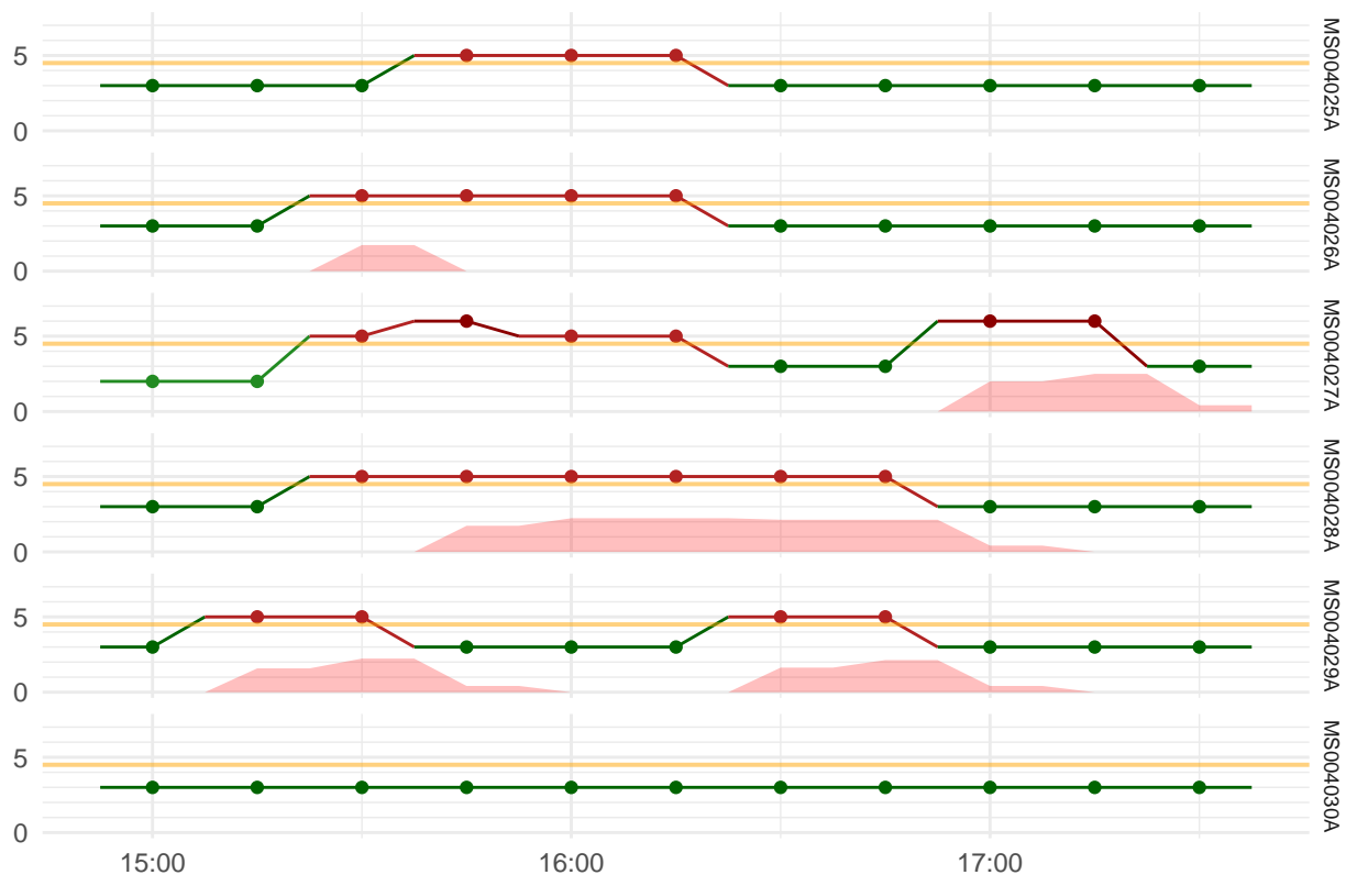
Figure 8.11: An incident occurring in the M4 motorway between MS004028A and MS004029A at 15:15 (6th January 2016). Traffic states [1 - 7] and incident score [0, 5] are shown.
