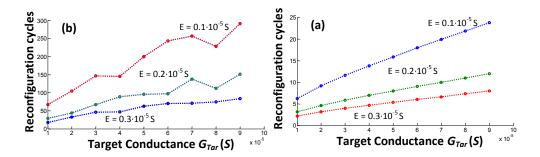
Figure 35: Average (a) and Worst-case (b) reconfiguration cycles to reach target conductance with different absolute error E.
