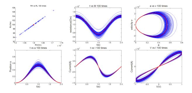
Figure 12: Simulation results for TiO<sub>2</sub> thin-film memristors. The blue curves are from 100 Monte-Carlo simulations, and red lines are the ideal condition. From top left to right bottom, the figures are  $R_H$  vs.  $R_L$ ; M(t) vs. t; v vs.  $\omega$ ;  $\omega$  vs. t; I vs. t; and I - V characteristics.
