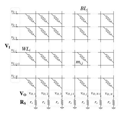
Figure 49: A memristor cross-point array
