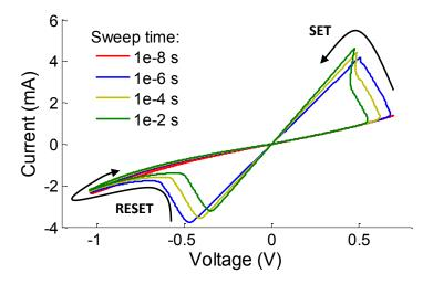
Figure 42: The I-V curve of a  $TaO_x$  device. Reproduced based on Strachan et al. (2013).
