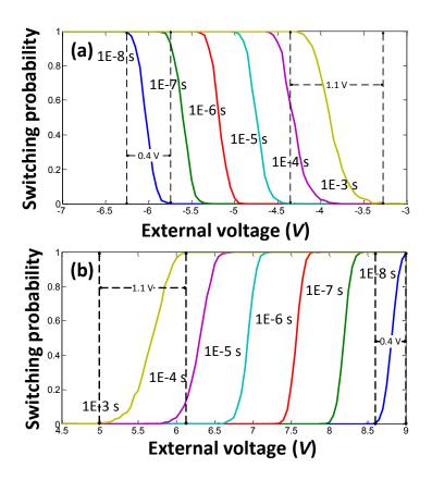
Figure 38: Voltage dependency of ON (a) and OFF (b) switching at different pulse widths  $t_{switch}$
