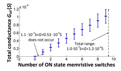
Figure 33: The conductance distribution of parallel connected memristive switches.
