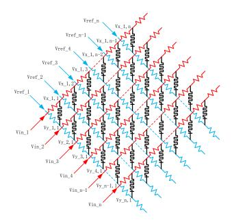
Figure 26: Memristor crossbar model
