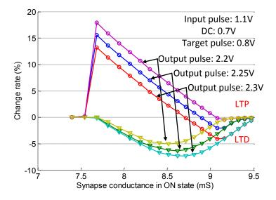
Figure 71: The MST synapse conductance change rate vs. its initial state.
