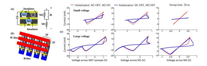
Figure 41: MST synapse design and I-V characteristics. (a) MST structure and equivalent circuit; (b) Conceptual layout in cross-point array; (c) DC-sweep I-V curves of the MST synapse,  $M_1$ , and  $M_2$  when applying a small voltage (top figures) or a large voltage (bottom figure).
