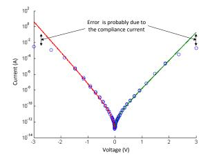
Figure 28: I-V curve of selector model based on TiN tunnelling device, the fitting error at high voltage probably comes from the compliance current limitation.
