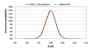
Figure 14: The Distribution of  $R'_L$  from 10,000 Monte-Carlo simulations and the fitting curve of Eq. (3.25).
