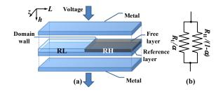
Figure 3: TMR-based spintronic memristor. (a) structure, and (b) equivalent circuit.
