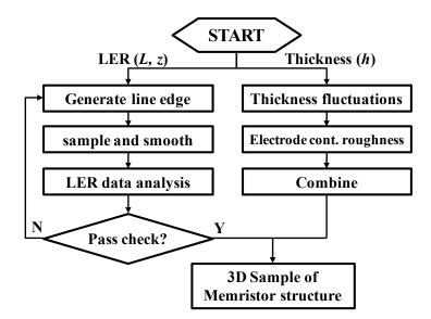
Figure 10: The flow of 3D memristor structure generation including geometry variations.
