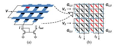
Figure 34: (a) A macro cell containing of 9 memristive switches on a 3x3 crossbar. (b) Partitioning a 6x6 memristive switch crossbar to obtain a 2x2 macro cell crossbar for continuous weight storage.
