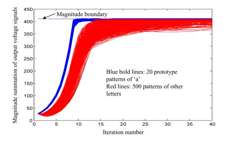
Figure 61: Experiment 2: Iteration number vs. magnitude summation of output voltage signals.
