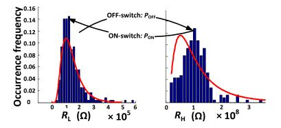
Figure 22: The static state distribution of a  $TiO_2$  memristor device.
