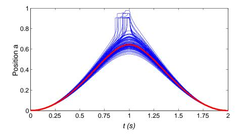
Figure 16:  $\omega'(t)$  when  $V_{ap} = 1.1V$  based on 100 Monte-Carlo simulations.
