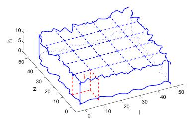
Figure 8: An example of 3D  $\text{TiO}_2$  memristor structure, which is partitioned into many filaments in statistical analysis.
