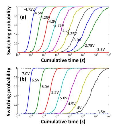
Figure 23: The time dependency of ON (a) and OFF (b) switching at different external voltage V.
