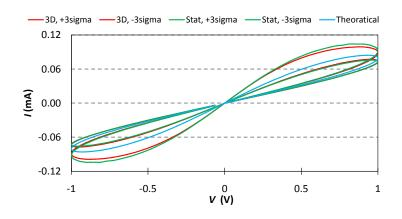
Figure 19: Comparison of I-V at  $\pm 3\sigma$  corners.
