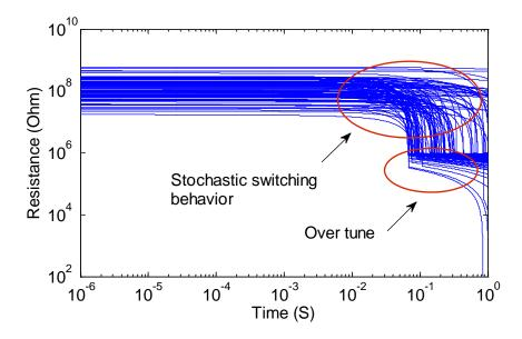
Figure 24: The analog switching process of a  $TiO_2$  memristor.
