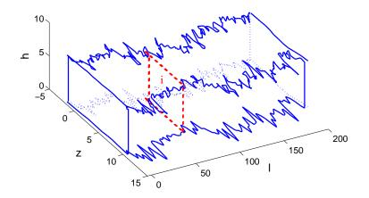
Figure 9: An example of 3D TMR-based spintronic memristor structure, which is partitioned into many filaments in statistical analysis.
