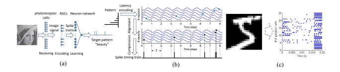
Figure 6: A spike-timing-based model for spatio-temporal pattern recognition. (a) The overview of the spike-timing-based model for vision system; (b) A general LPE flow; (c) An example of spatio-temporal pattern conversion: the image "5" is partitioned and converted to multiple spike-timing trains.
