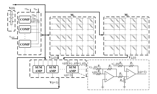
Figure 50: The conceptual diagram of the BSB recall circuit.
