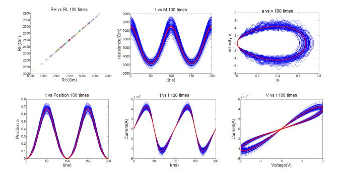
Figure 13: Simulation results for spintronic memristors. The blue curves are from 100 Monte-Carlo simulations, and red lines are the ideal condition. From top left to right bottom, the figures are  $R_H$  vs.  $R_L$ ; M(t) vs. t; v vs.  $\omega$ ;  $\omega$  vs. t; I vs. t; and I - V characteristics.
