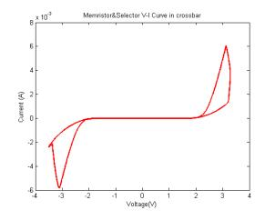
Figure 29: I-V curve of Nonlinear device with TaOx memristor in series connection with the TiN selector.
