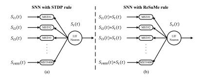
Figure 72: A spiking neural network with 400 synaptic inputs and 1 LIF output neuron and the spike configurations for (a) STDP rule or (b) ReSuMe rule.
