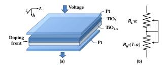
Figure 2:  $TiO_2$  thin-film memristor. (a) structure, and (b) equivalent circuit.
