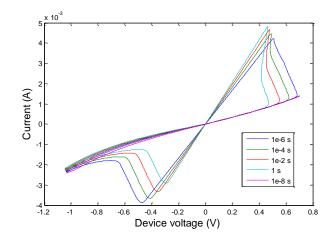
Figure 27: I-V curve of TaOx memristor device compact model
