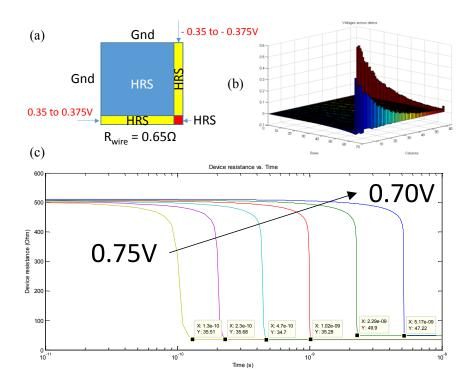
Figure 31: Simulation examples. (a) Simulation setup; (b) Static simulation result of voltage map for 64-by-64 linear cross-point array; (c) Dynamic simulation result of voltage on selected device for 4-by-4 linear cross-point array.
