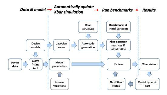
Figure 25: Matlab simulation flow
