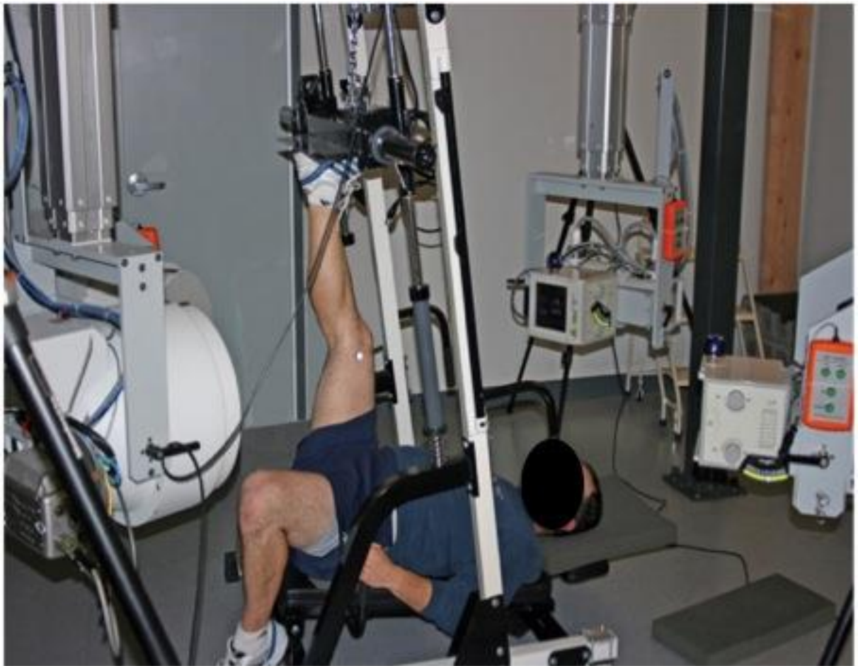
Figure 12. Modified leg press used in kinematic testing
