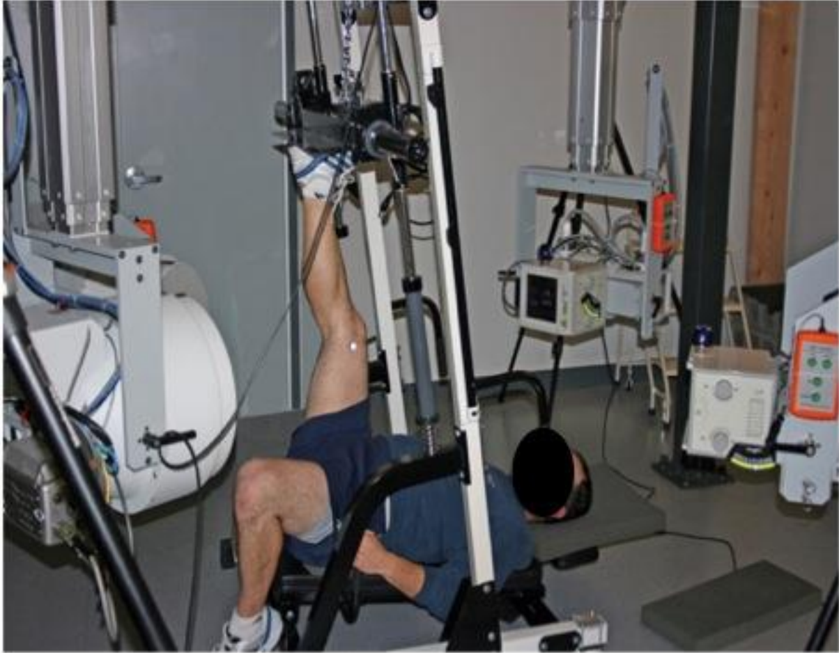
Figure 26. Modified leg press used in kinematic testing. Same legpress used in Chapter 2.
