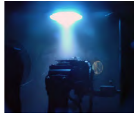
Figure 2 – Magnetron devices are widely used for material processing and surface modification. Crossed electric and magnetic field configuration is used to confine electrons creating dense plasma. The configuration and many physics processes are similar to those in the Hall thruster.
