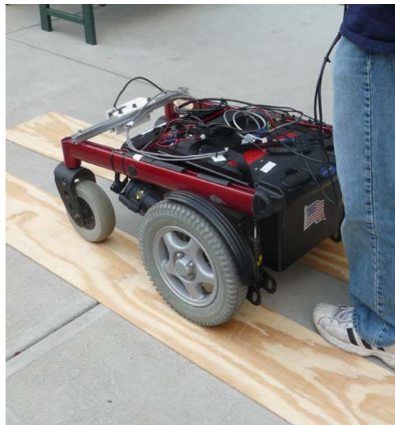
Figure 12: P1 driven over plywood tracks
