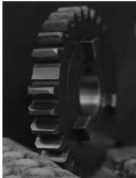
Fig. 4. B4 gear with the broken tooth.
