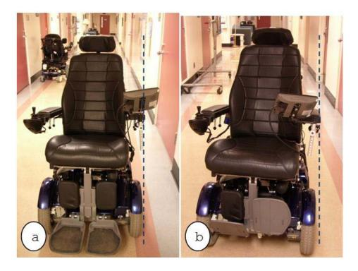
Figure 16. Improvement of the touch screen mount to decrease the width of the system and prevent equipment
