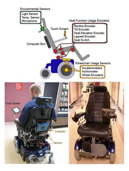
Figure 4. Instrumentation of Virtual Seating Coach System
