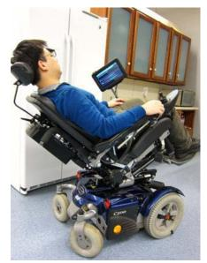
Figure 20. The revision of VSC with a tablet computer
