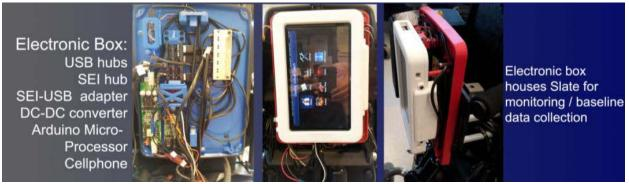
Figure 19. The electronic box which can accommodate the tablet computer if needed
