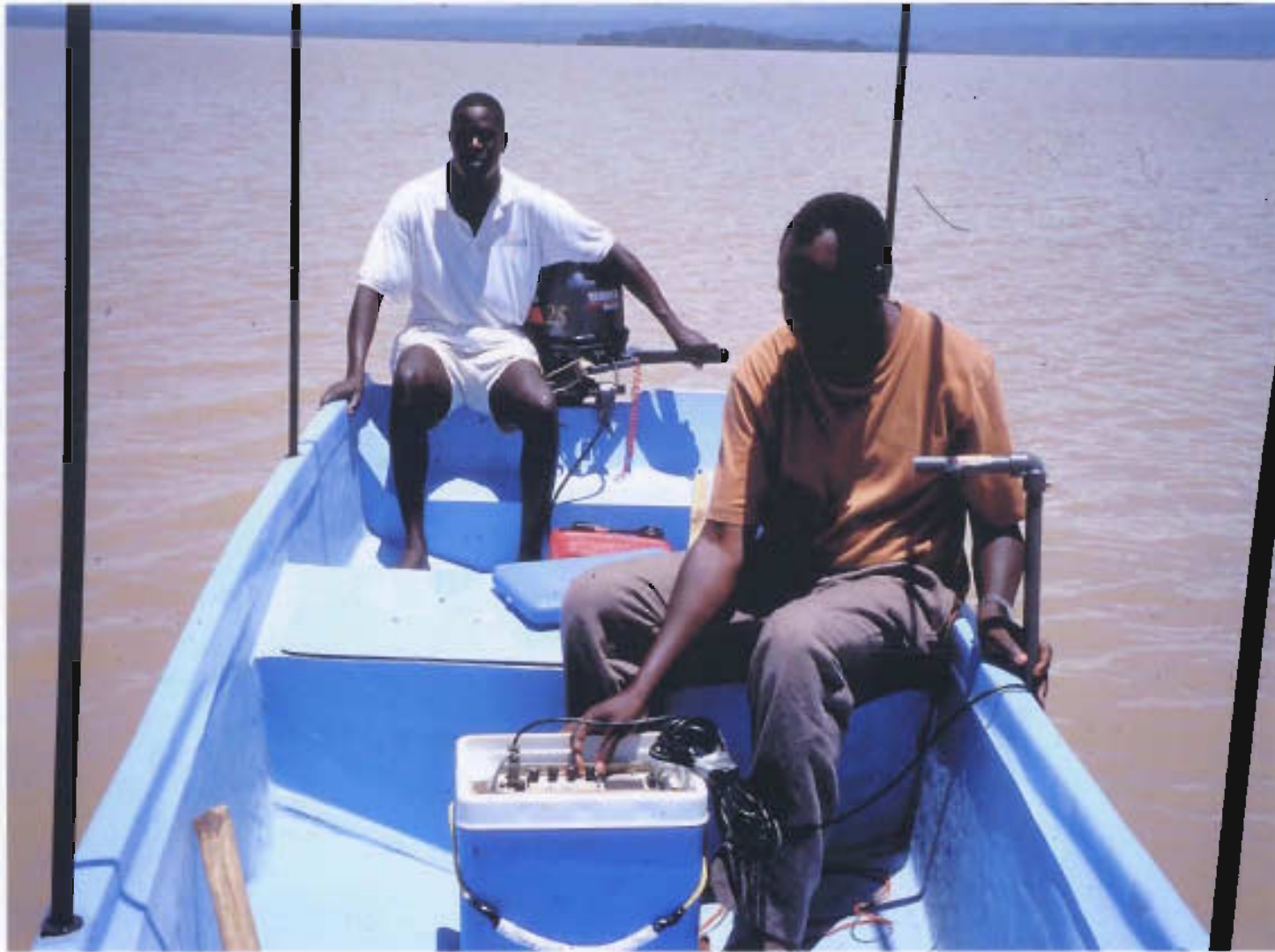
Plate 4.2 Tracking ultrasonic-tagged lungfish in Lake Baringo: tuning in a tag's frequency on the receiver to detect signals from a subject fish using the directional hydrophone immersed in the water.
