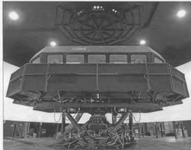
Figure 3.3: 6 degree of freedom motion based simulator
