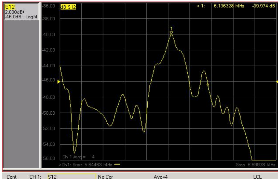
Figure 6. 4 Basic Sensor response of the sample sensor with wireless module (wireless module not connected).
