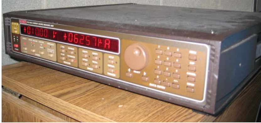
Figure 5. 2 Keithley 238 current source measurement unit.
