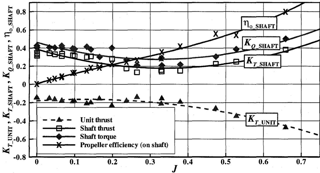
Figure B-25: Open water characteristics for tractor mode at 60° azimuthing angle
