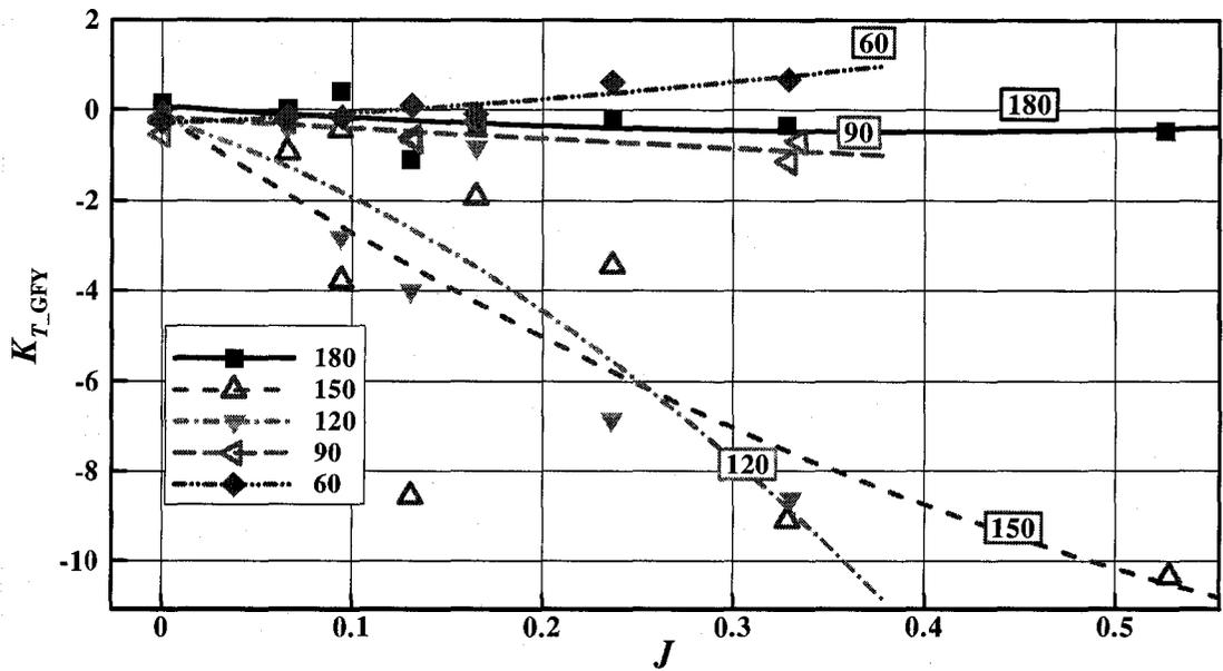
Figure D-9:  $K_{T\_GFY}$  vs.  $J$  at an azimuthing angle of 180 ~ 60 degrees in ice covered water
