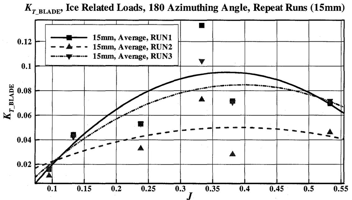
Figure C-24:  $K_{T\_BLADE}$  vs.  $J$ , average ice related loads at 15mm depth of cut (repeated)
