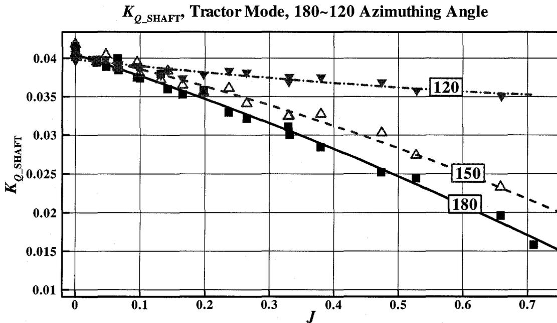
Figure 3-24:  $K_{Q\_SHAFT}$  vs.  $J$  with different azimuthing angles (180-120 degrees)
