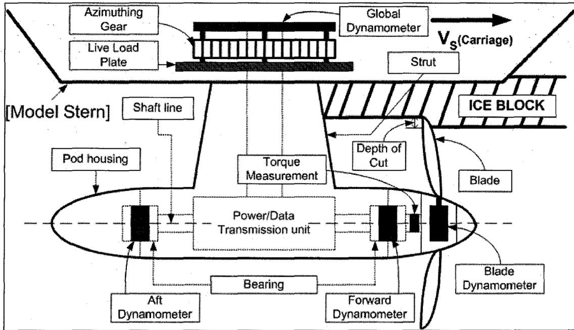
Figure 3-7: Sketch for the model podded propulsor system with measurement devices
