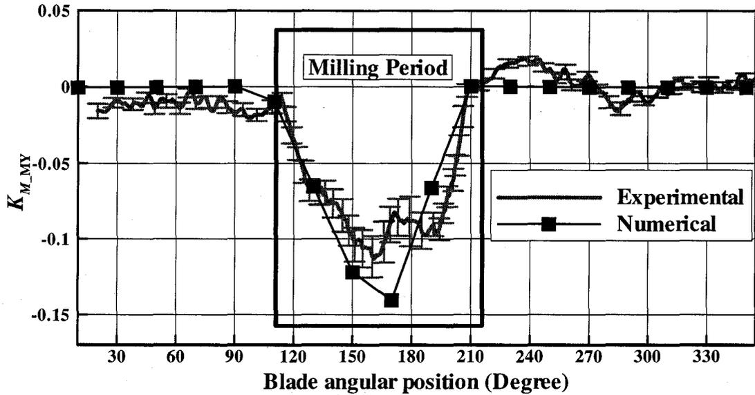
Figure 5-3: Time series comparison for  $K_{M\_MY}$  (ice related loads,  $J= 0.238$ , 35mm)
