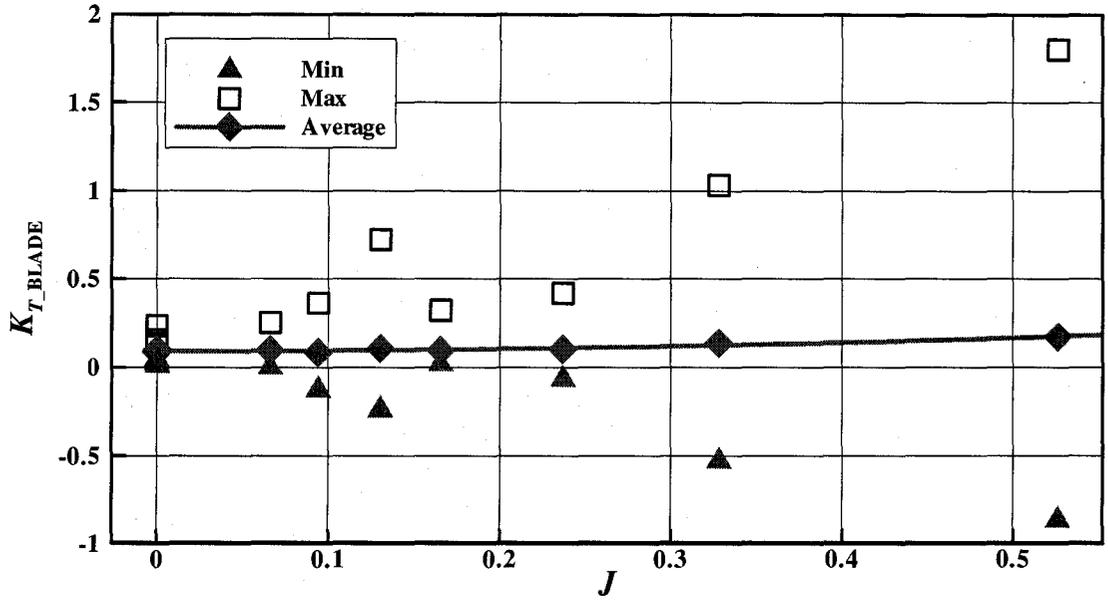
Figure D-6:  $K_{T\_BLADE}$  vs.  $J$  at an azimuthing angle of 180 degrees in ice covered water
