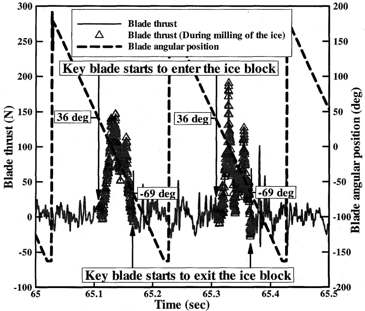
Figure 3-17: Blade thrust during ice milling periods based on the ice milling angle ( $\alpha_m$ : from 36 degrees to -69 degrees, 35mm depth of cut and 5 rps)
