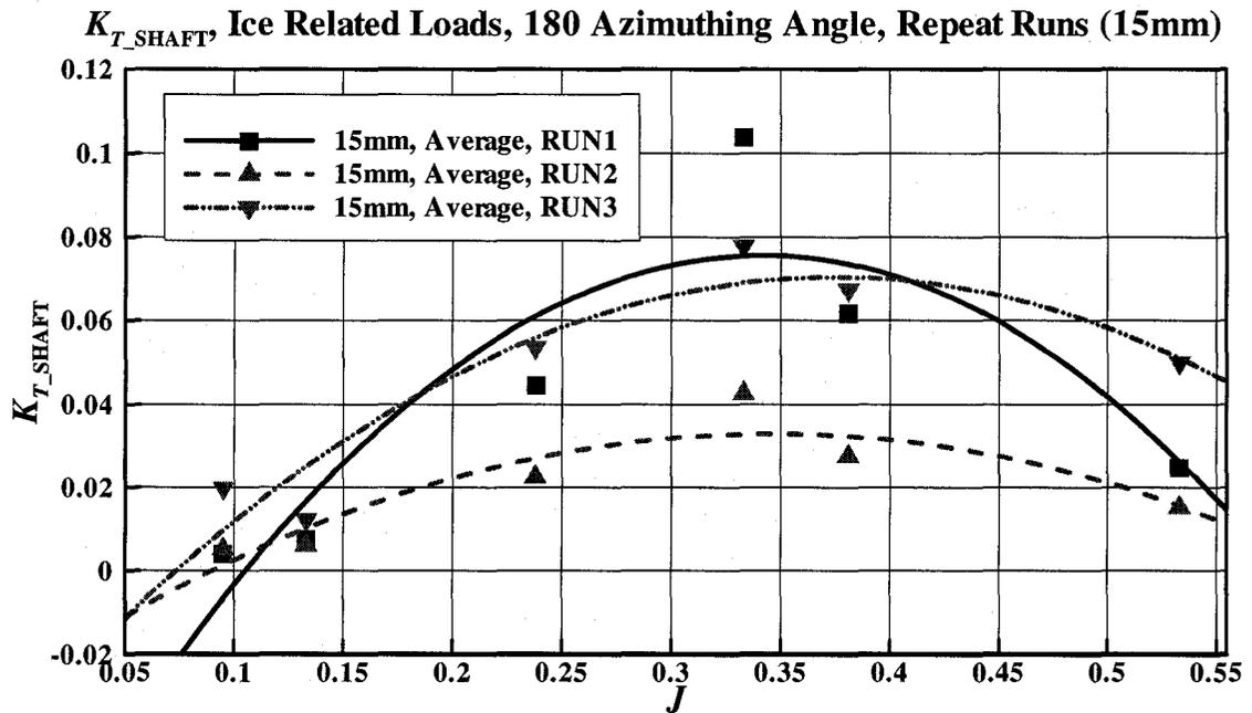
Figure C-22:  $K_{T\_SHAFT}$  vs.  $J$ , average ice related loads at 15mm depth of cut (repeated)
