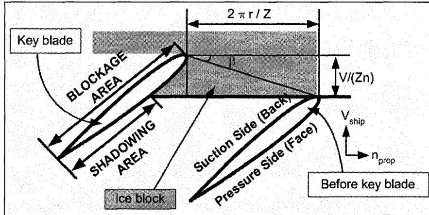
Figure 4-5: Conceptual sketch of the blockage and shadowing area ( $\beta$  is the angle of advance,  $V$  is the carriage speed, and  $Z$  is the number of blade)
