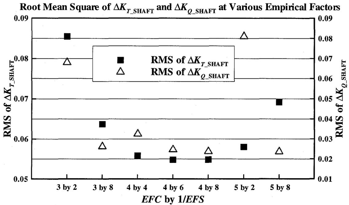
Figure 5-35: RMS of  $\Delta K_{T\_SHAFT}$  and  $\Delta K_{Q\_SHAFT}$  at Various Empirical Factors ( $EFC$  by  $1/EFS$ )
