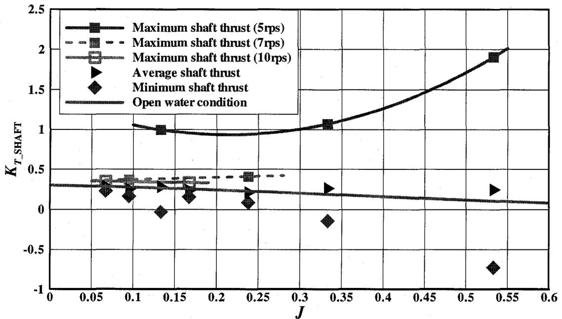
Figure 3-41: Maximum, minimum and average  $K_{T\_SHAFT}$  for the 35mm depth of cut (ice-related loads + separable hydrodynamic loads during milling period) and open water
