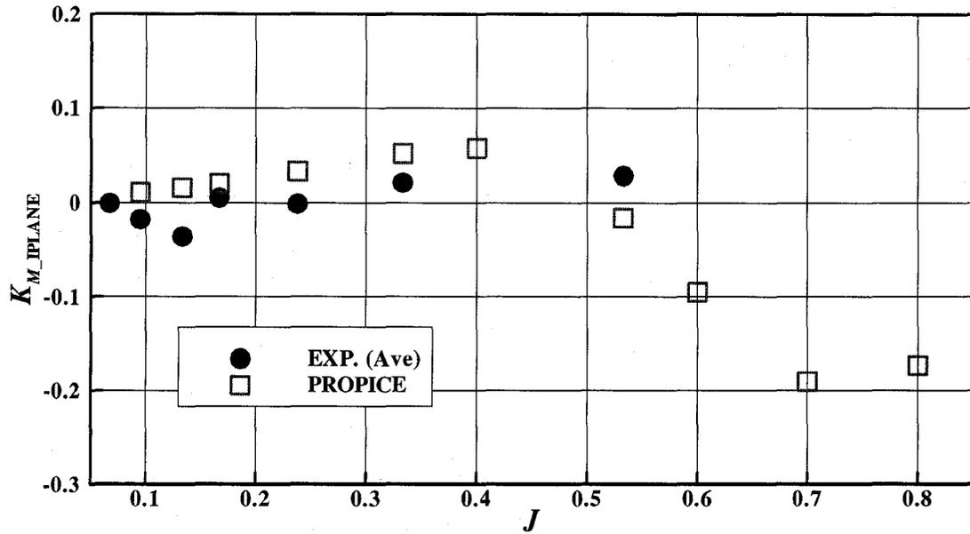
Figure 5-7:  $K_{M\_IPLANE}$  comparison (ice related loads, azimuthing angle of 180 degrees, 35 mm depth of cut, key blade only)
