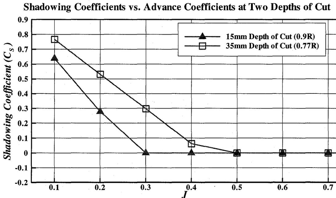
Figure 3-31: Shadowing coefficients vs. advance coefficients at two depths of cut
