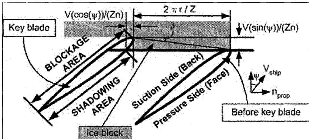
Figure 4-8: Shadowing area at various azimuthing angles
