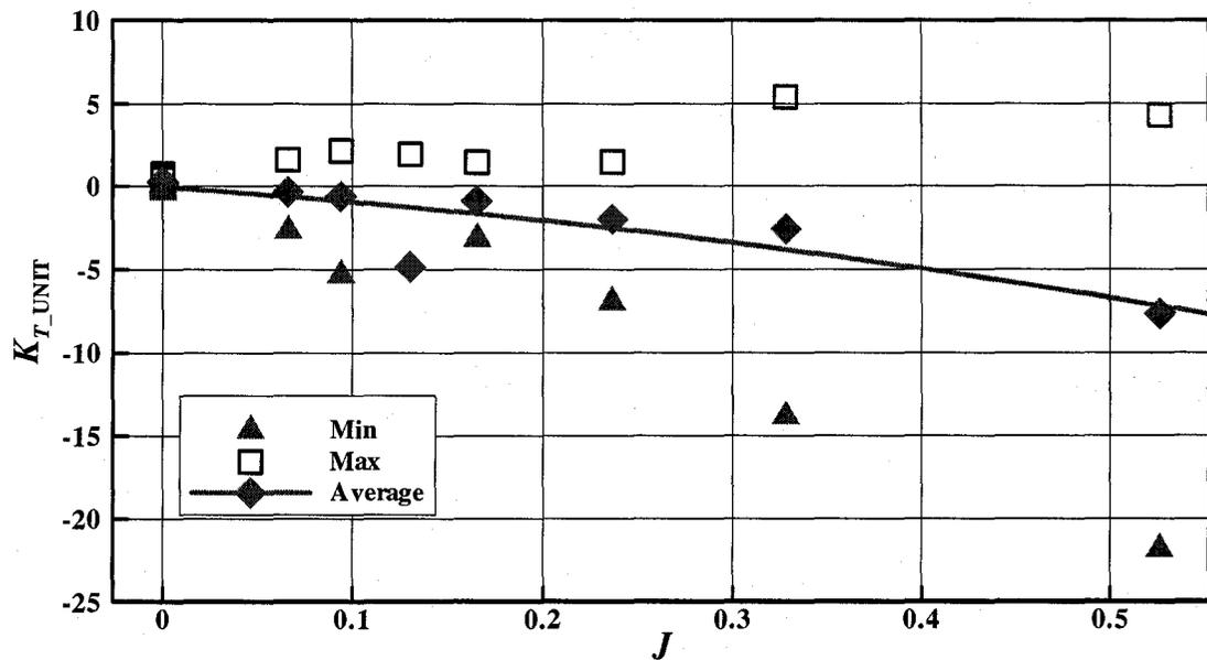
Figure D-1:  $K_{T\_UNIT}$  vs.  $J$ , an azimuthing angle of 180 degrees in ice covered water
