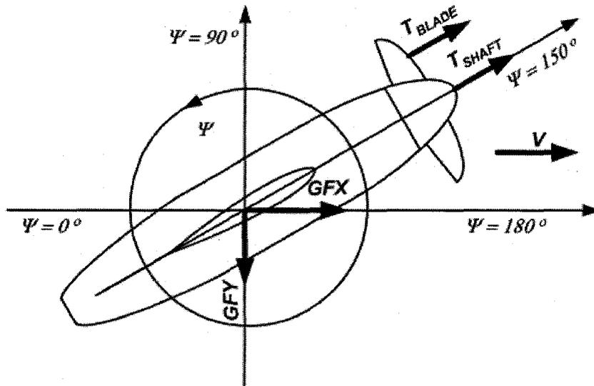
Figure 3-19: Tractor mode with an azimuthing angle of 150 degrees,  $V$  is the carriage speed, top view
