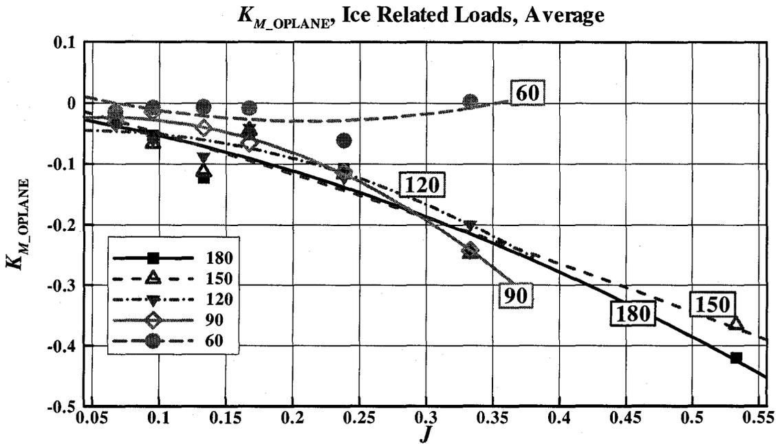
Figure C-13:  $K_{M\_OPLANE}$  vs.  $J$ , average ice related loads at various azimuthing angles (180 ~ 60 degrees)
