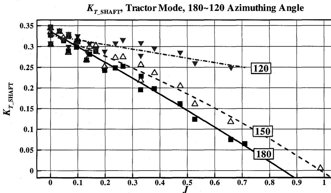
Figure 3-23:  $K_{T\_SHAFT}$  vs.  $J$  at different azimuthing angles (180-120 degrees)
