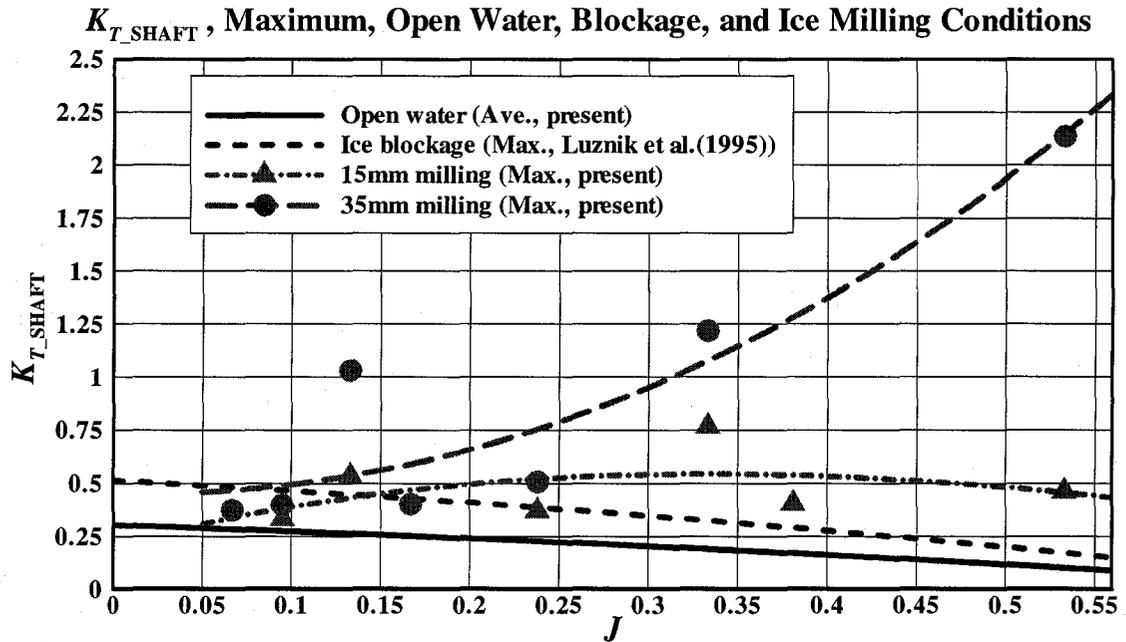
Figure 3-39: Thrust coefficient comparison among open water, ice blockage and ice milling conditions (for 15 and 35 mm depth of cut: ice-related loads + separable hydrodynamic loads during a milling period)
