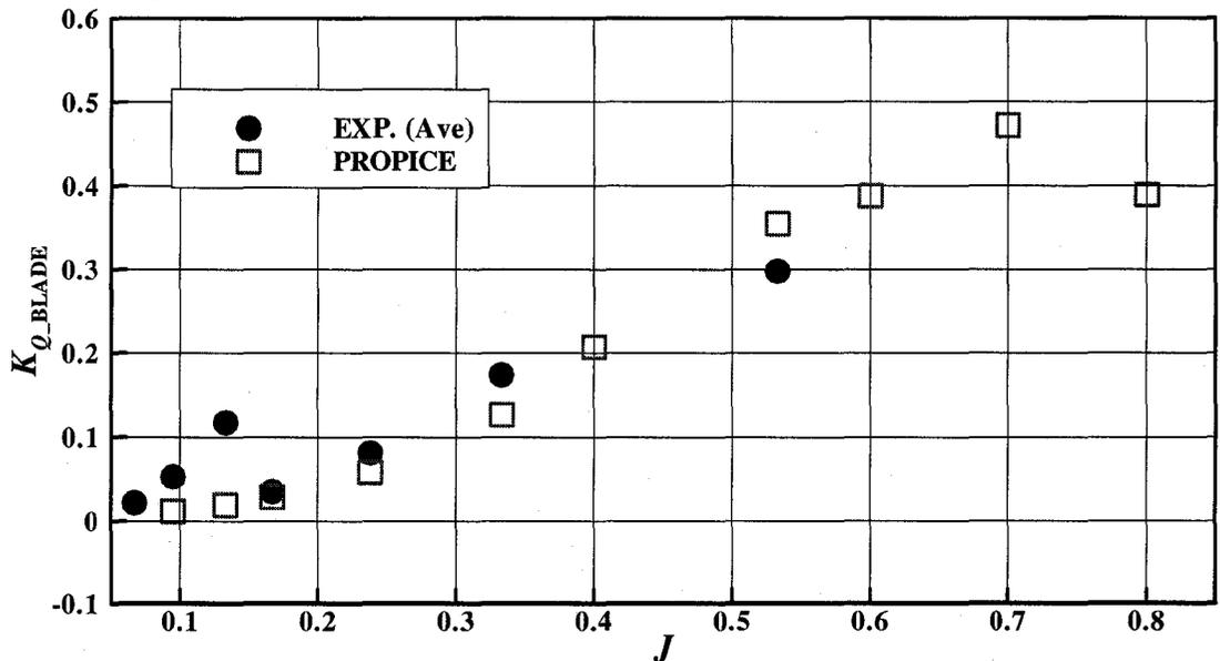
Figure 5-6:  $K_{Q\_BLADE}$  comparison (ice related loads, azimuthing angle of 180 degrees, 35 mm depth of cut, key blade only)
