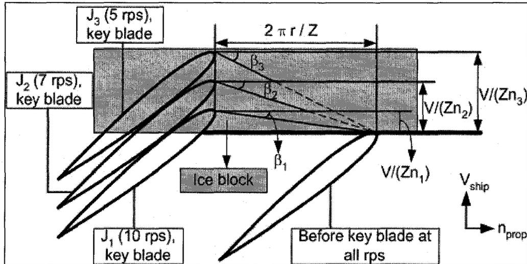
Figure 3-30: Conceptual sketch for propeller-ice interaction with top view, where  $\beta$  is the angle of advance,  $r$  is the radius of the propeller (0.15 m),  $Z$  is number of blades (4),  $V$  is carriage speed,  $n_1$ ,  $n_2$  and  $n_3$  is 10, 7, and 5 rps respectively.
