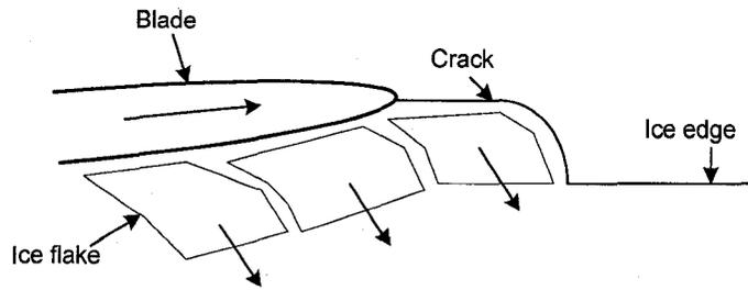
Figure 2-7: Ice flake on face side (after Soininen, 1998)
