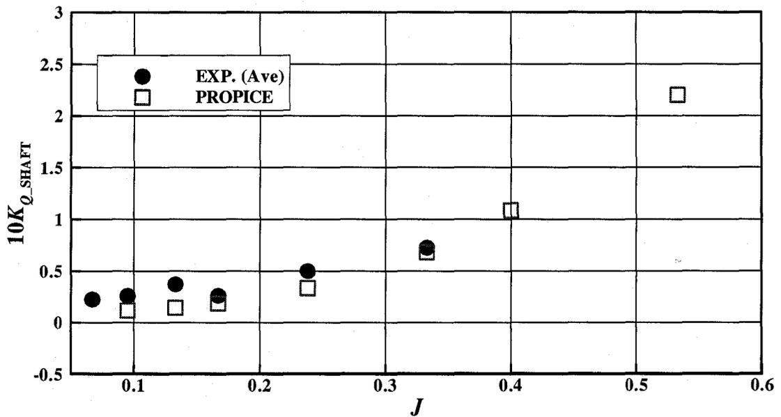
Figure 5-16:  $10K_{Q\_SHAFT}$  comparison (ice related loads, azimuthing angle of 120 degrees, 35 mm depth of cut)
