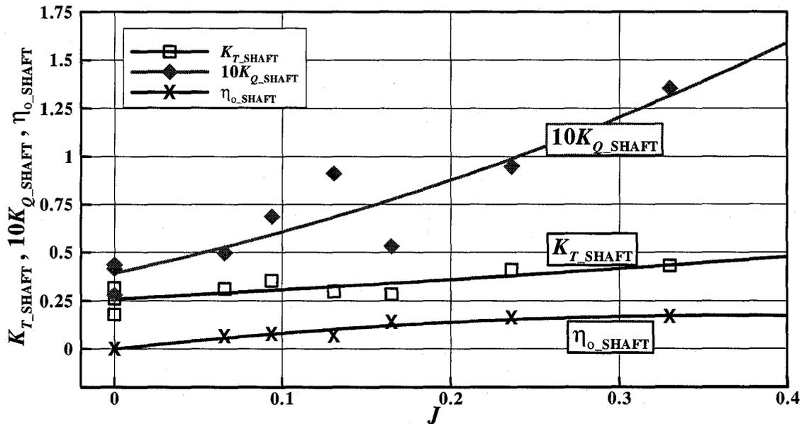
Figure D-17: Ice covered water characteristics for a tractor mode at an azimuthing angle of 120 degrees
