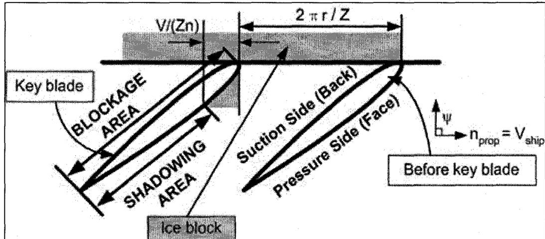
Figure 4-9: Shadowing area at an azimuthing angle of 90 degrees
