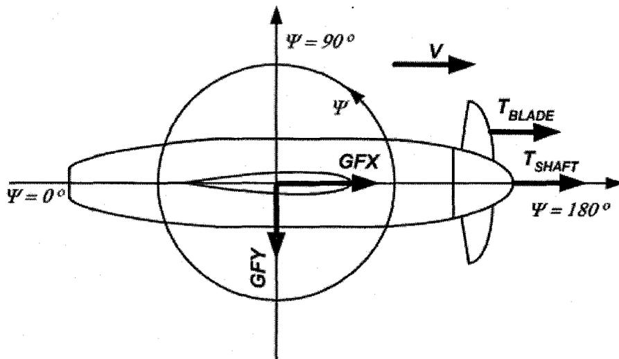
Figure 3-18: Tractor mode with an azimuthing angle of 180 degrees,  $V$  is the carriage speed, top view
