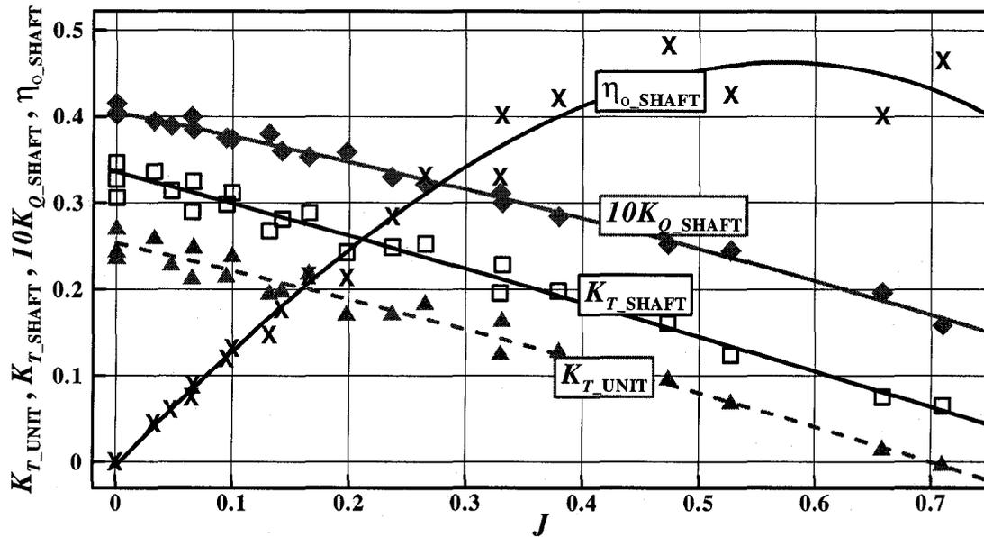
Figure 3-21: Open water characteristics of the model podded propulsor with a tractor mode
