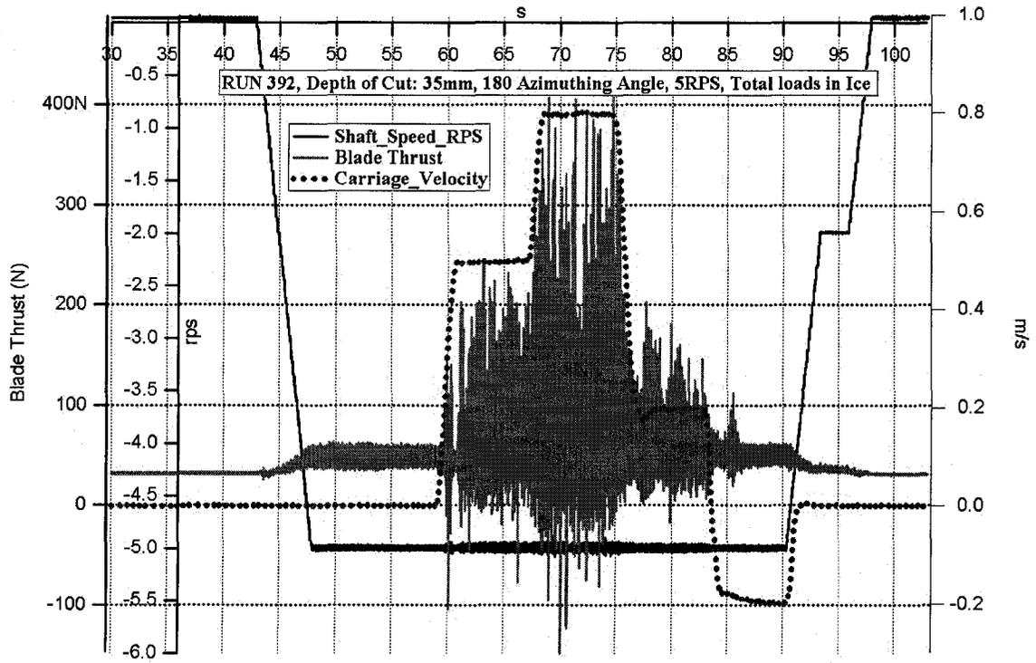
Figure 3-16: Time series data for blade thrust vs. rps & carriage speed
