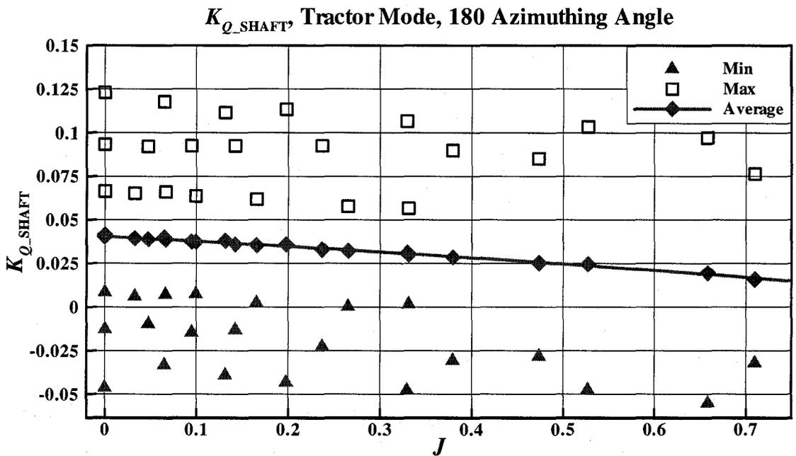
Figure B-5:  $K_{Q\_SHAFT}$  vs.  $J$  at an azimuthing angle of 180 degrees in open water
