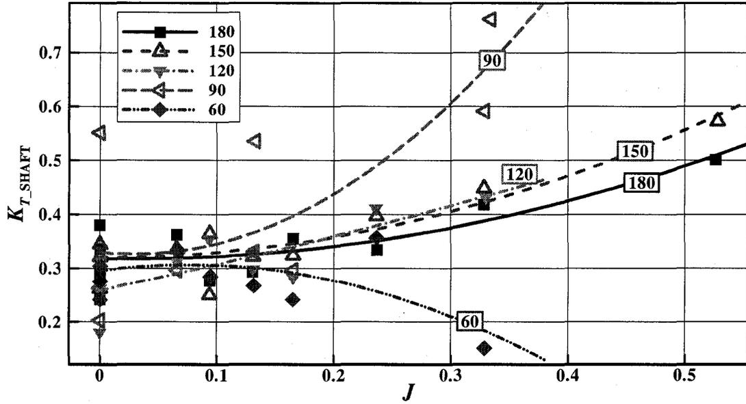
Figure 3-36:  $K_{T\_SHAFT}$ , total loads at various azimuthing angles in ice covered water
