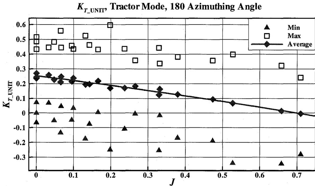
Figure B-1:  $K_{T\_UNIT}$  vs.  $J$  at an azimuthing angle of 180 degrees in open water
