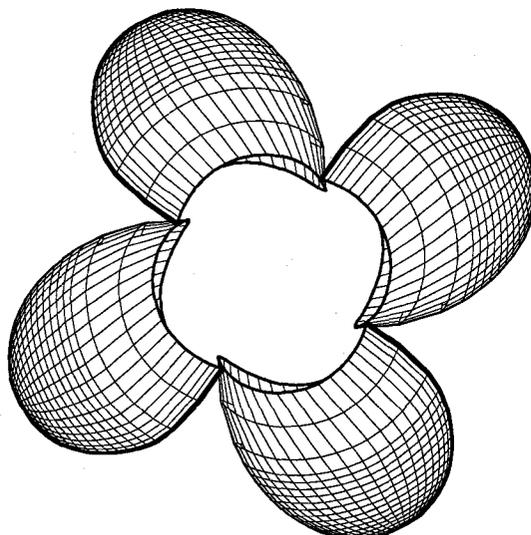
Figure 4-3: Geometry and paneling of the propeller
