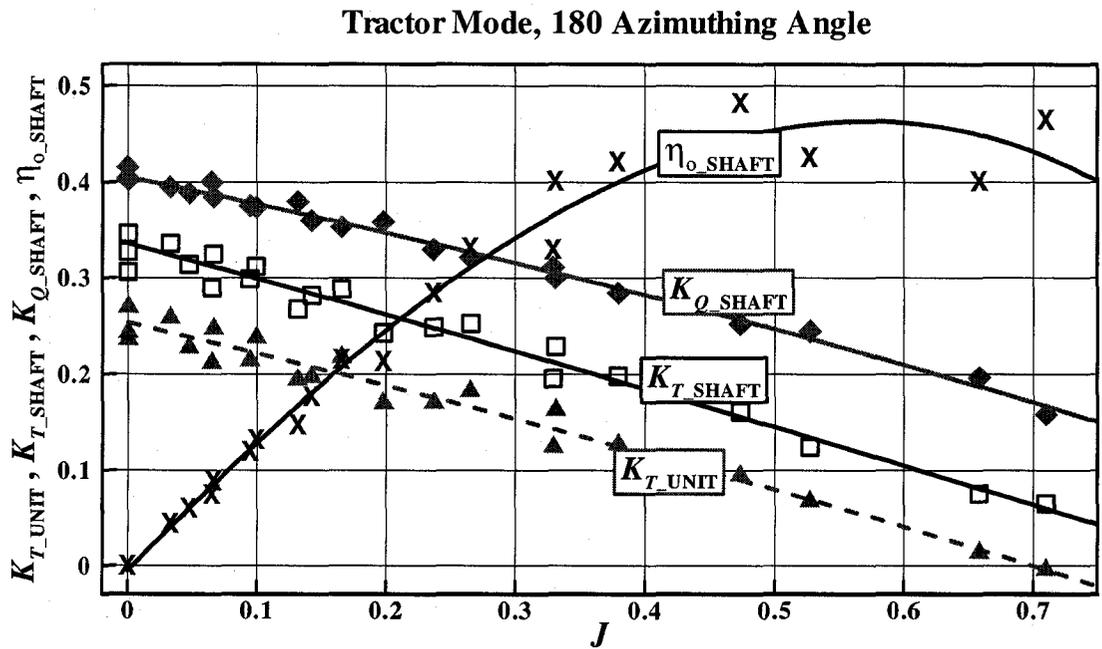
Figure B-21: Open water characteristics for tractor mode at 180° azimuthing angle
