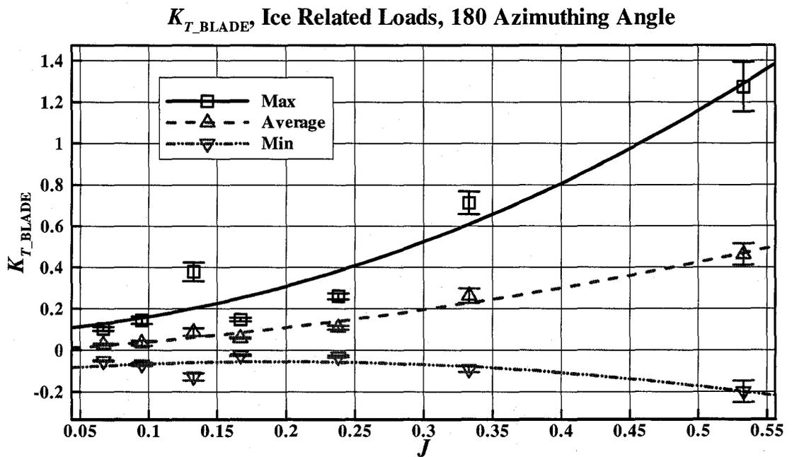
Figure C-3:  $K_{T\_BLADE}$  vs.  $J$ , maximum-average-minimum ice related loads with error bars
