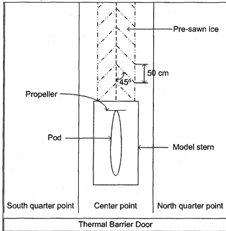
Figure 3-14: Sketch of pre-sawn ice sheet with 180 degrees tractor mode
