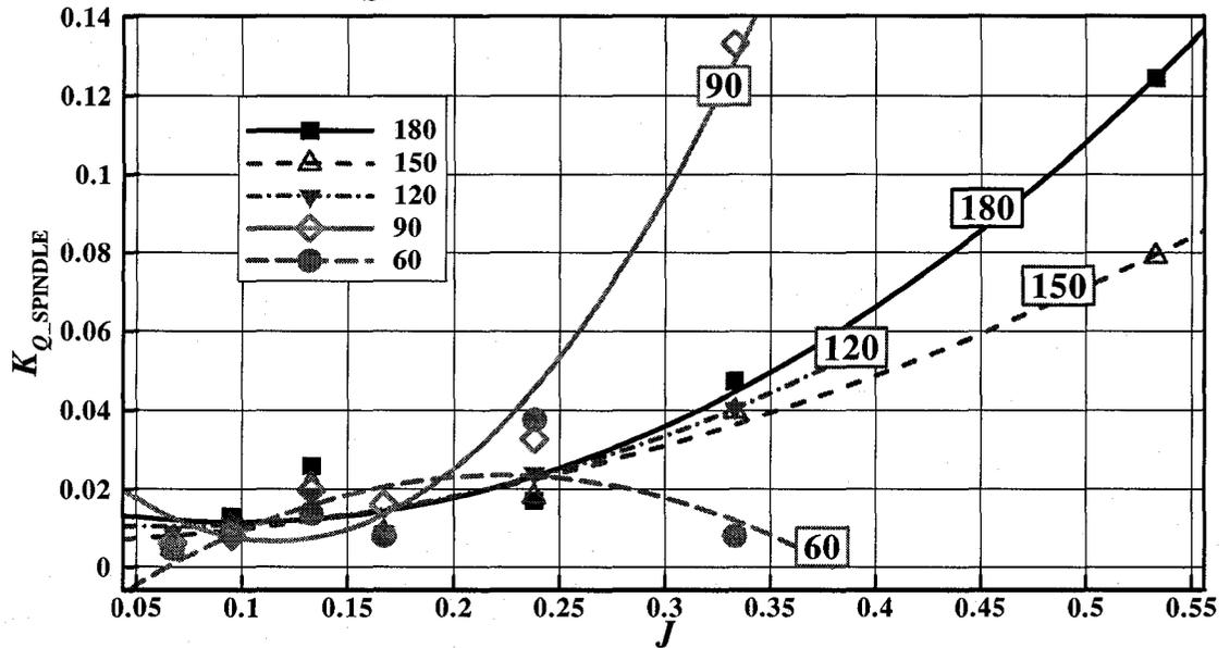
Figure C-21:  $K_{Q\_SPINDLE}$  vs.  $J$ , maximum ice related loads at various azimuthing angles (180 ~ 60 degrees)
