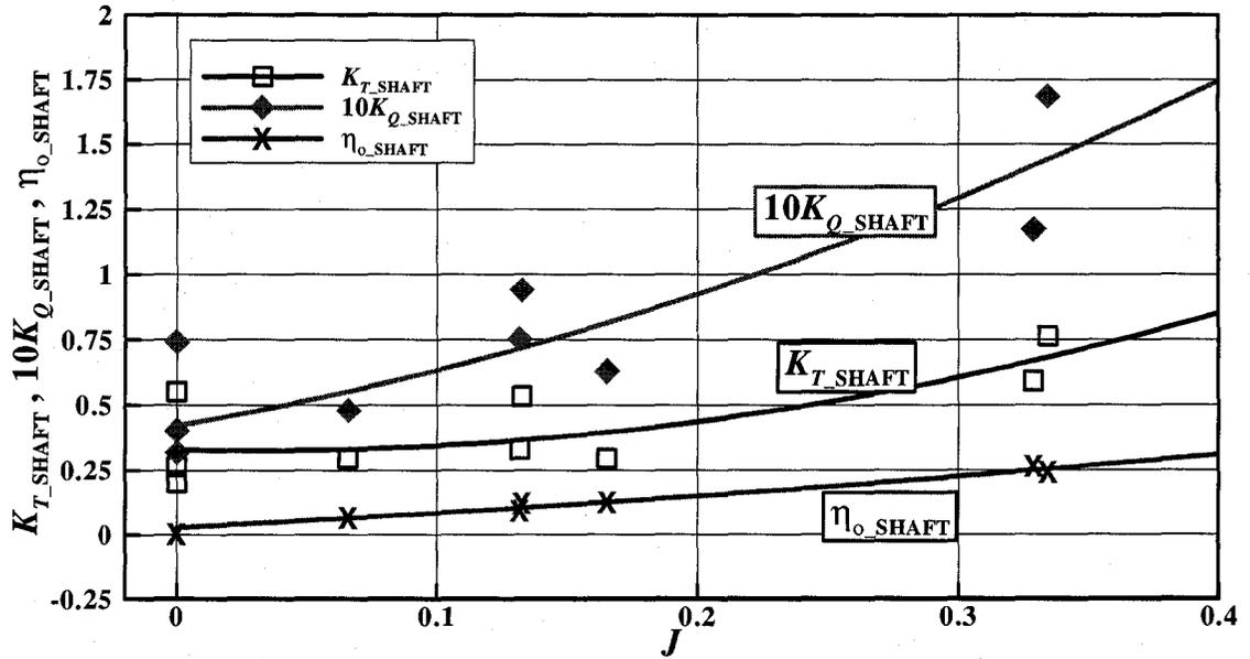
Figure D-18: Ice covered water characteristics for a tractor mode at an azimuthing angle of 90 degrees
