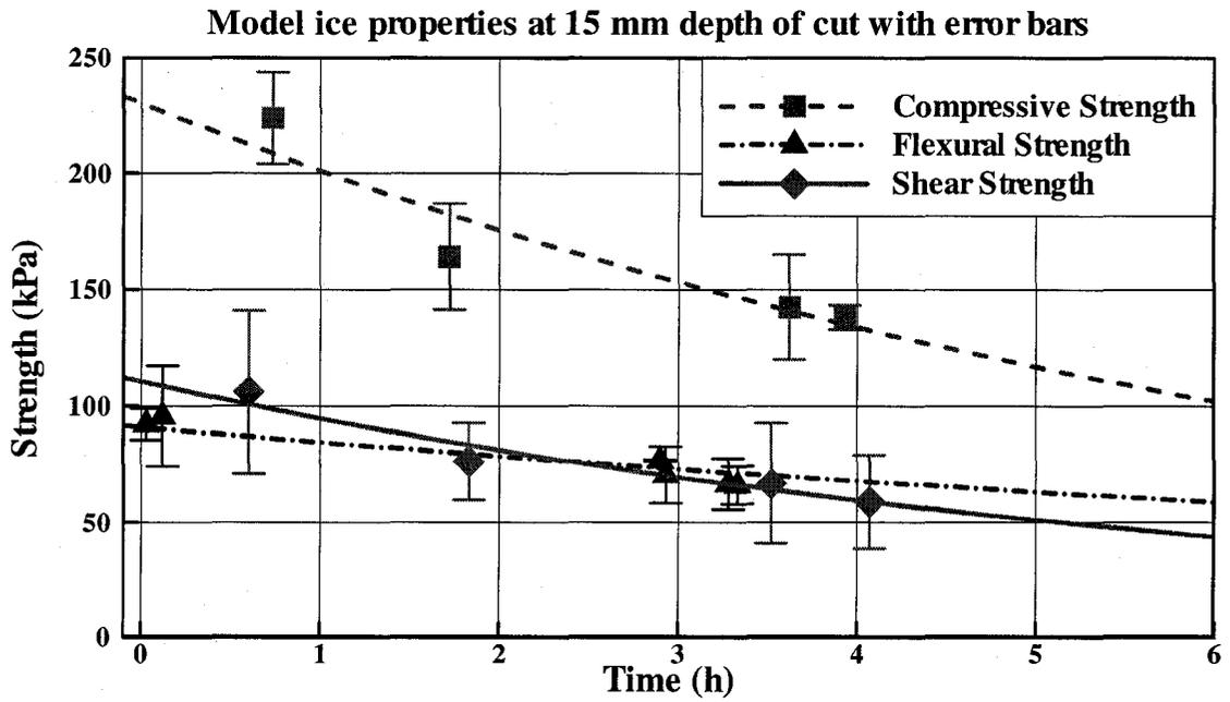
Figure 3-3: Model ice properties at the depth of cut of 15 mm with error bars ( $\pm 2$  times standard deviations)
