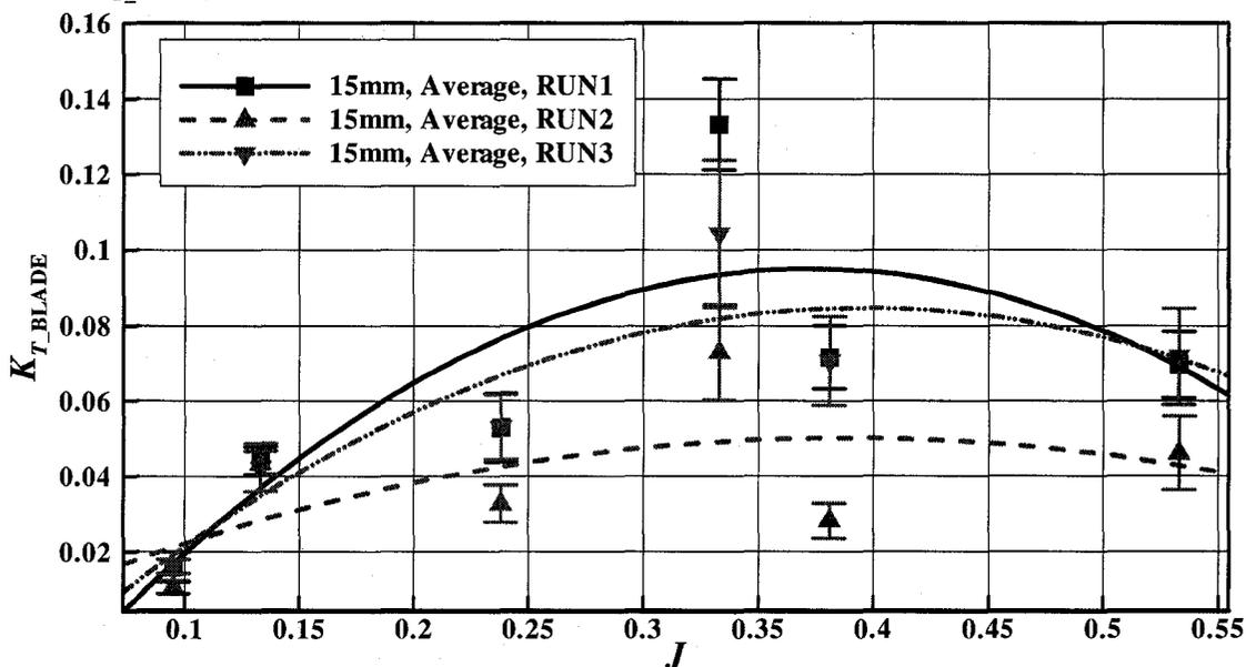
Figure 3-32:  $K_{T\_BLADE}$ , average ice related loads, tractor mode, repeat runs (15mm)
