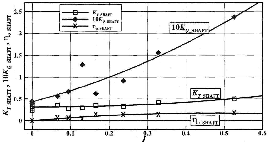
Figure D-15: Ice covered water characteristics for a tractor mode at an azimuthing angle of 180 degrees
