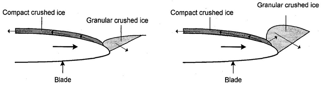
Figure 2-9: Crushed ice (after Soininen, 1998)
