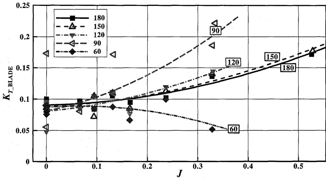
Figure D-13:  $K_{T\_BLADE}$  vs.  $J$  at an azimuthing angle of 180 ~ 60 degrees in ice covered water
