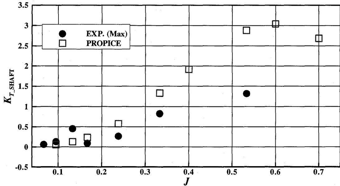
Figure E-2: Maximum  $K_{T\_SHAFT}$  comparison (ice related loads, azimuthing angle of 150 degrees, 35 mm depth of cut)
