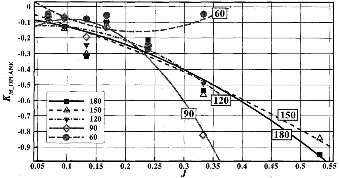
Figure C-20:  $K_{M\_OPLANE}$  vs.  $J$ , negative maximum ice related loads at various azimuthing angles (180 ~ 60 degrees)
