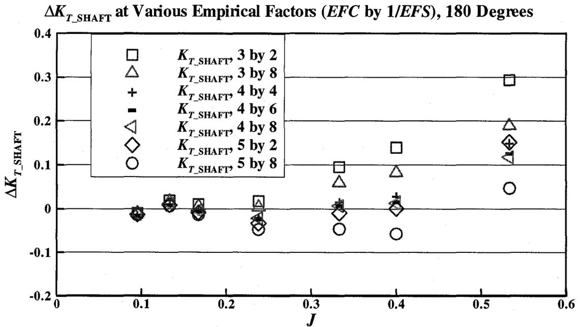
Figure 5-25:  $\Delta K_{T\_SHAFT}$  at various empirical factors ( $EFC$  by  $1/EFS$ ) with 180 degrees and 35 mm depth of cut
