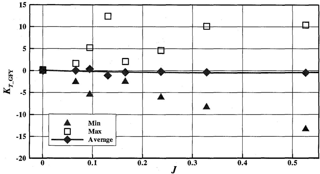
Figure D-2:  $K_{T\_GFY}$  vs.  $J$  at an azimuthing angle of 180 degrees in ice covered water
