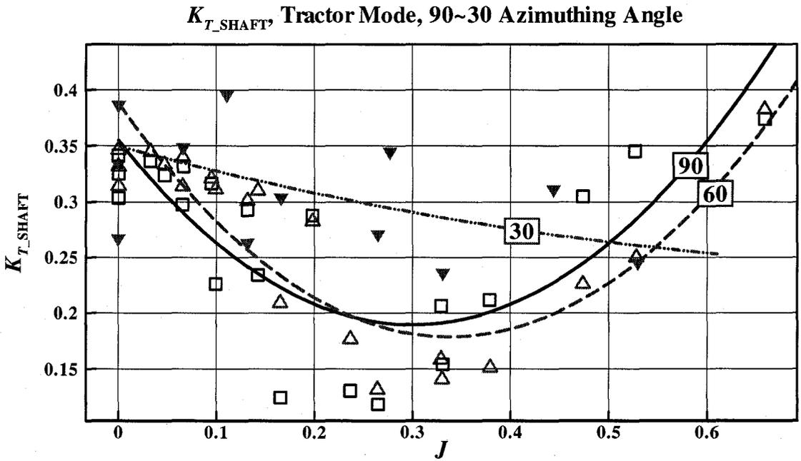
Figure B-14:  $K_{T\_SHAFT}$  vs.  $J$  at various azimuthing angles (90–30 degrees) in open water
