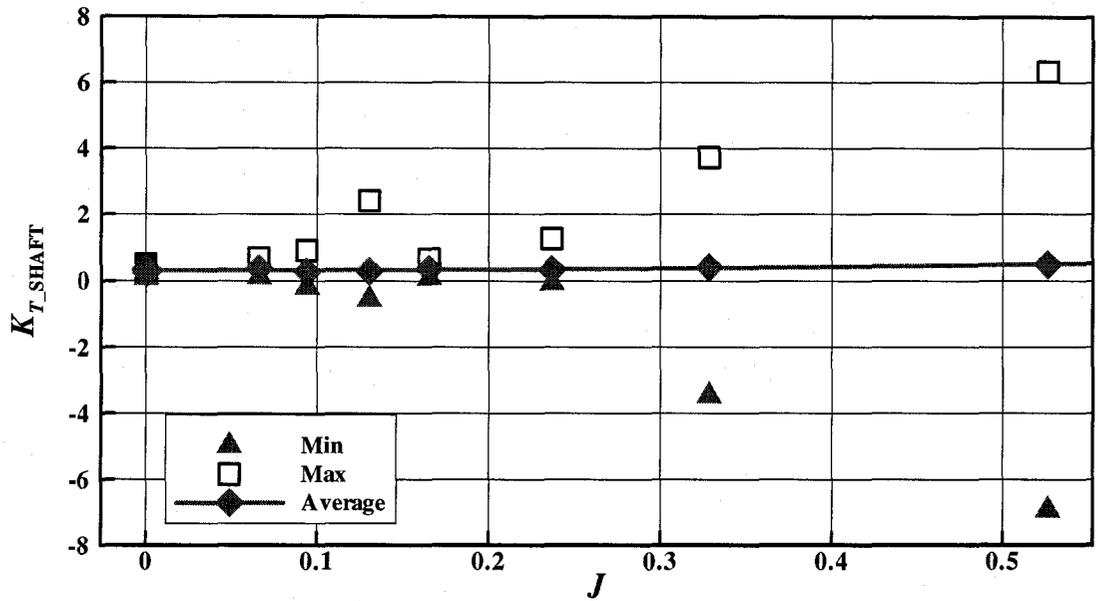
Figure D-4:  $K_{T\_SHAFT}$  vs.  $J$  at an azimuthing angle of 180 degrees in ice covered water
