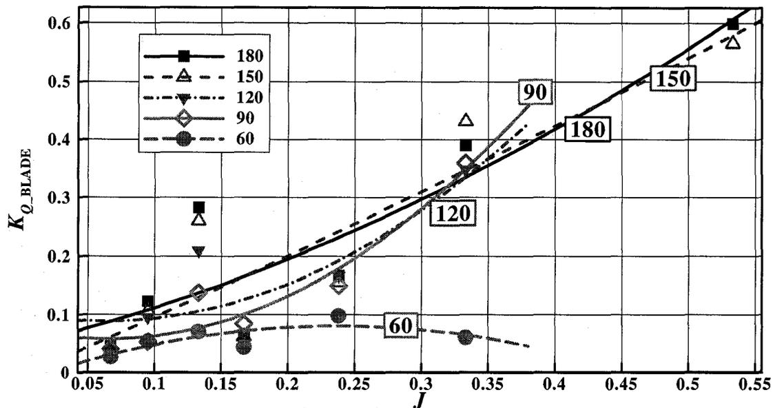
Figure C-18:  $K_{Q\_BLADE}$  vs.  $J$ , maximum ice related loads at various azimuthing angles (180 ~ 60 degrees)
