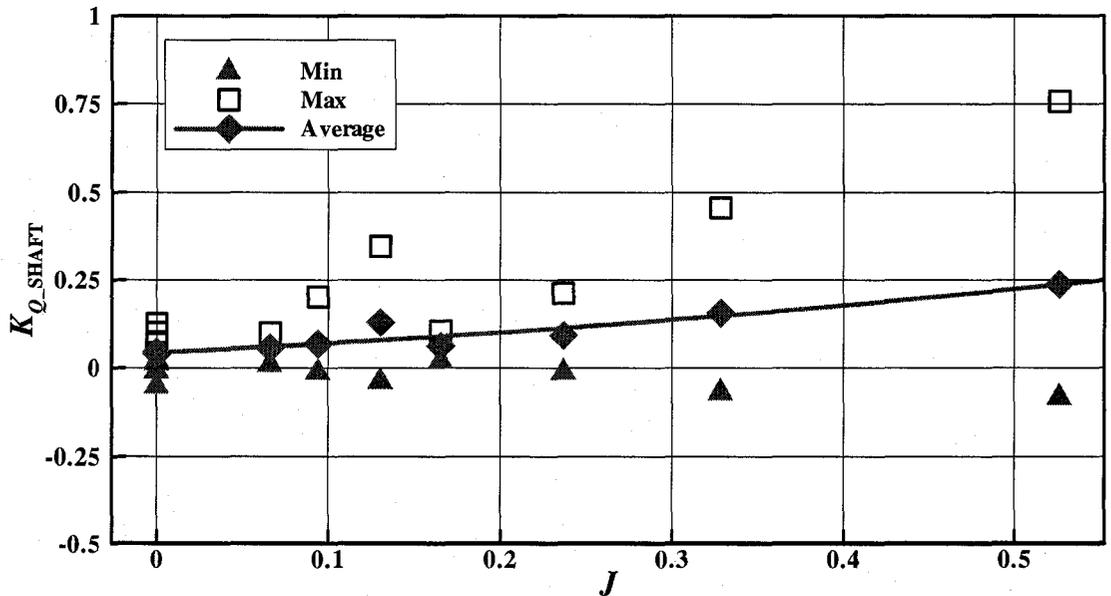
Figure D-5:  $K_{Q\_SHAFT}$  vs.  $J$  at an azimuthing angle of 180 degrees in ice covered water
