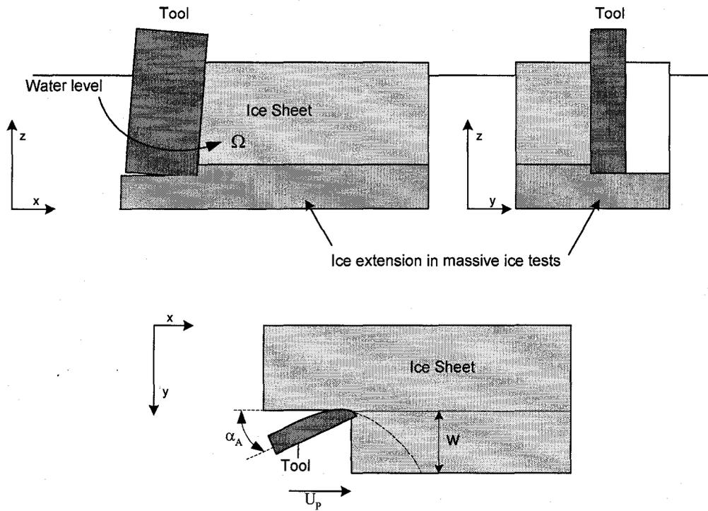
Figure 2-6: Test concept (after Soininen, 1998)
