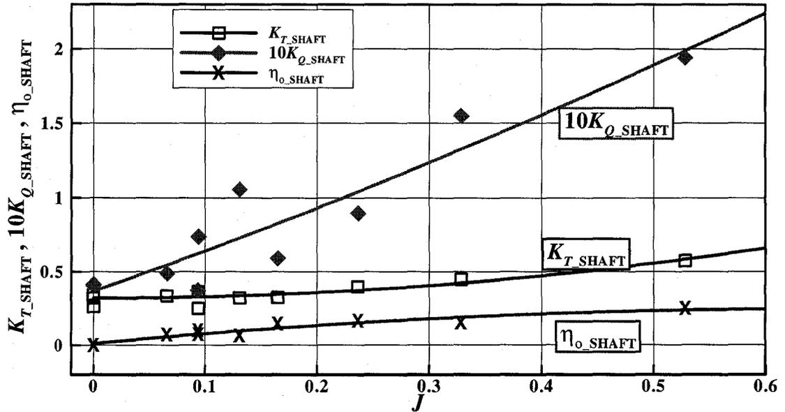
Figure D-16: Ice covered water characteristics for a tractor mode at an azimuthing angle of 150 degrees
