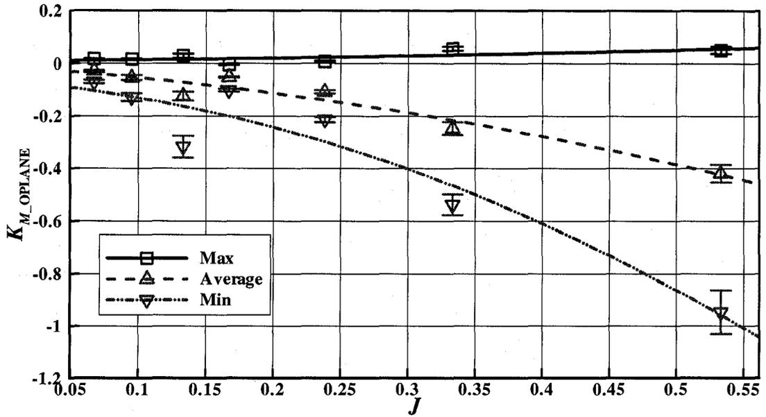
Figure C-6 :  $K_{M\_OPLANE}$  vs.  $J$ , maximum-average-minimum ice related loads with error bars
