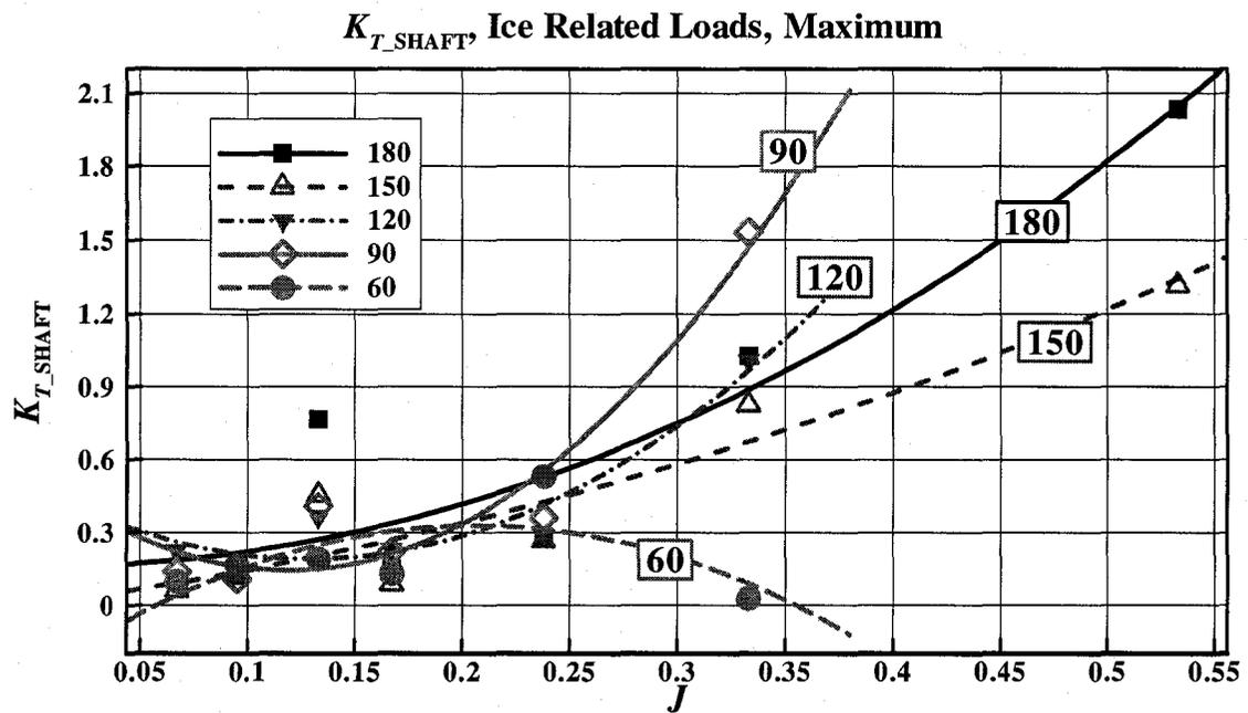
Figure C-15:  $K_{T\_SHAFT}$  vs.  $J$ , maximum ice related loads at various azimuthing angles (180 ~ 60 degrees)
