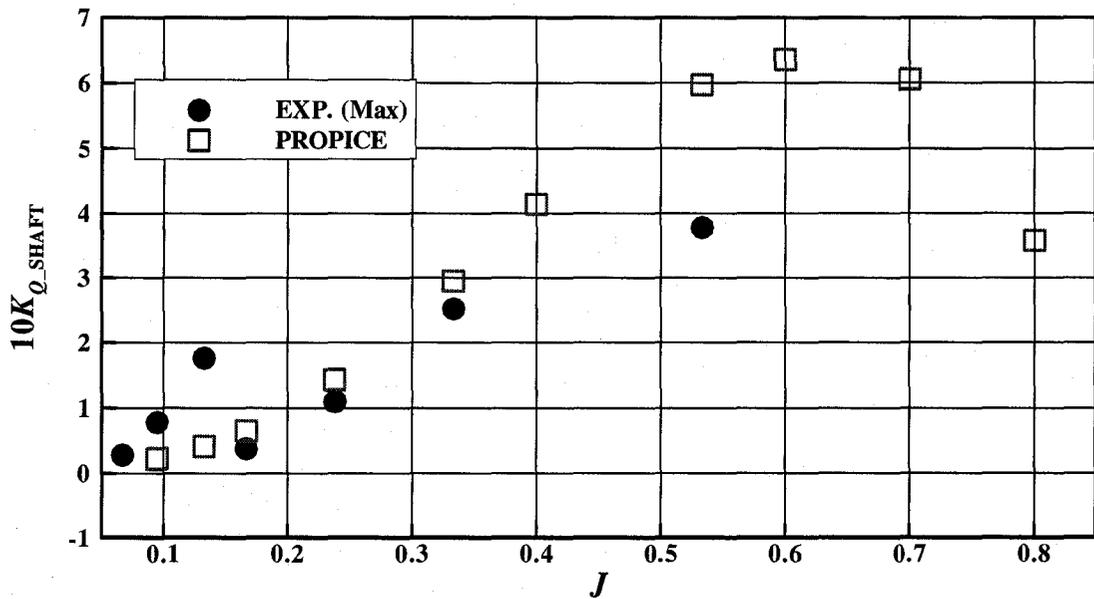
Figure E-5: Maximum  $10K_{Q\_SHAFT}$  comparison (ice related loads, azimuthing angle of 180 degrees, 35 mm depth of cut)
