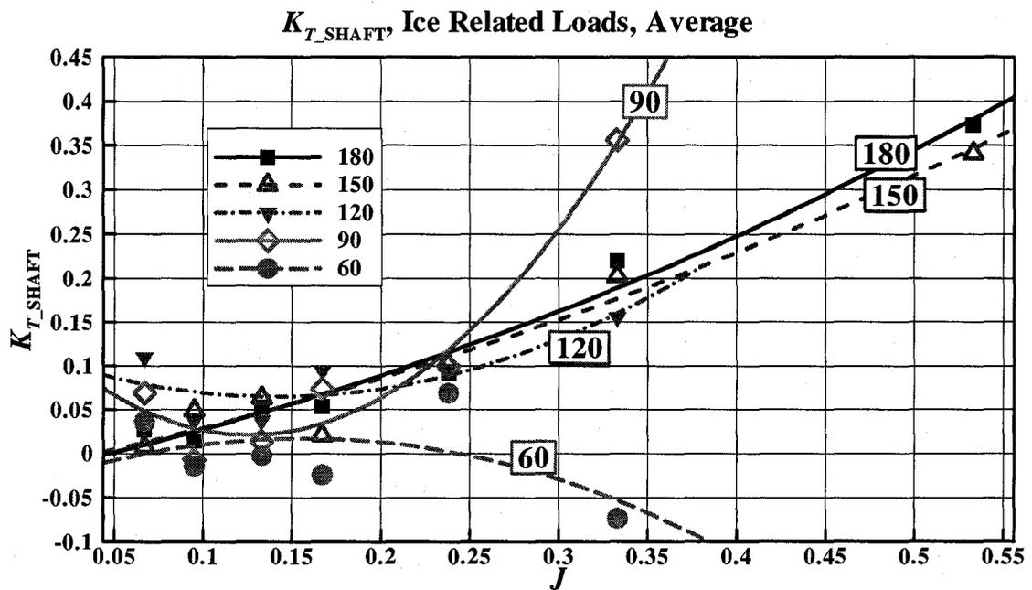
Figure C-8:  $K_{T\_SHAFT}$  vs.  $J$ , average ice related loads at various azimuthing angles (180 ~ 60 degrees)
