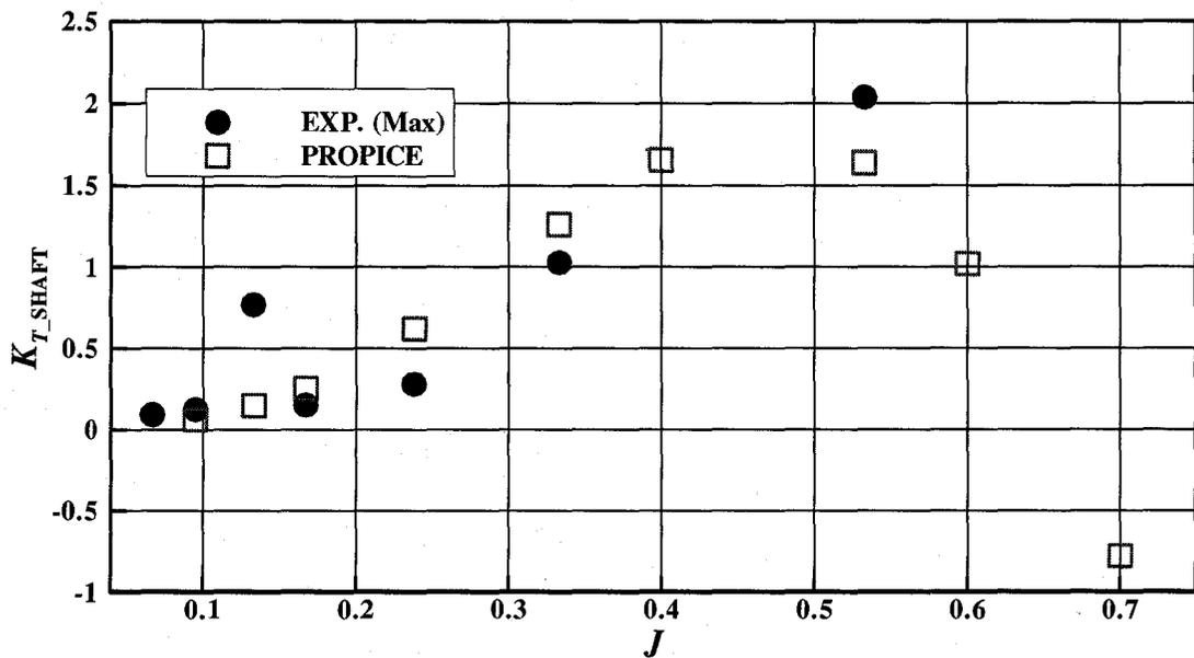
Figure E-1: Maximum  $K_{T\_SHAFT}$  comparison (ice related loads, azimuthing angle of 180 degrees, 35 mm depth of cut)
