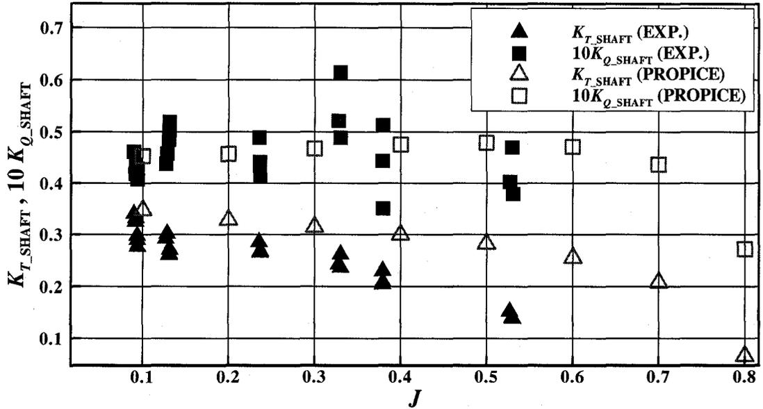
Figure 5-20:  $K_{T\_SHAFT}$  and  $10K_{Q\_SHAFT}$  comparison (Total loads, azimuthing angle of 180 degrees, 15 mm depth of cut)
