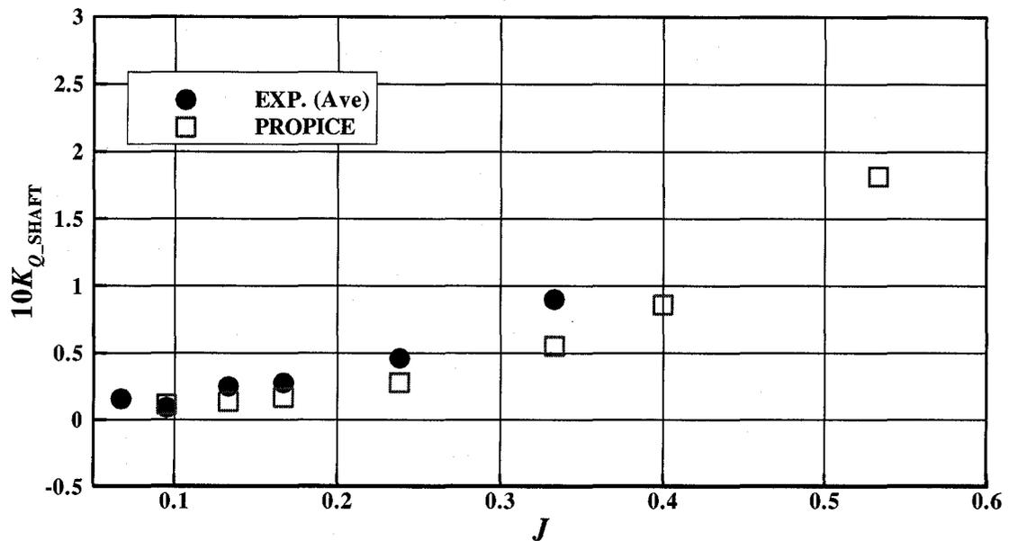
Figure 5-17:  $10K_{Q\_SHAFT}$  comparison (ice related loads, azimuthing angle of 90 degrees, 35 mm depth of cut)
