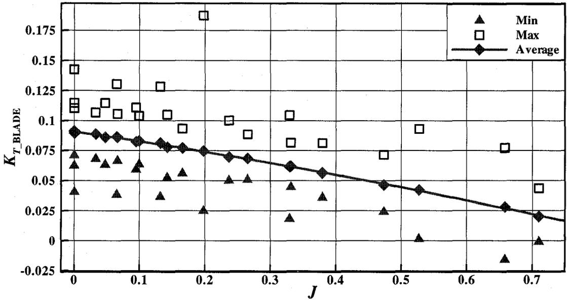
Figure B-6:  $K_{T\_BLADE}$  vs.  $J$  at an azimuthing angle of 180 degrees in open water
