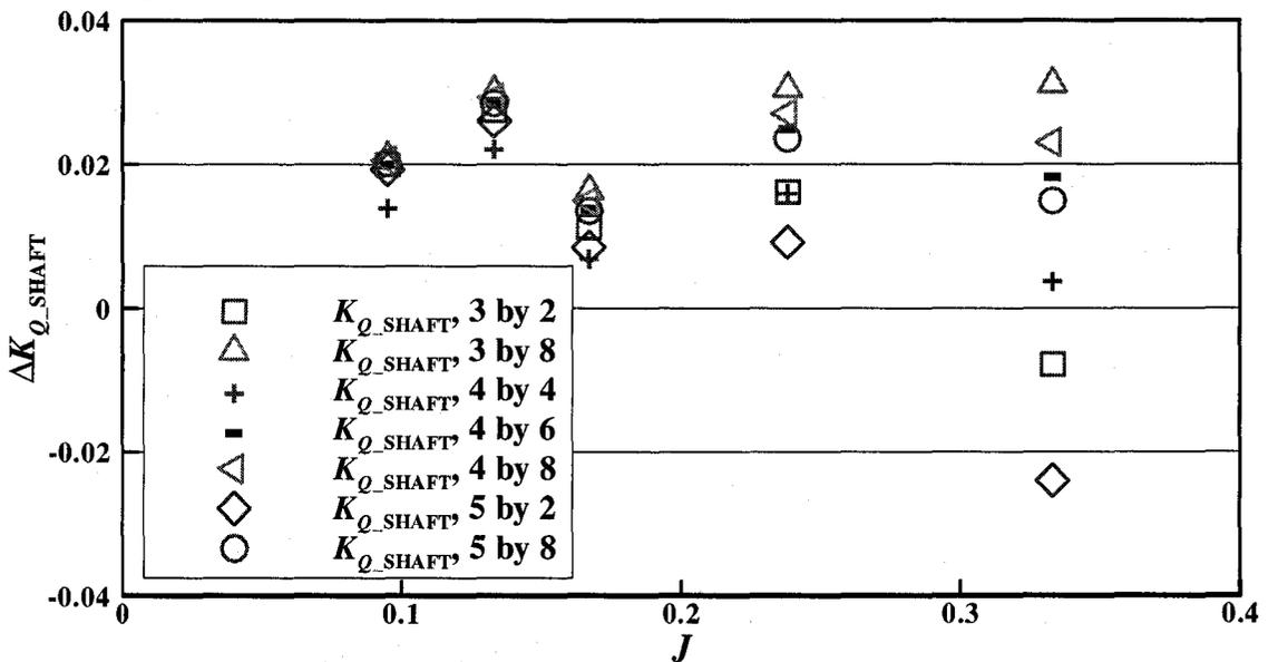
Figure 5-32:  $\Delta K_{Q\_SHAFT}$  at various empirical factors ( $EFC$  by  $1/EFS$ ) with 120 degrees and 35 mm depth of cut
