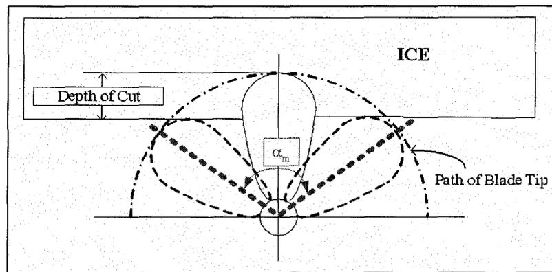
Figure 3-15: Depth of cut and milling angle
