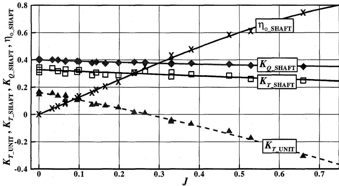
Figure B-23: Open water characteristics for tractor mode at 120° azimuthing angle
