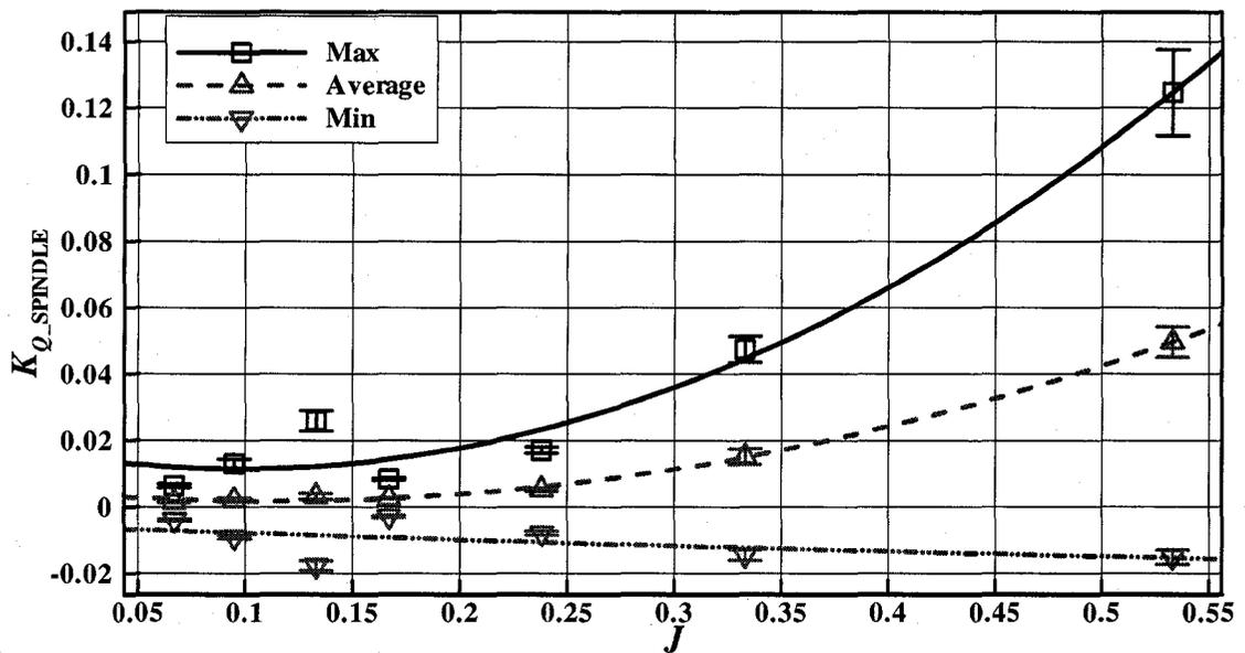
Figure C-7:  $K_{Q\_SPINDLE}$  vs.  $J$ , maximum-average-minimum ice related loads with error bars
