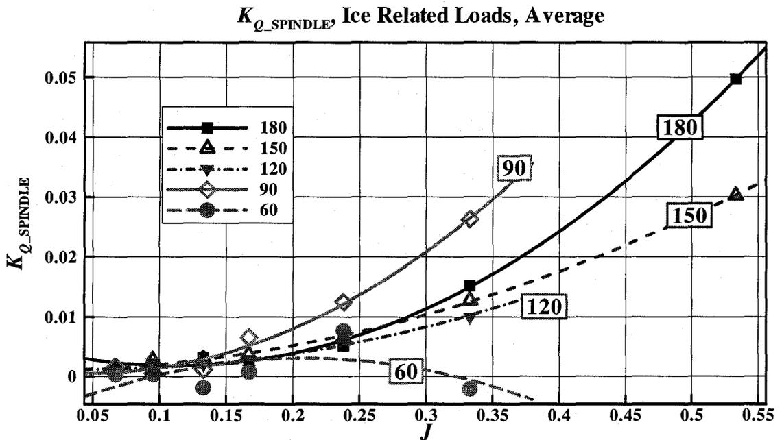
Figure C-14:  $K_{Q\_SPINDLE}$  vs.  $J$ , average ice related loads at various azimuthing angles (180 ~ 60 degrees)
