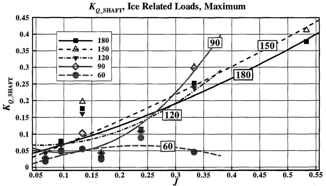
Figure C-16:  $K_{Q\_SHAFT}$  vs.  $J$ , maximum ice related loads at various azimuthing angles (180 ~ 60 degrees)
