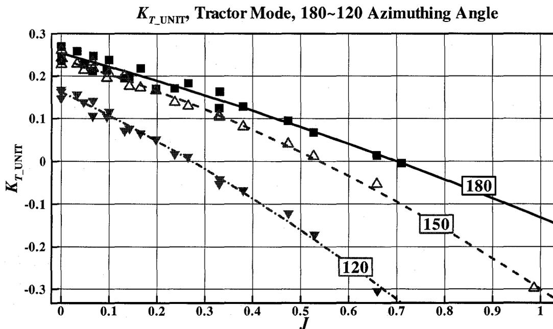
Figure 3-22:  $K_{T\_UNIT}$  vs.  $J$  at different azimuthing angles (180-120 degrees)
