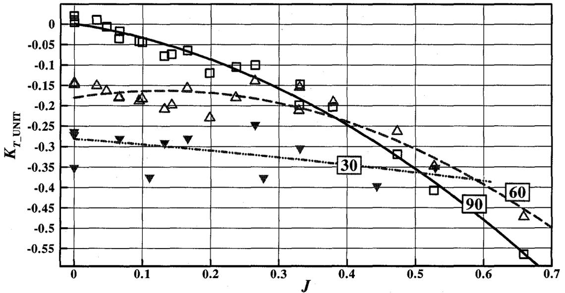
Figure B-9:  $K_{T\_UNIT}$  vs.  $J$  at various azimuthing angles (90–30 degrees) in open water
