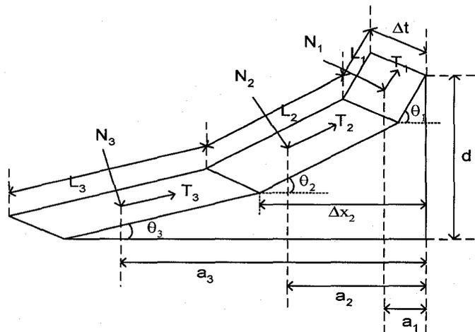
Figure 2-4: Acting stress calculation (after Kotras et al., 1985)
