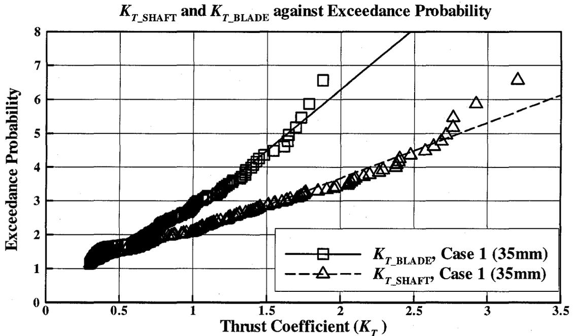
Figure 3-47: Comparison between shaft thrust and blade thrust coefficients with exceedance probability in “Case 1”
