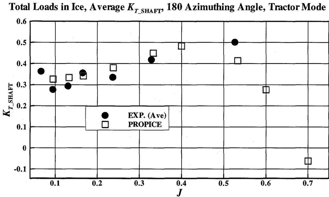
Figure 5-18:  $K_{T\_SHAFT}$  comparison (Total loads, azimuthing angle of 180 degrees, 35 mm depth of cut)
