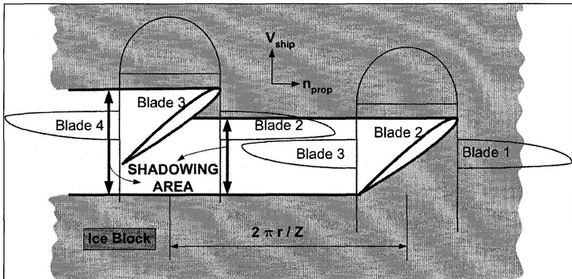
Figure 3-29: Shadowing area ( $Z$  is the number of the blades)
