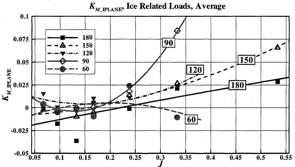
Figure C-12:  $K_{M\_IPLANE}$  vs.  $J$ , average ice related loads at various azimuthing angles (180 ~ 60 degrees)
