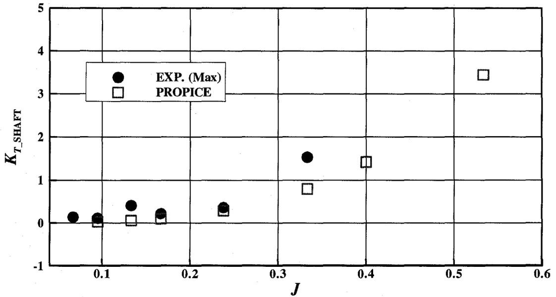
Figure E-4: Maximum  $K_{T\_SHAFT}$  comparison (ice related loads, azimuthing angle of 120 degrees, 35 mm depth of cut)
