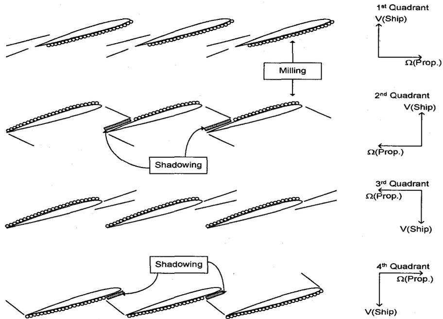
Figure 2-2: Four quadrants operating condition and blade shadowing phenomena (after Kotras et al., 1985)
