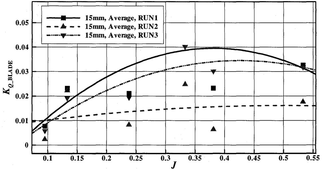
Figure C-25:  $K_{Q\_BLADE}$  vs.  $J$ , average ice related loads at 15mm depth of cut (repeated)
