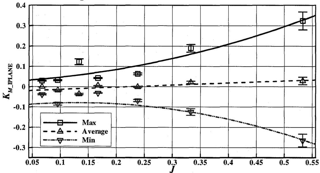
Figure C-5:  $K_{M\_IPLANE}$  vs.  $J$ , maximum-average-minimum ice related loads with error bars
