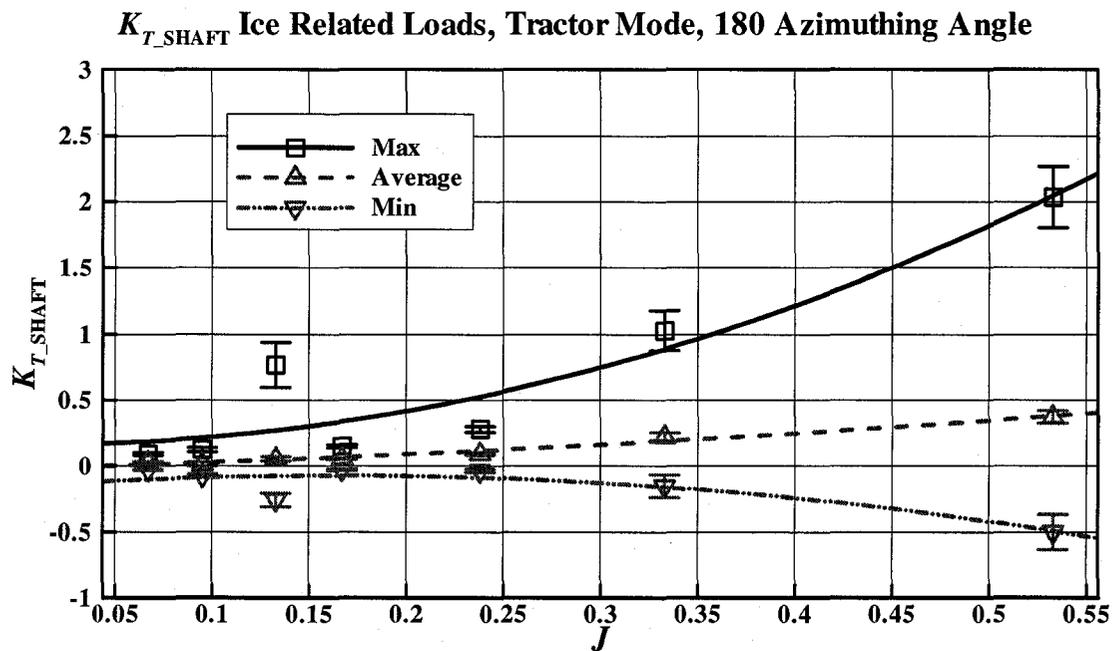
Figure 3-25:  $K_{T\_SHAFT}$ , ice related loads at azimuthing angle of 180 degrees (tractor mode)
