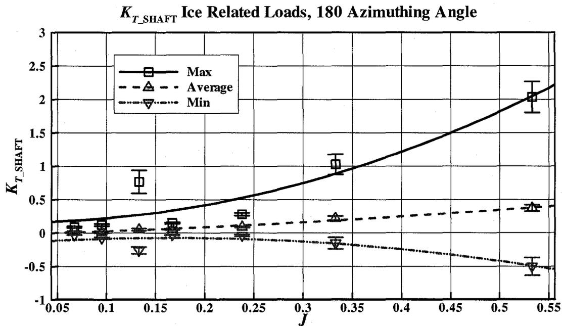
Figure C-1:  $K_{T\_SHAFT}$  vs.  $J$ , maximum-average-minimum ice related loads with error bars
