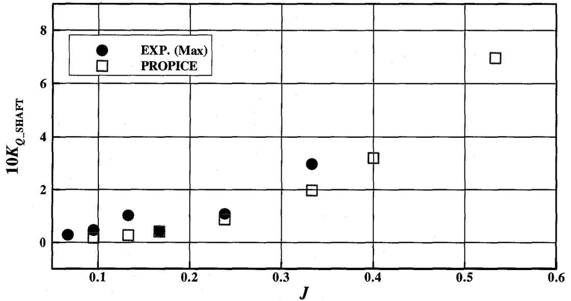
Figure E-8: Maximum  $10K_{Q\_SHAFT}$  comparison (ice related loads, azimuthing angle of 120 degrees, 35 mm depth of cut)
