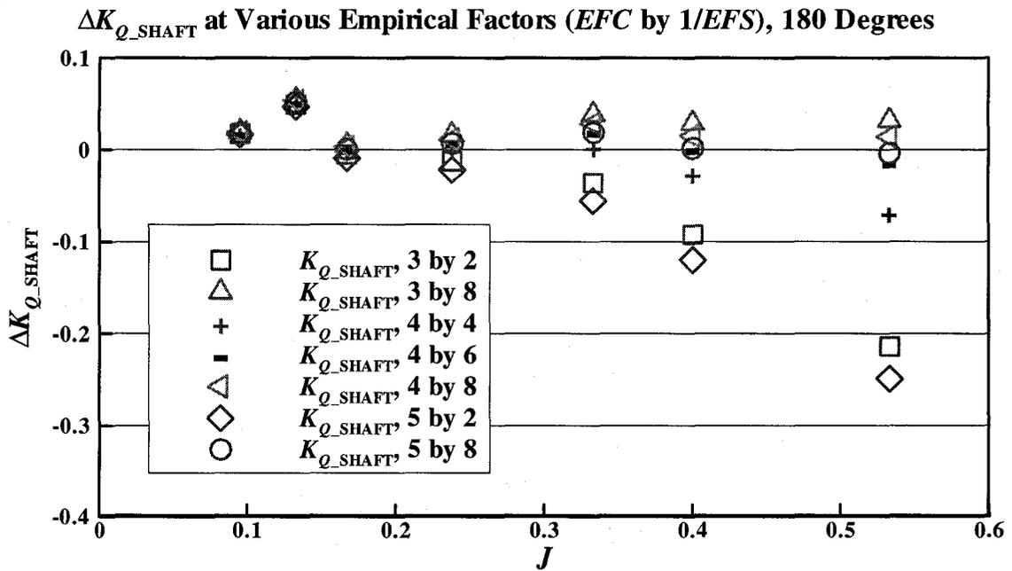
Figure 5-30:  $\Delta K_{Q\_SHAFT}$  at various empirical factors ( $EFC$  by  $1/EFS$ ) with 180 degrees and 35 mm depth of cut
