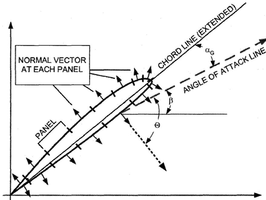
Figure 4-7: Geometrical consideration for the ice contact area ( $\Theta$  : the interacting angle)
