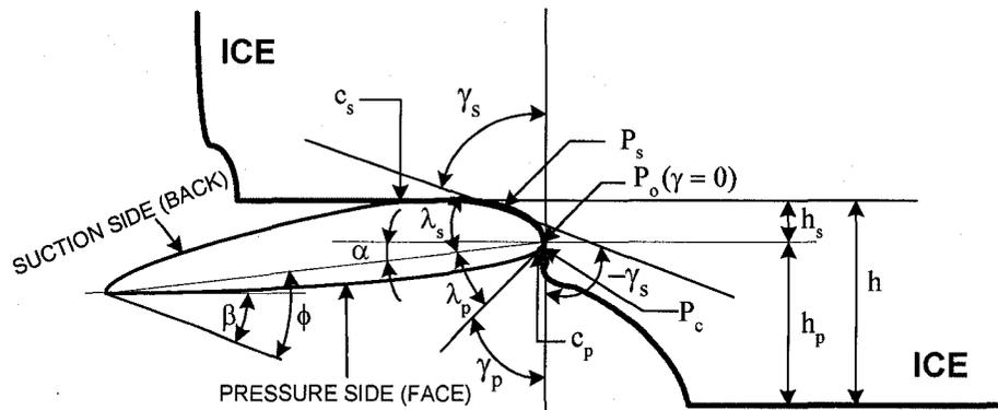
Figure 2-5: Cutting geometry (after Veitch, 1995)
