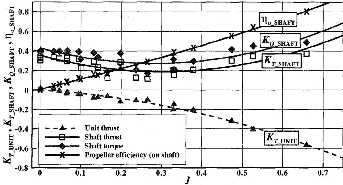
Figure B-24: Open water characteristics for tractor mode at 90° azimuthing angle
