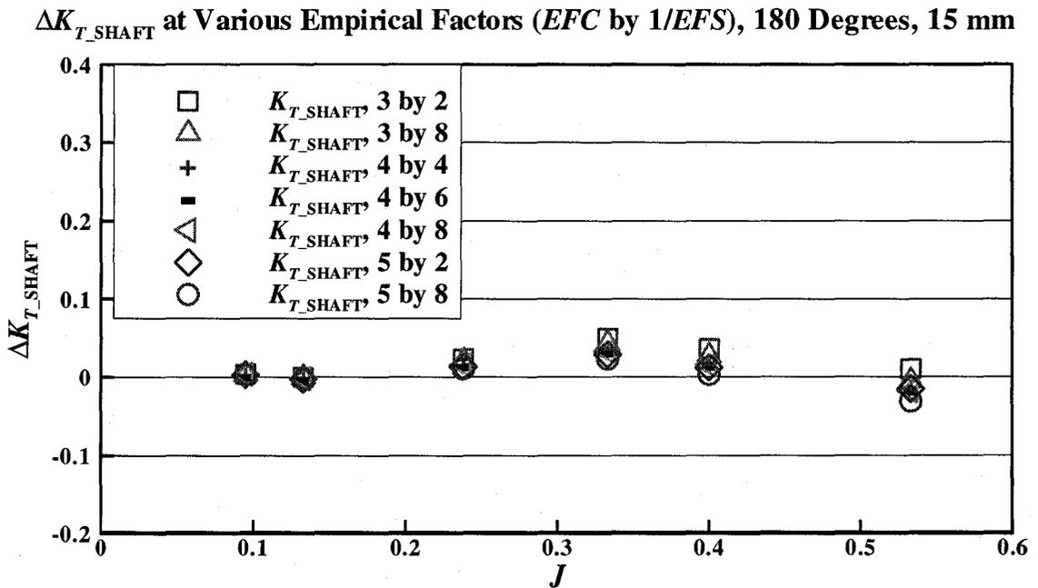
Figure 5-29:  $\Delta K_{T\_SHAFT}$  at various empirical factors ( $EFC$  by  $1/EFS$ ) with 180 degrees and 15 mm depth of cut
