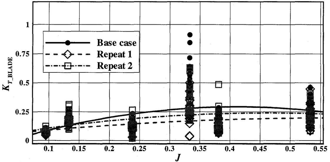
Figure 3-43: Maximum  $K_{T\_BLADE}$  from the repeat tests (an azimuthing angle of 180 degrees, a depth of cut of 15 mm)
