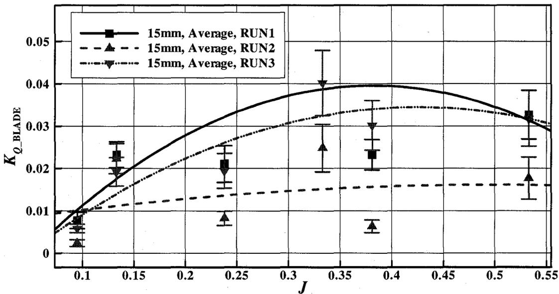
Figure 3-33:  $K_{Q\_BLADE}$ , average ice related loads, tractor mode, repeat runs (15mm)
