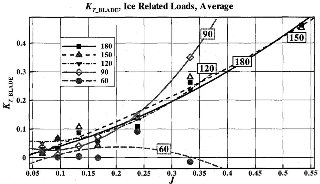
Figure C-10:  $K_{T\_BLADE}$  vs.  $J$ , average ice related loads at various azimuthing angles (180 ~ 60 degrees)
