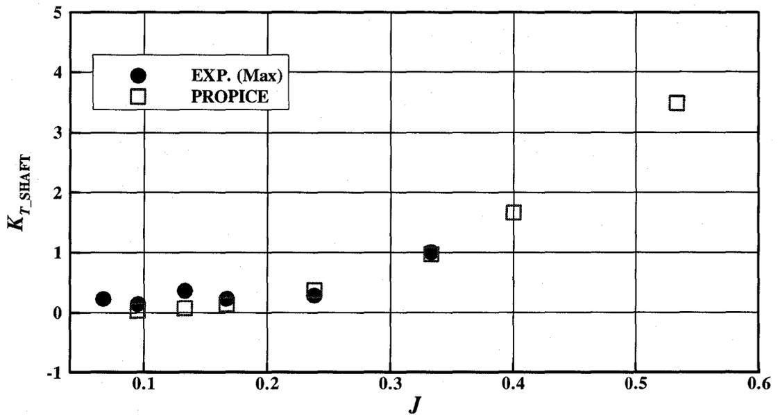
Figure E-3: Maximum  $K_{T\_SHAFT}$  comparison (ice related loads, azimuthing angle of 120 degrees, 35 mm depth of cut)
