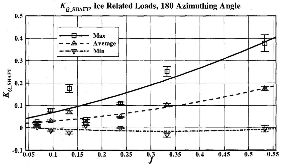
Figure C-2:  $K_{Q\_SHAFT}$  vs.  $J$ , maximum-average-minimum ice related loads with error bars
