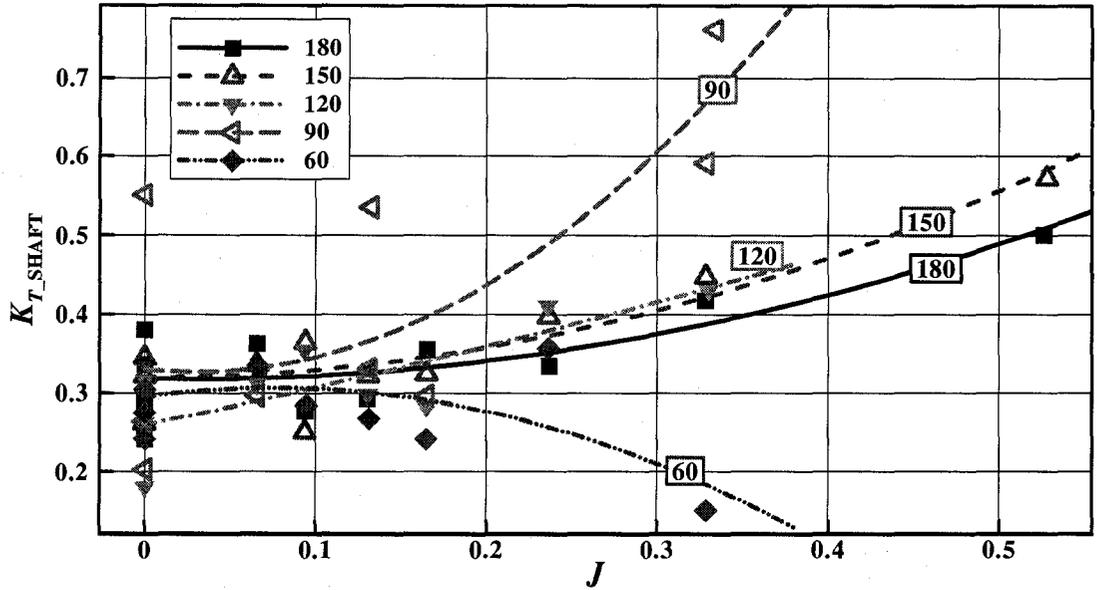
Figure D-11:  $K_{T\_SHAFT}$  vs.  $J$  at an azimuthing angle of 180 ~ 60 degrees in ice covered water
