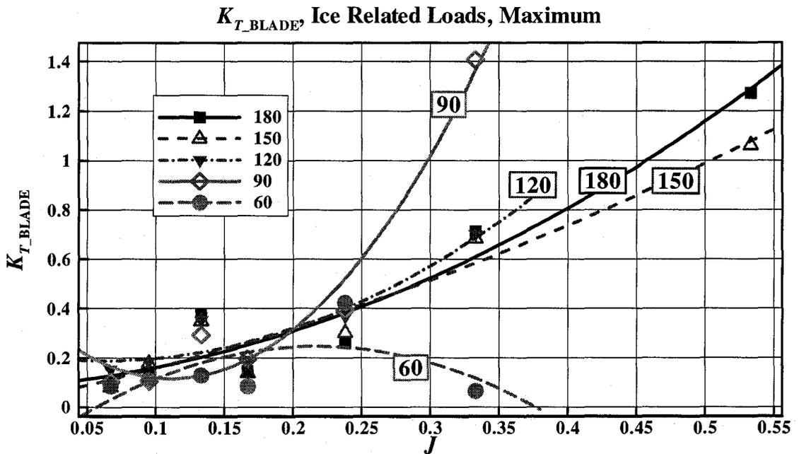
Figure C-17:  $K_{T\_BLADE}$  vs.  $J$ , maximum ice related loads at various azimuthing angles (180 ~ 60 degrees)
