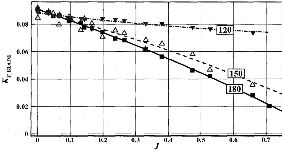
Figure B-17:  $K_{T\_BLADE}$  vs.  $J$  at various azimuthing angles (180–120 degrees) in open water
