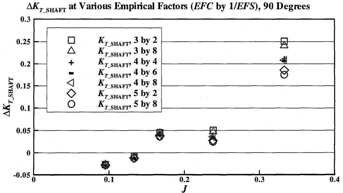
Figure 5-28:  $\Delta K_{T\_SHAFT}$  at various empirical factors ( $EFC$  by  $1/EFS$ ) with 90 degrees and 35 mm depth of cut
