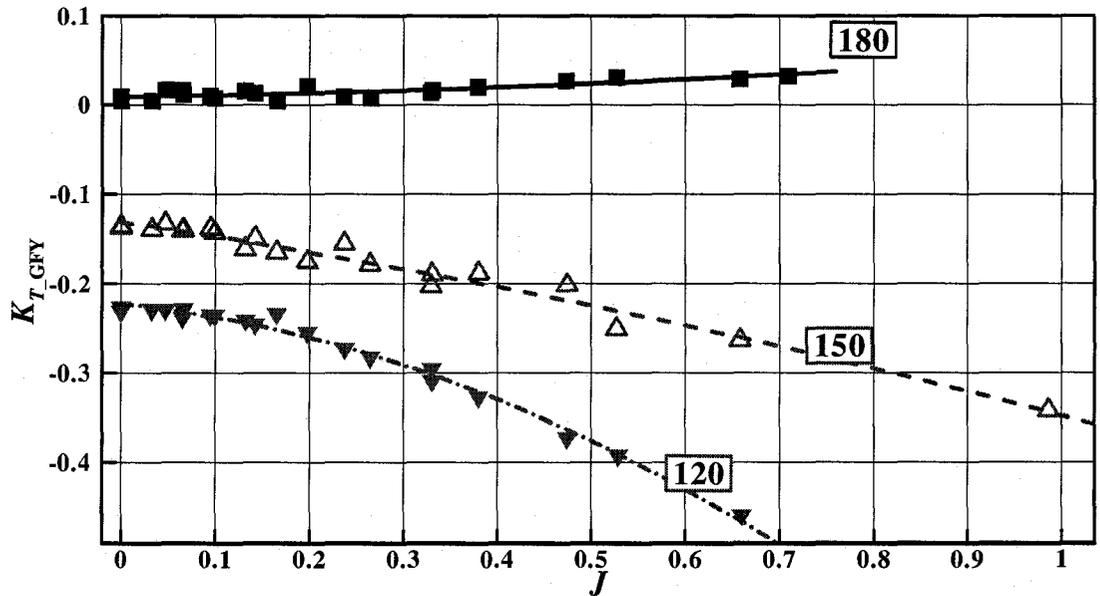
Figure B-10:  $K_{T\_GFY}$  vs.  $J$  at various azimuthing angles (180–120 degrees) in open water
