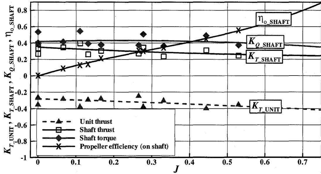
Figure B-26: Open water characteristics for tractor mode at 30° azimuthing angle
