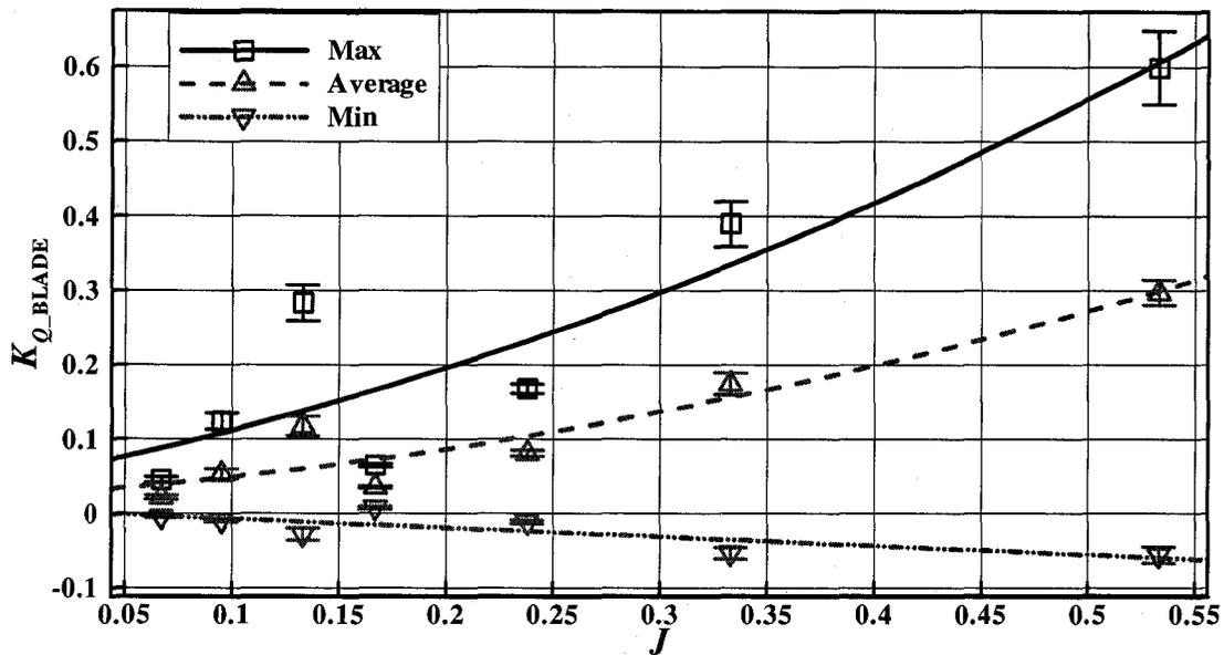
Figure C-4:  $K_{Q\_BLADE}$  vs.  $J$ , maximum-average-minimum ice related loads with error bars
