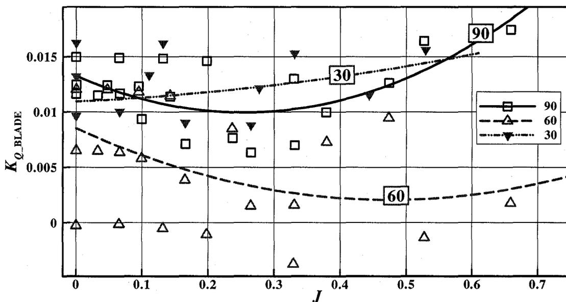
Figure B-20:  $K_{Q\_BLADE}$  vs.  $J$  at various azimuthing angles (90–30 degrees) in open water
