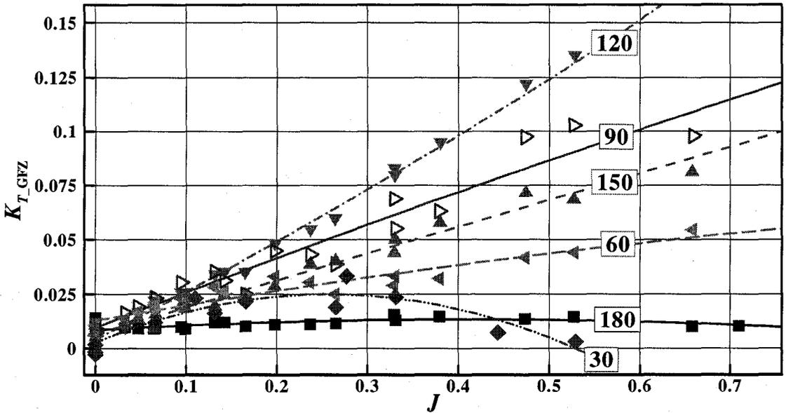
Figure B-12:  $K_{T\_GFZ}$  vs.  $J$  at various azimuthing angles (180~30 degrees) in open water
