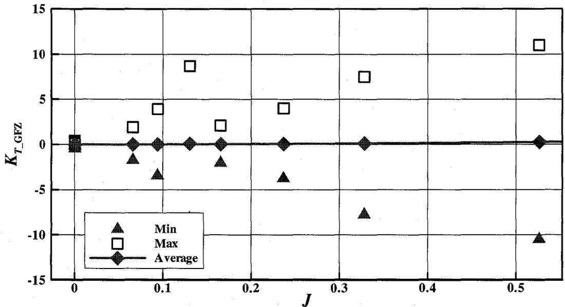
Figure D-3:  $K_{T\_GFZ}$  vs.  $J$  at an azimuthing angle of 180 degrees in ice covered water
