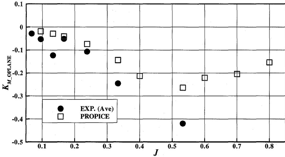
Figure 5-8:  $K_{M\_OPLANE}$  comparison (ice related loads, azimuthing angle of 180 degrees, 35 mm depth of cut, key blade only)
