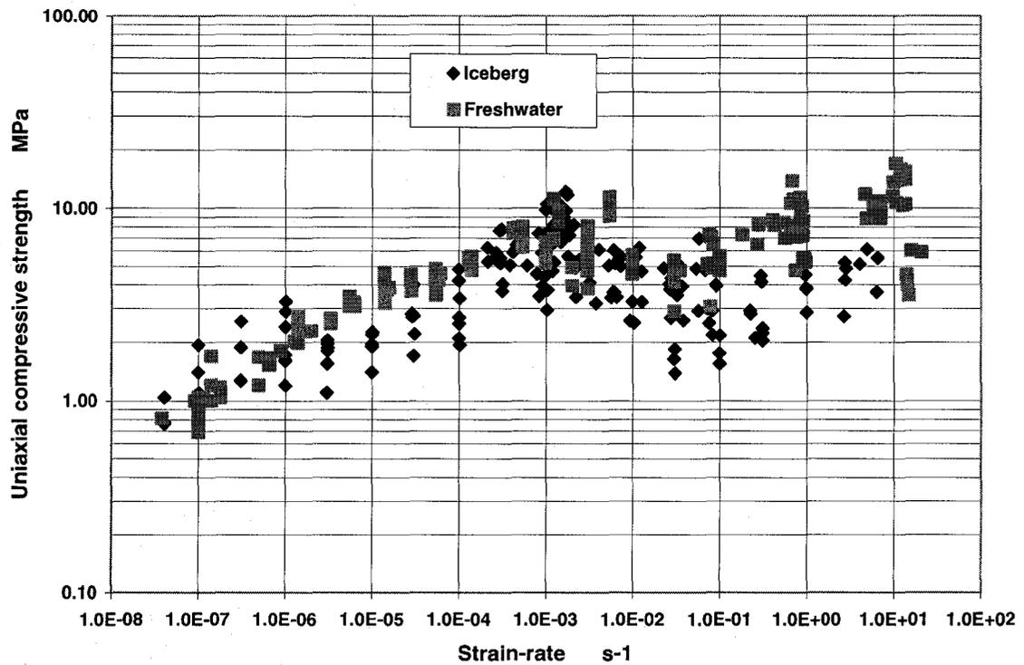
Figure 3-40: Uniaxial compressive strength vs. strain rate (after Jones, 2006)
