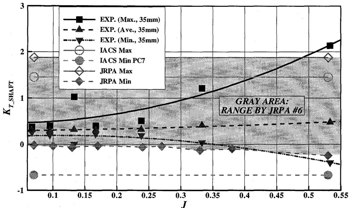
Figure 5-22:  $K_{T\_SHAFT}$  comparison among the present tests (maximum, minimum and average values), the JRPA #6 (maximum and minimum), and the IACS (maximum and minimum for the PC7)
