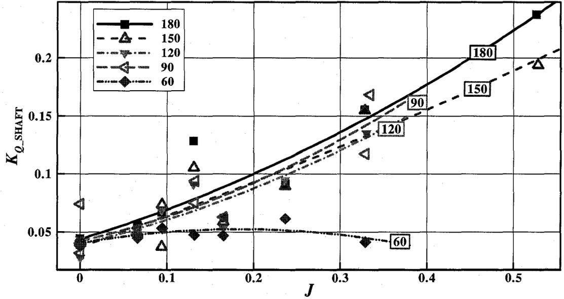
Figure D-12:  $K_{Q\_SHAFT}$  vs.  $J$  at an azimuthing angle of 180 ~ 60 degrees in ice covered water
