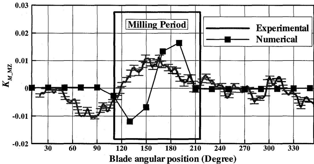
Figure 5-4: Time series comparison for  $K_{M\_MZ}$  (ice related loads,  $J= 0.238$ , 35mm)
