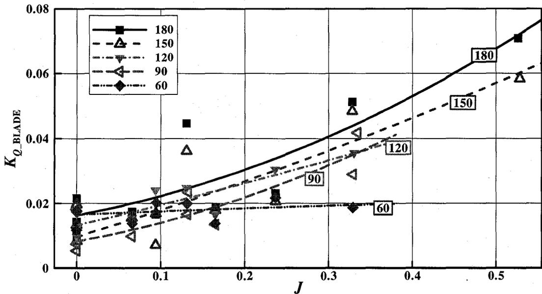
Figure D-14:  $K_{Q\_BLADE}$  vs.  $J$  at an azimuthing angle of 180 ~ 60 degrees in ice covered water
