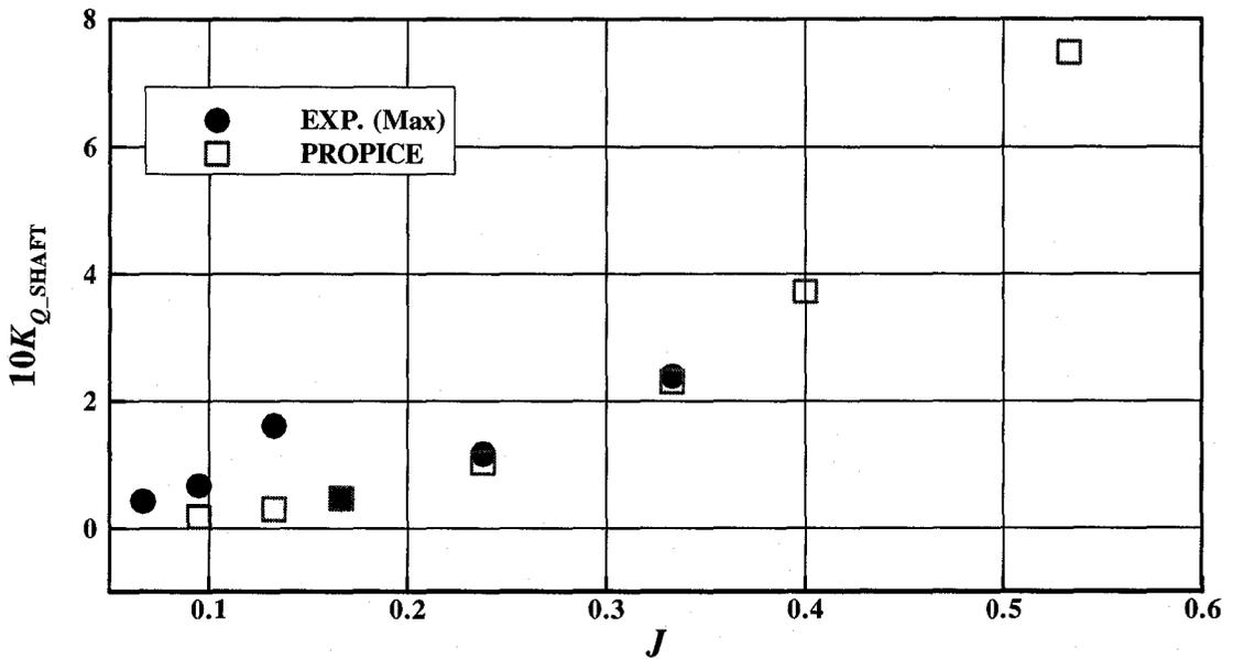
Figure E-7: Maximum  $10K_{Q\_SHAFT}$  comparison (ice related loads, azimuthing angle of 120 degrees, 35 mm depth of cut)
