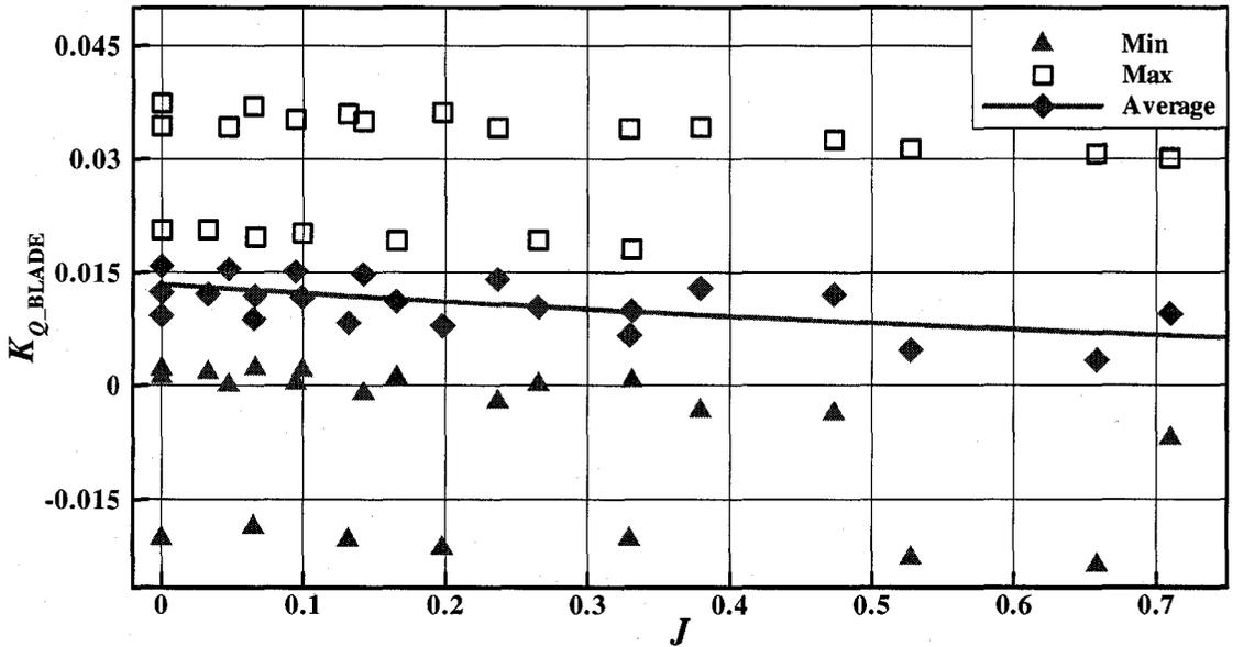
Figure B-7:  $K_{Q\_BLADE}$  vs.  $J$  at an azimuthing angle of 180 degrees in open water
