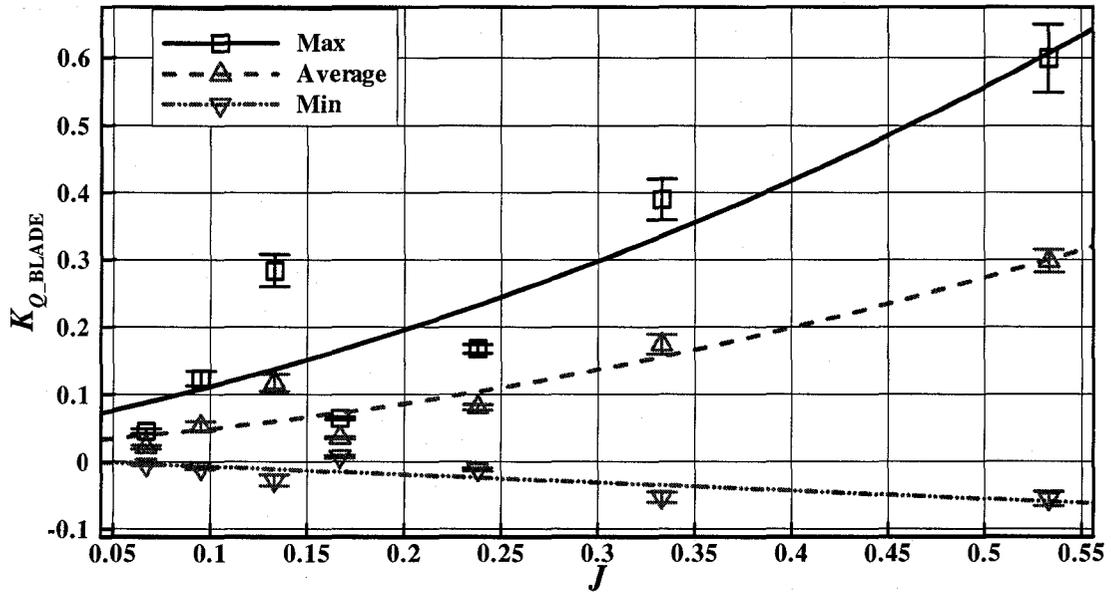
Figure 3-28:  $K_{Q\_BLADE}$ , ice related loads at an azimuthing angle of 180 degrees (tractor mode)
