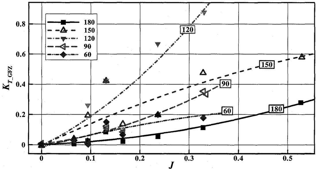
Figure D-10:  $K_{T\_GFZ}$  vs.  $J$  at an azimuthing angle of 180 ~ 60 degrees in ice covered water
