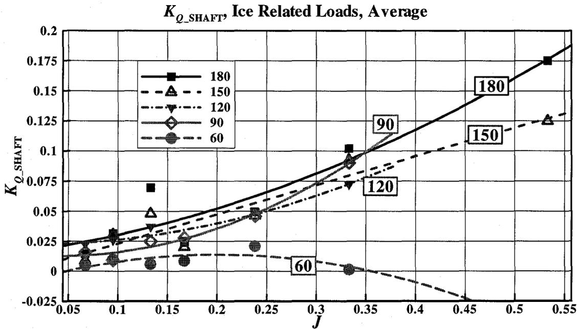
Figure C-9:  $K_{Q\_SHAFT}$  vs.  $J$ , average ice related loads at various azimuthing angles (180 ~ 60 degrees)
