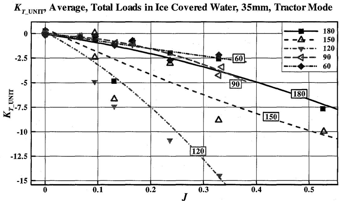
Figure D-8:  $K_{T\_UNIT}$  vs.  $J$  at an azimuthing angle of 180 ~ 60 degrees in ice covered water
