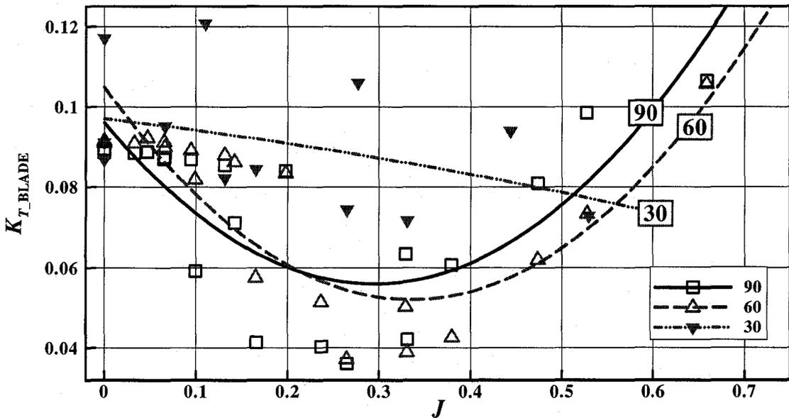
Figure B-18:  $K_{T\_BLADE}$  vs.  $J$  at various azimuthing angles (90–30 degrees) in open water
