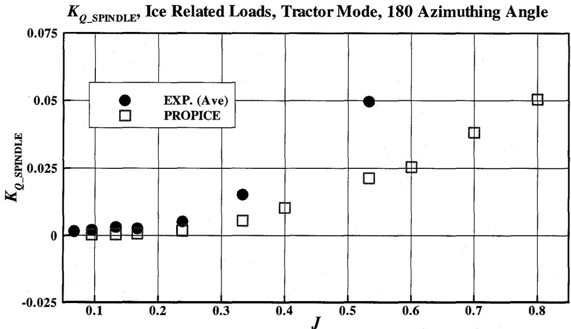
Figure 5-9:  $K_{Q\_SPINDLE}$  comparison (ice related loads, azimuthing angle of 180 degrees, 35 mm depth of cut, key blade only)
