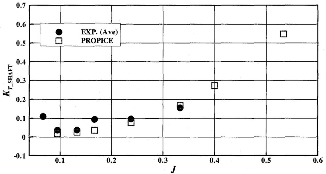
Figure 5-12:  $K_{T\_SHAFT}$  comparison (ice related loads, azimuthing angle of 120 degrees, 35 mm depth of cut)
