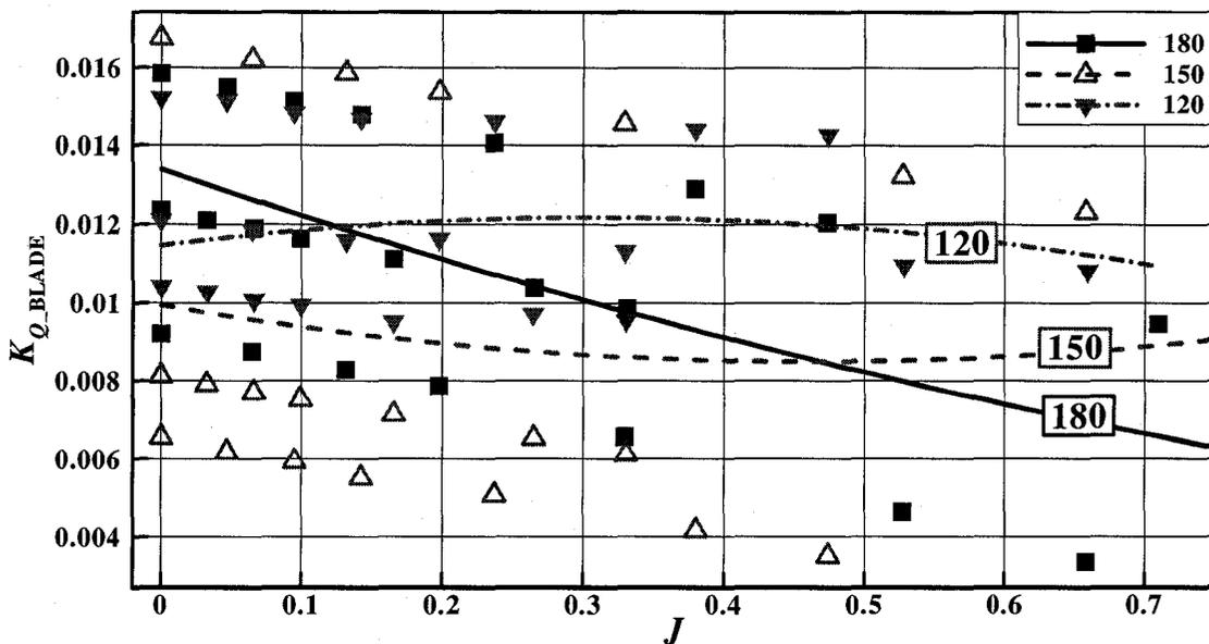
Figure B-19:  $K_{Q\_BLADE}$  vs.  $J$  at various azimuthing angles (180–120 degrees) in open water
