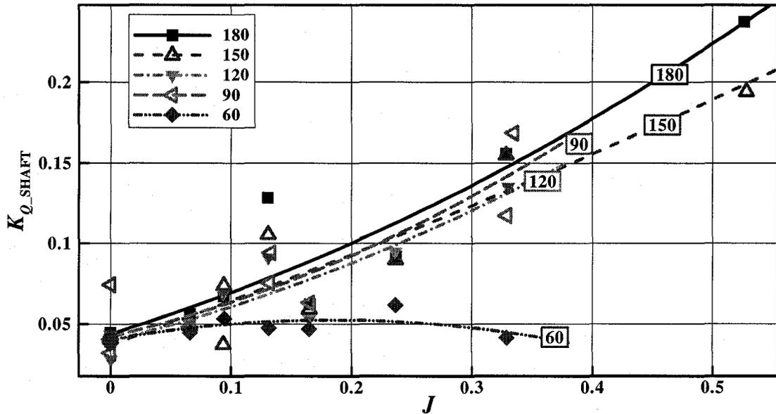
Figure 3-37:  $K_{Q\_SHAFT}$ , total loads at various azimuthing angles in ice covered water
