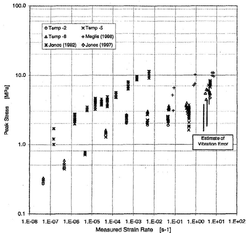
Figure 5-24: EG/AD/S compressive strength with three different temperatures and other types of ice from literatures against strain rate (after Moores, 2002)
