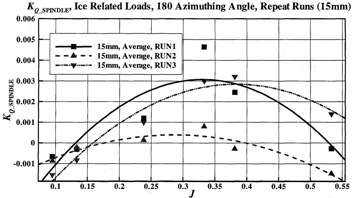
Figure C-28:  $K_{Q\_SPINDLE}$  vs.  $J$ , average ice related loads at 15mm depth of cut (repeated)
