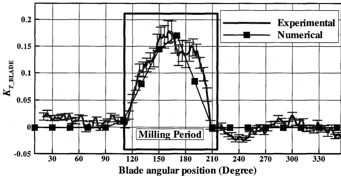
Figure 5-1: Time series comparison for  $K_{T\_BLADE}$  (ice related loads,  $J= 0.238$ , 35mm)
