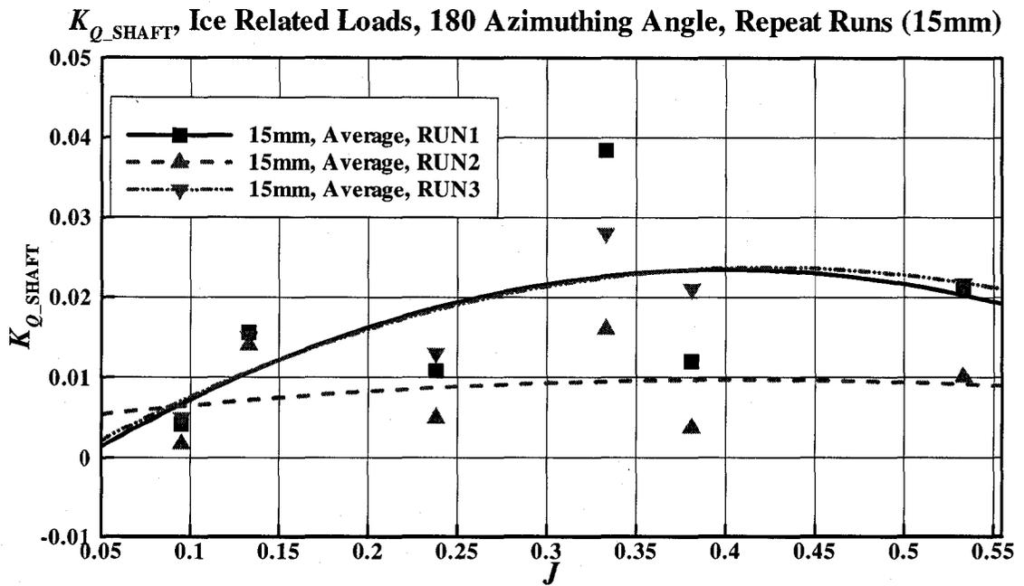
Figure C-23:  $K_{Q\_SHAFT}$  vs.  $J$ , average ice related loads at 15mm depth of cut (repeated)
