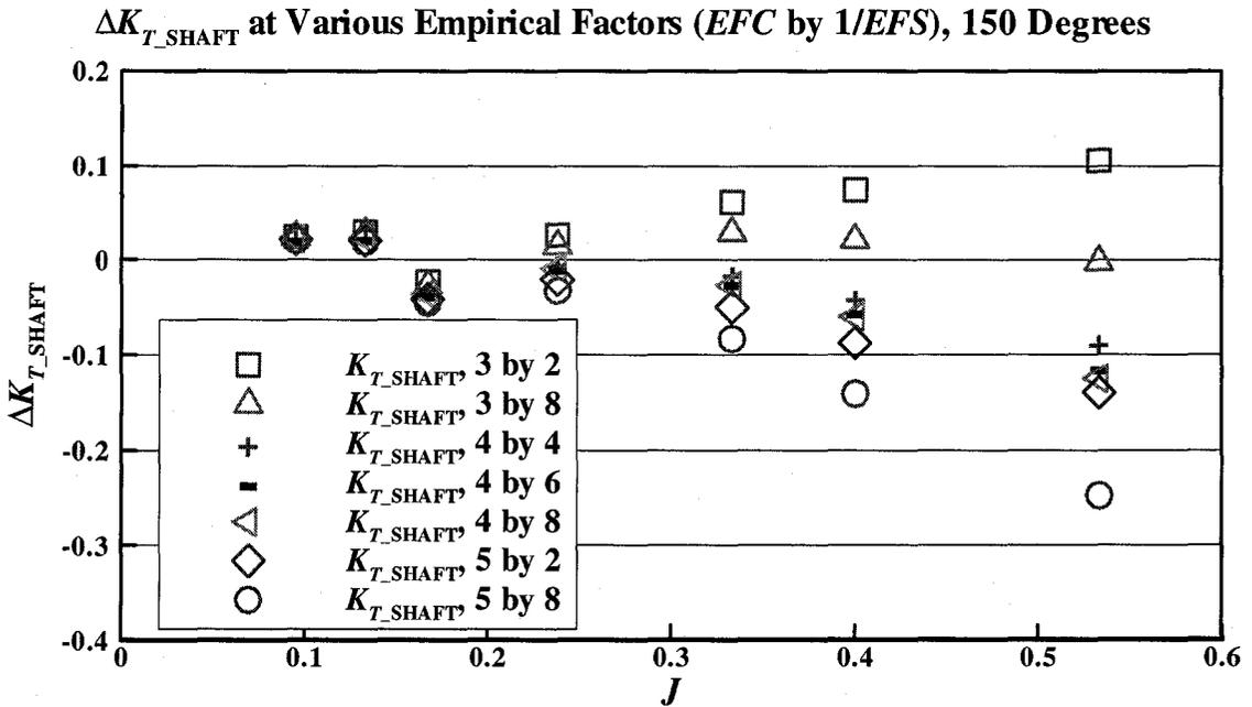
Figure 5-26:  $\Delta K_{T\_SHAFT}$  at various empirical factors (*EFC* by  $1/EFS$ ) with 150 degrees and 35 mm depth of cut
