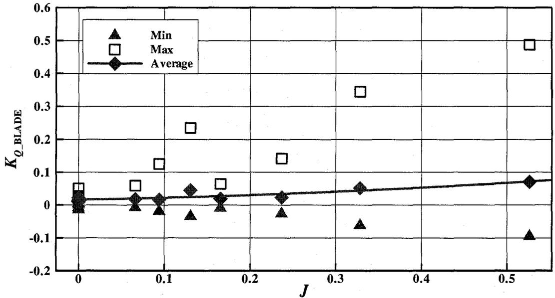
Figure D-7:  $K_{Q\_BLADE}$  vs.  $J$  at an azimuthing angle of 180 degrees in ice covered water
