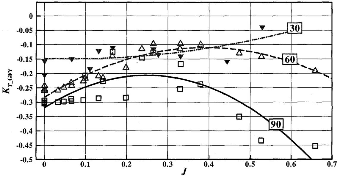
Figure B-11:  $K_{T\_GFY}$  vs.  $J$  at various azimuthing angles (90~30 degrees) in open water
