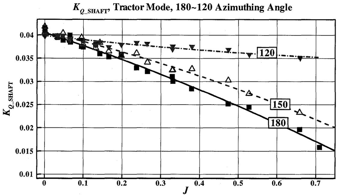
Figure B-15:  $K_{Q\_SHAFT}$  vs.  $J$  at various azimuthing angles (180–120 degrees) in open water
