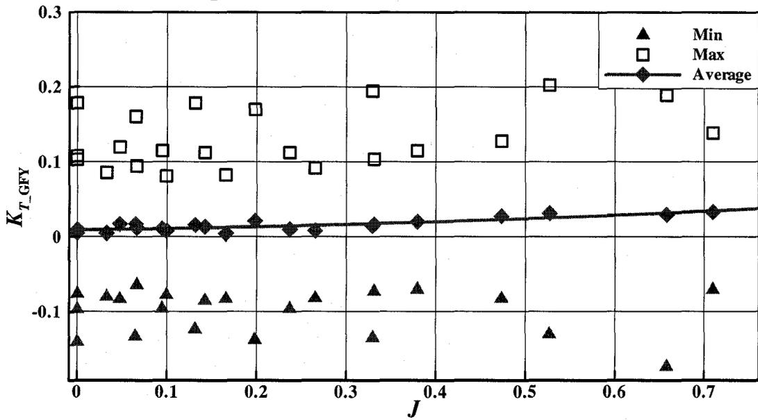
Figure B-2:  $K_{T\_GFY}$  vs.  $J$  at an azimuthing angle of 180 degrees in open water
