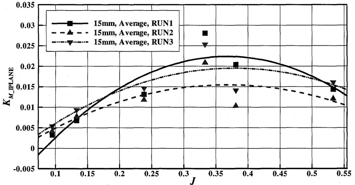
Figure C-26:  $K_{M\_IPLANE}$  vs.  $J$ , average ice related loads at 15mm depth of cut (repeated)
