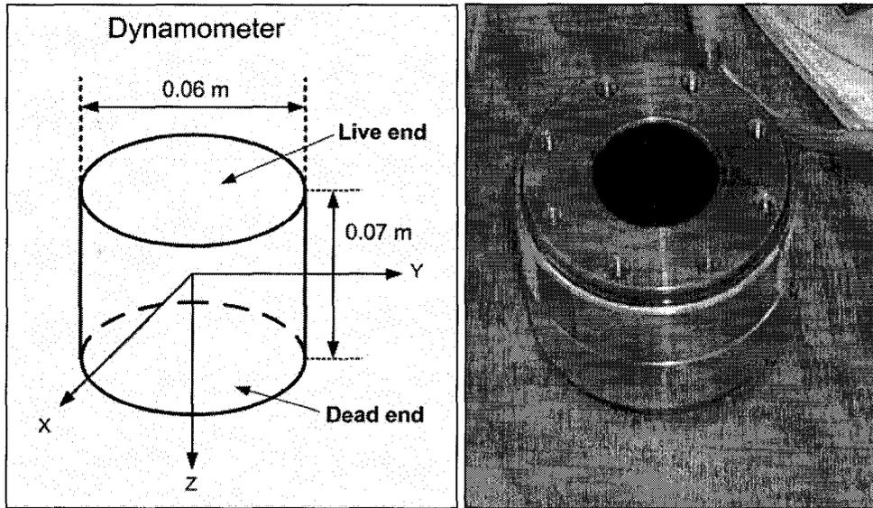
Figure 3-10: Dimension of AMTI dynamometer
