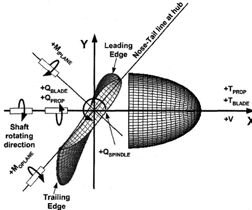
Figure 3-20: Sign conventions for the loads acting on the blade (look from the center of hub)
