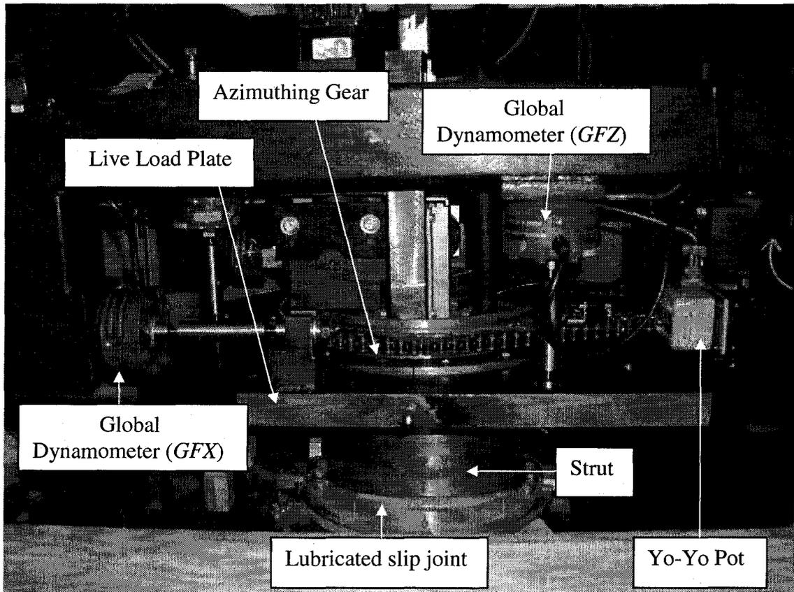
Figure 3-8: Apparatus of global dynamometer and azimuthing gear
