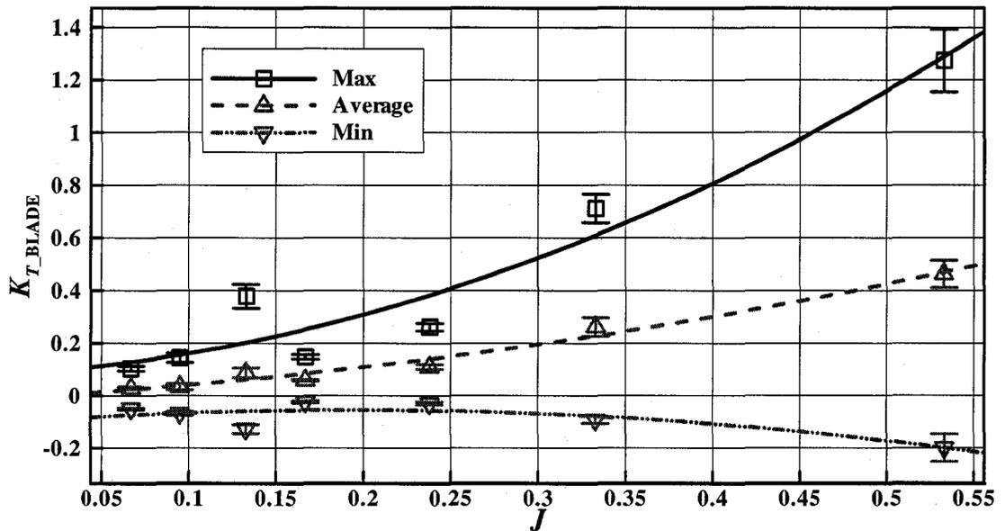
Figure 3-27:  $K_{T\_BLADE}$ , ice related loads at an azimuthing angle of 180 degrees (tractor mode)
