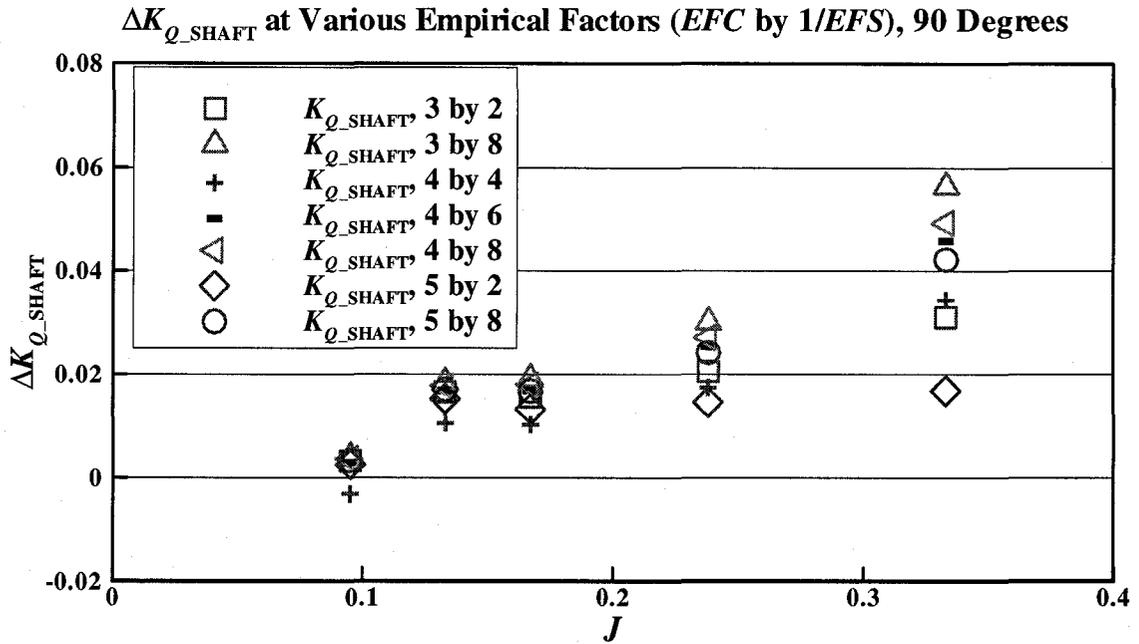
Figure 5-33:  $\Delta K_{Q\_SHAFT}$  at various empirical factors ( $EFC$  by  $1/EFS$ ) with 90 degrees and 35 mm depth of cut
