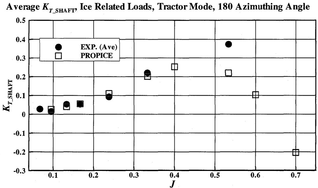
Figure 5-10:  $K_{T\_SHAFT}$  comparison (ice related loads, azimuthing angle of 180 degrees, 35 mm depth of cut)
