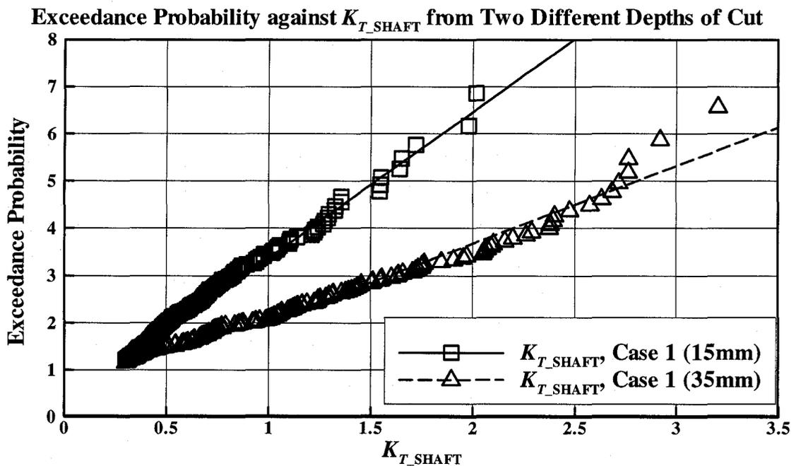
Figure 3-46: Exceedance probability against shaft thrust coefficients at two different depths of cut in “Case 1”
