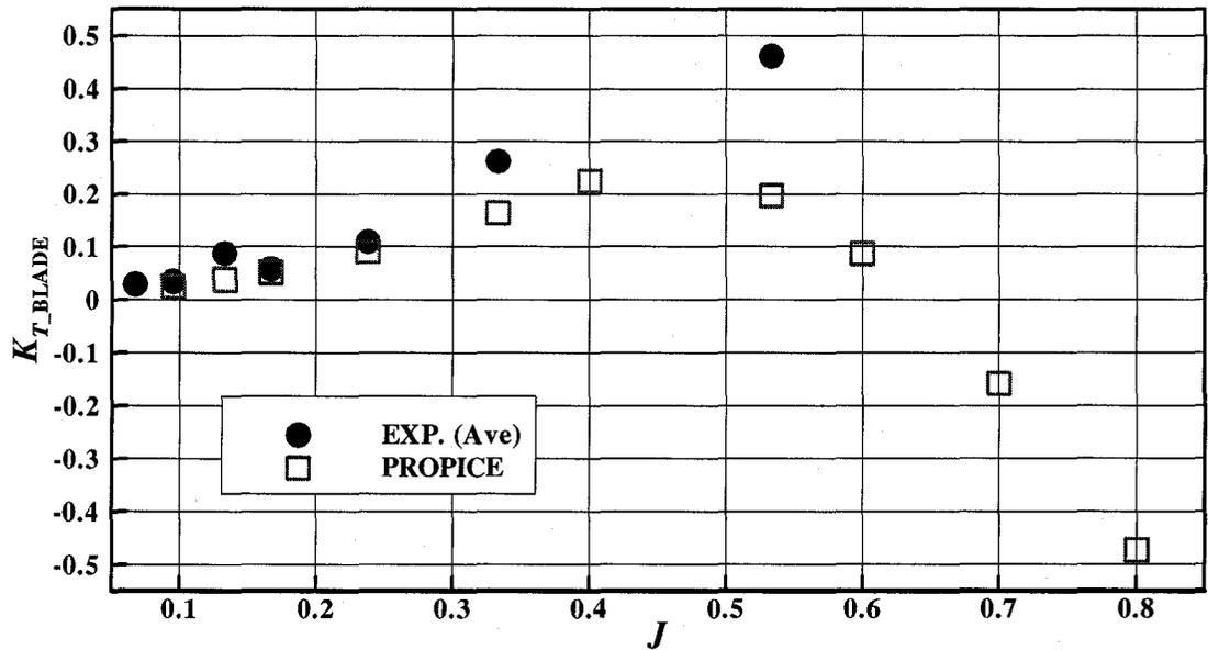
Figure 5-5:  $K_{T\_BLADE}$  comparison (ice related loads, azimuthing angle of 180 degrees, 35 mm depth of cut, key blade only)
