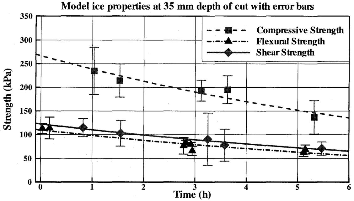
Figure 3-2: Model ice properties at the depth of cut of 35 mm with error bars ( $\pm 2$  times standard deviations)
