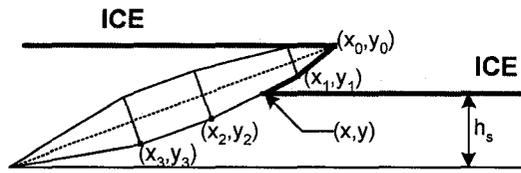
Figure 2-3: Intersection shape of the propeller blade (after Kotras et al., 1985)
