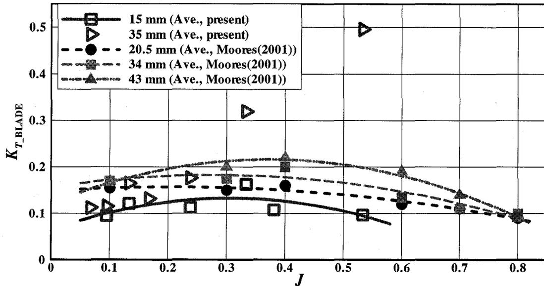
Figure 3-38: Comparison of average blade thrust coefficient ( $K_{T\_BLADE}$ , one blade only) with previous test results (ice-related loads + separable hydrodynamic loads during a milling period). The lines are the 2<sup>nd</sup> order polynomial lines of best fit
