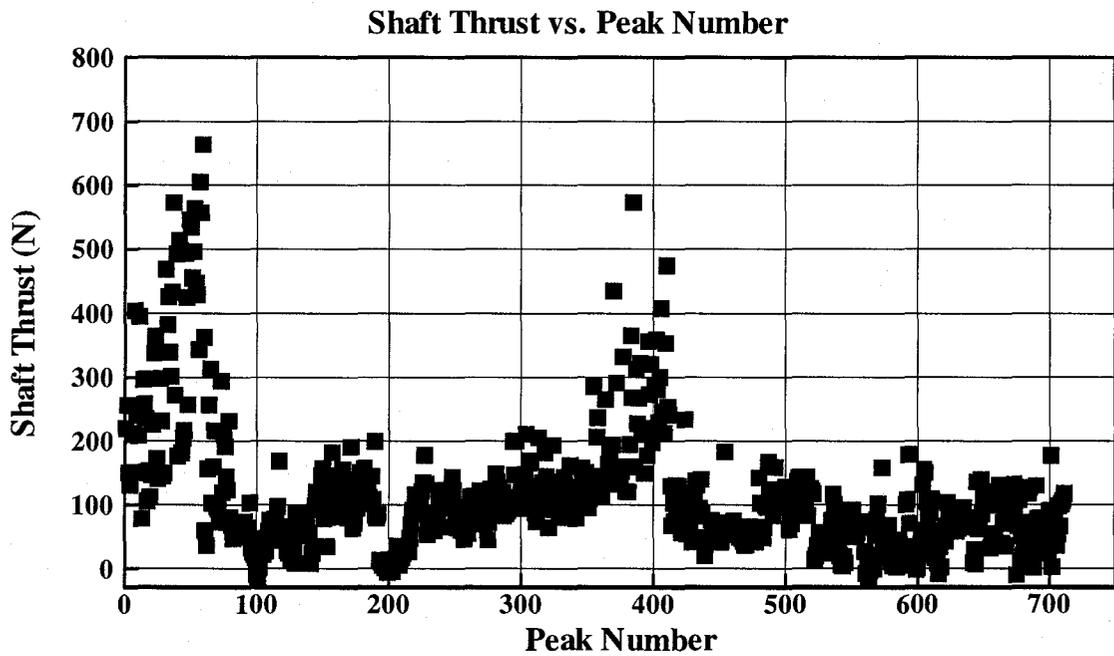
Figure 3-44: Measured maximum total force values for the assumed ice interaction segments in the time series for the selected test run (Case 1)
