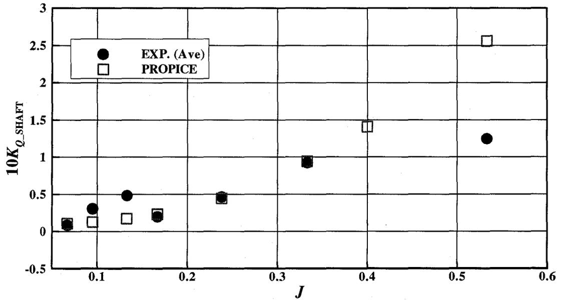
Figure 5-15:  $10K_{Q\_SHAFT}$  comparison (ice related loads, azimuthing angle of 150 degrees, 35 mm depth of cut)
