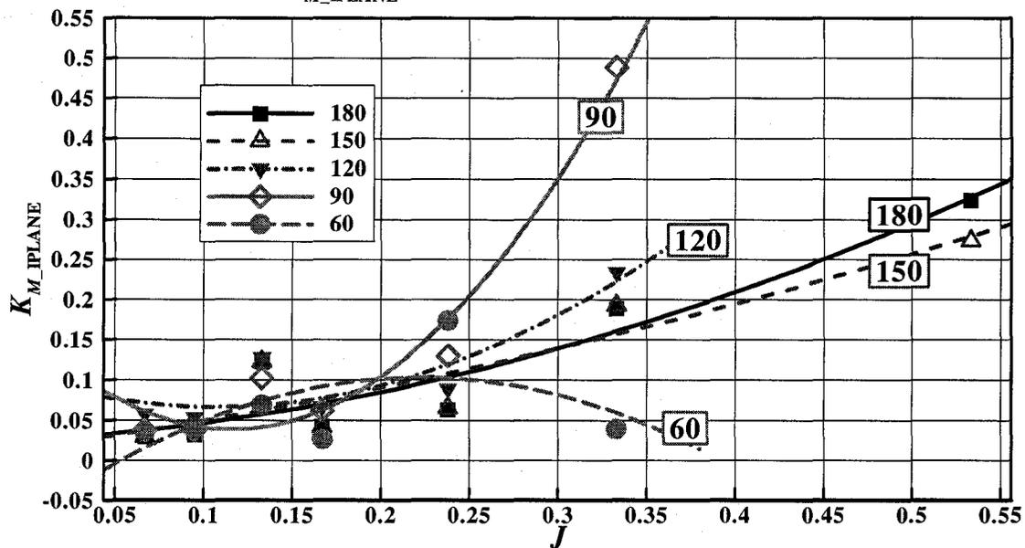
Figure C-19:  $K_{M\_IPLANE}$  vs.  $J$ , maximum ice related loads at various azimuthing angles (180 ~ 60 degrees)
