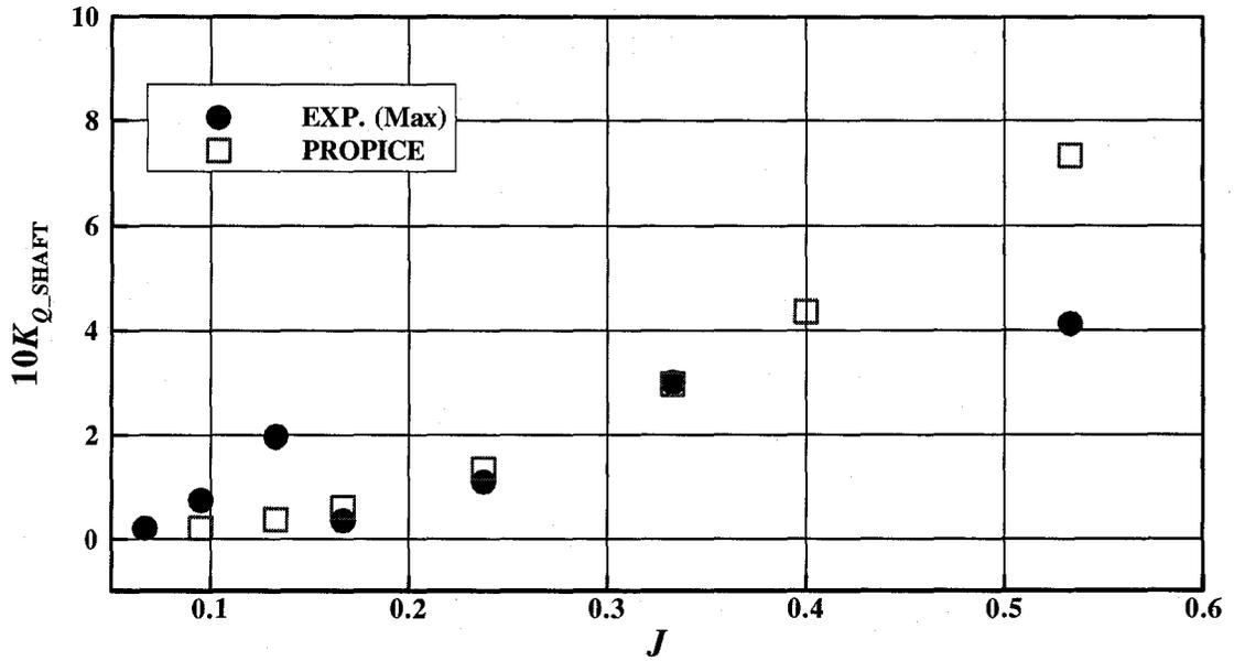
Figure E-6: Maximum  $10K_{Q\_SHAFT}$  comparison (ice related loads, azimuthing angle of 150 degrees, 35 mm depth of cut)
