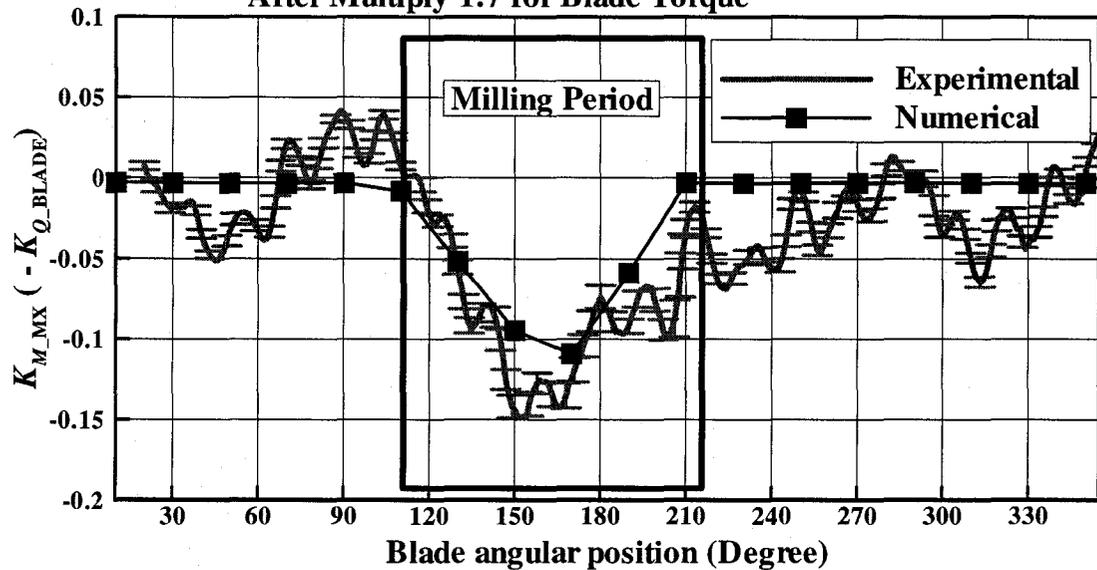
Figure 5-2: Time series comparison for  $K_{M\_MX}$  after multiplying 1.7 for the blade torque (ice related loads,  $J= 0.238$ , 35mm)
