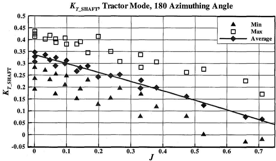
Figure B-4:  $K_{T\_SHAFT}$  vs.  $J$  at an azimuthing angle of 180 degrees in open water
