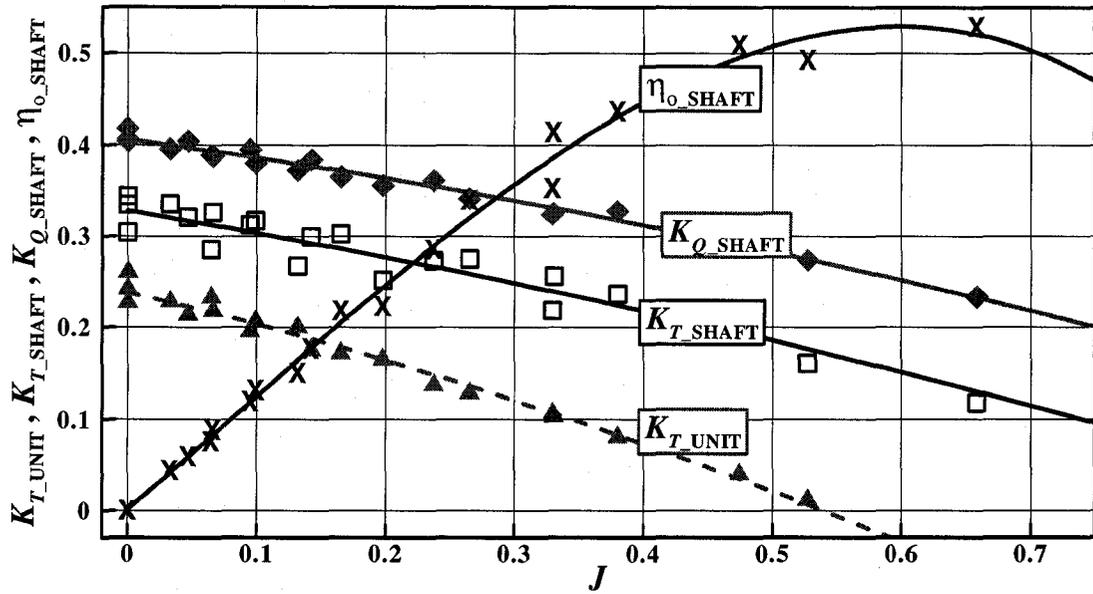
Figure B-22: Open water characteristics for tractor mode at 150° azimuthing angle
