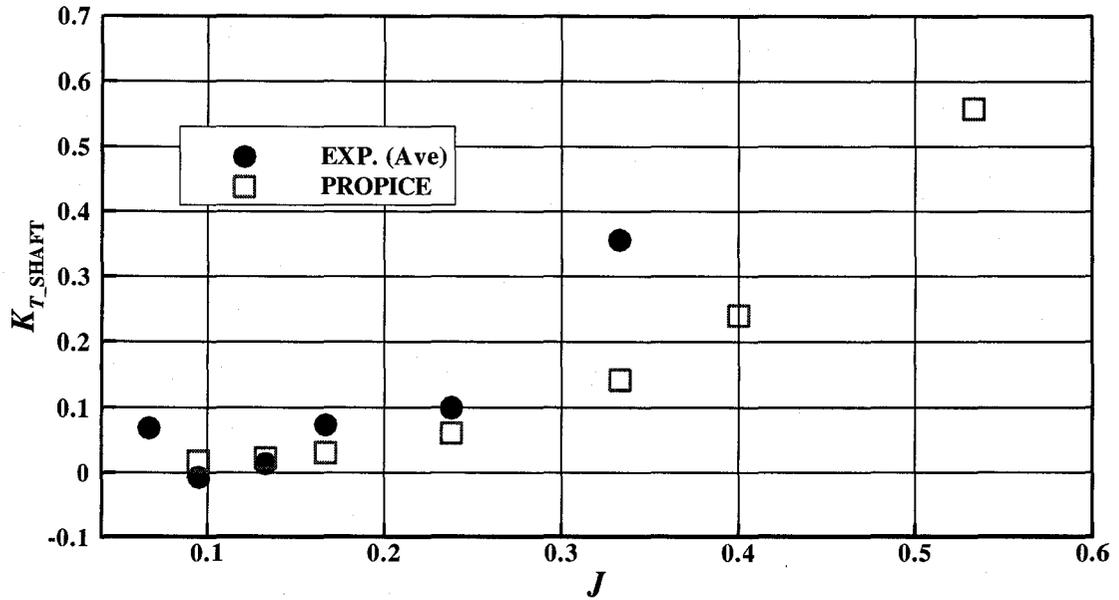
Figure 5-13:  $K_{T\_SHAFT}$  comparison (ice related loads, azimuthing angle of 90 degrees, 35 mm depth of cut)
