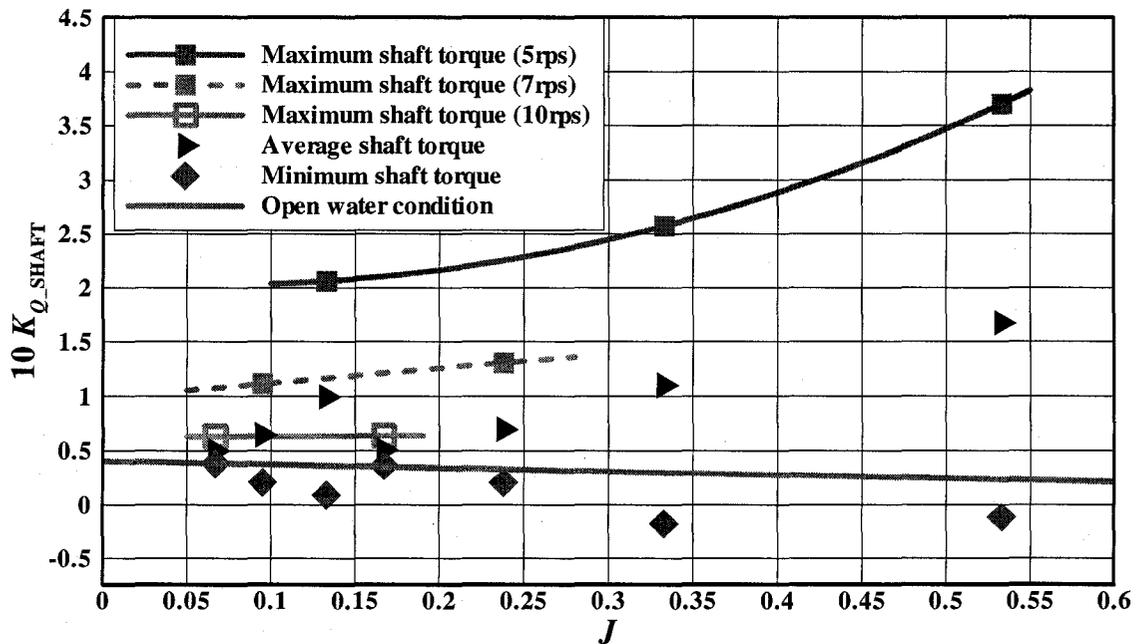
Figure 3-42: Maximum, minimum and average  $K_{Q\_SHAFT}$  for the 35mm depth of cut (ice-related loads + separable hydrodynamic loads during milling period) and open water
