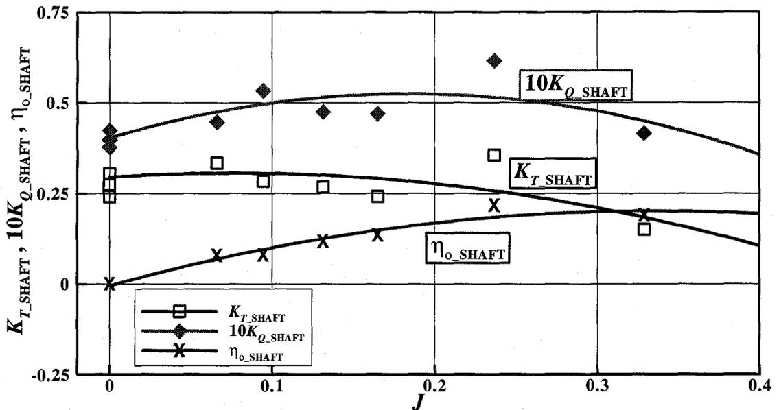
Figure D-19: Ice covered water characteristics for a tractor mode at an azimuthing angle of 60 degrees
