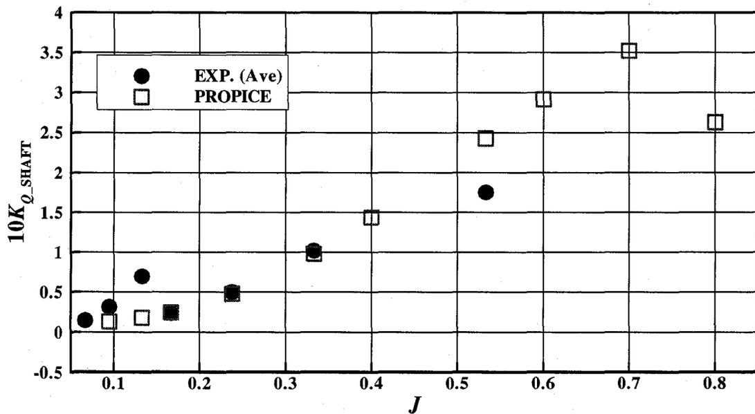
Figure 5-14:  $10K_{Q\_SHAFT}$  comparison (ice related loads, azimuthing angle of 180 degrees, 35 mm depth of cut)
