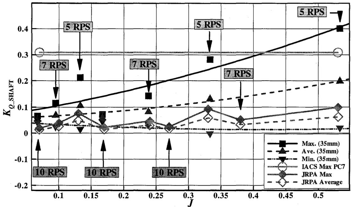
Figure 5-23:  $K_{Q\_SHAFT}$  comparison among the present tests (maximum, minimum and average values), the JRPA #6 (maximum and average), and the IACS (maximum for the PC7)
