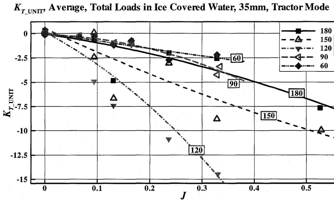
Figure 3-35:  $K_{T\_UNIT}$ , total loads at various azimuthing angles in ice covered water
