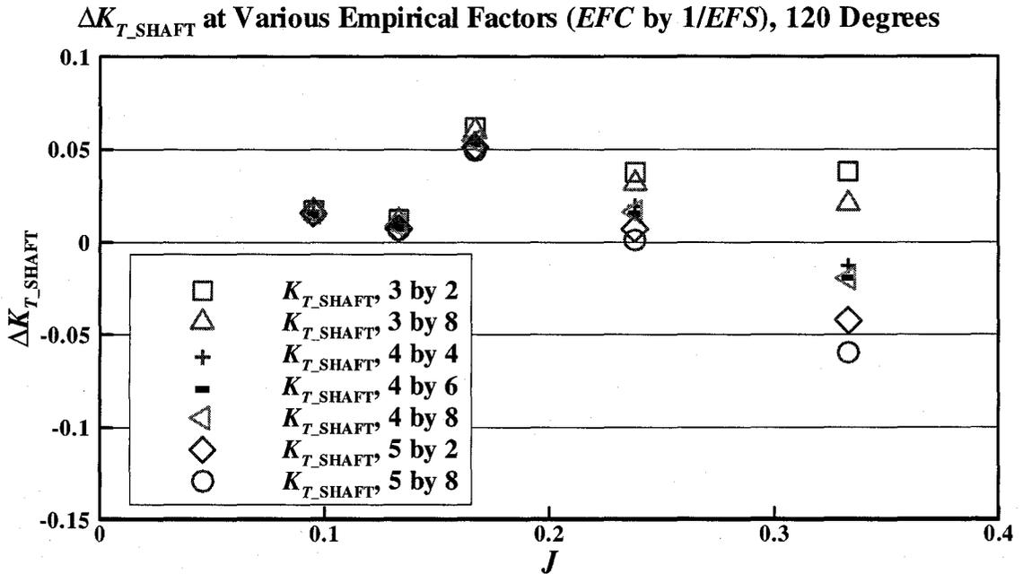
Figure 5-27:  $\Delta K_{T\_SHAFT}$  at various empirical factors (*EFC* by  $1/EFS$ ) with 120 degrees and 35 mm depth of cut
