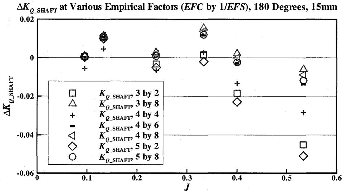
Figure 5-34:  $\Delta K_{Q\_SHAFT}$  at various empirical factors ( $EFC$  by  $1/EFS$ ) with 180 degrees and 15 mm depth of cut
