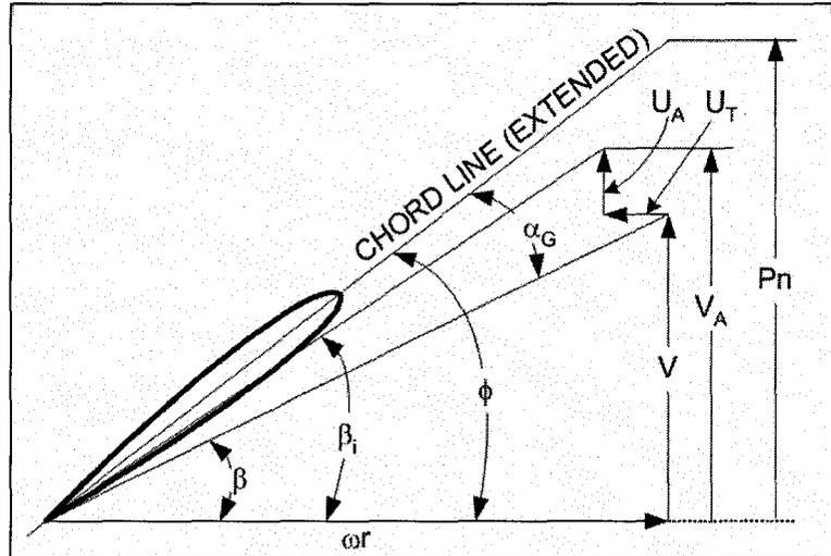
Figure 4-6: Velocity diagram for a propeller blade section,  $\beta$  is the angle of advance,  $\beta_i$  is the hydrodynamic pitch angle,  $\phi$  is the geometric pitch angle,  $\alpha_G$  is the geometric angle of attack,  $V$  is the carriage speed,  $V_A$  is the advance speed,  $U_T$  and  $U_A$  are the tangential and axial induced velocities, and  $P$  is the pitch at  $0.7R$
