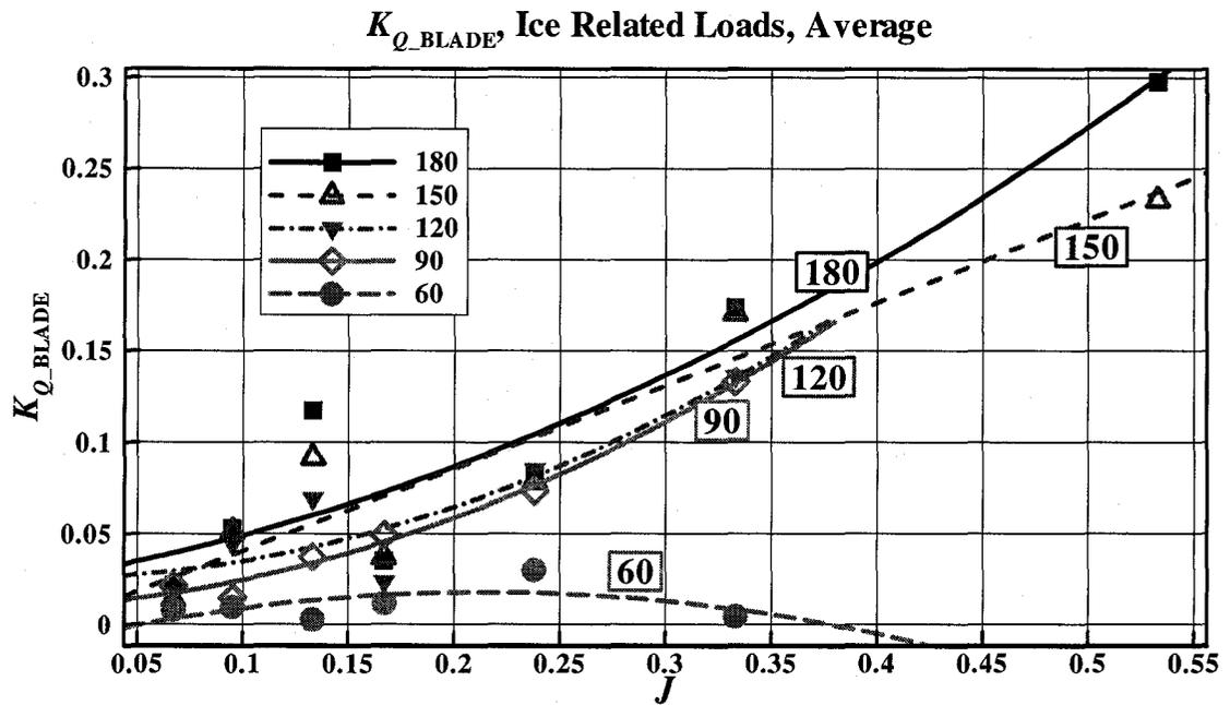
Figure C-11:  $K_{Q\_BLADE}$  vs.  $J$ , average ice related loads at various azimuthing angles (180 ~ 60 degrees)
