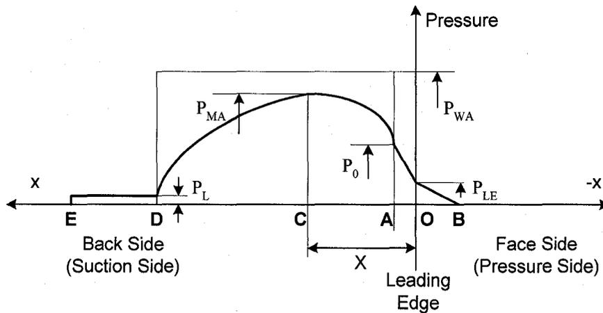
Figure 2-10: Pressure distributions (after Soininen, 1998)
