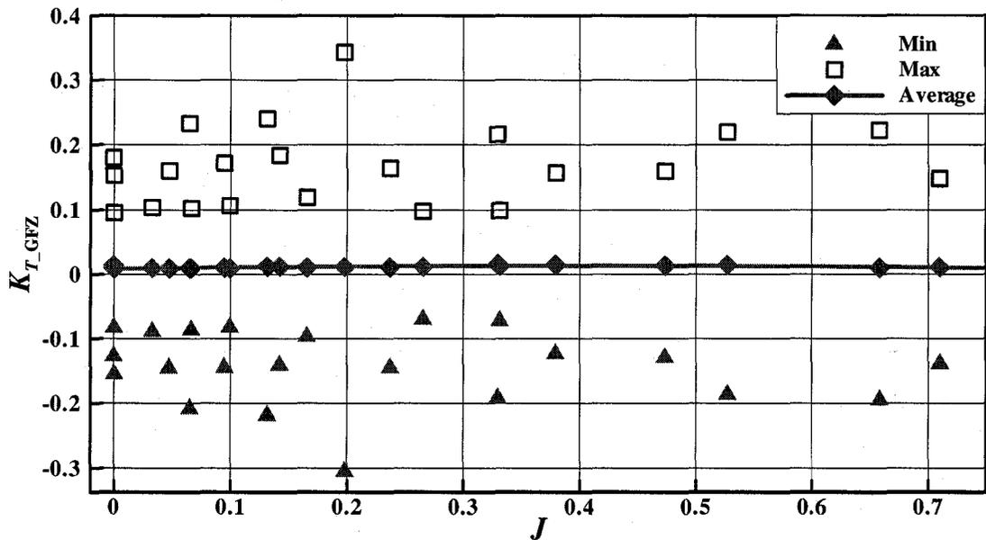
Figure B-3:  $K_{T\_GFZ}$  vs.  $J$  at an azimuthing angle of 180 degrees in open water
