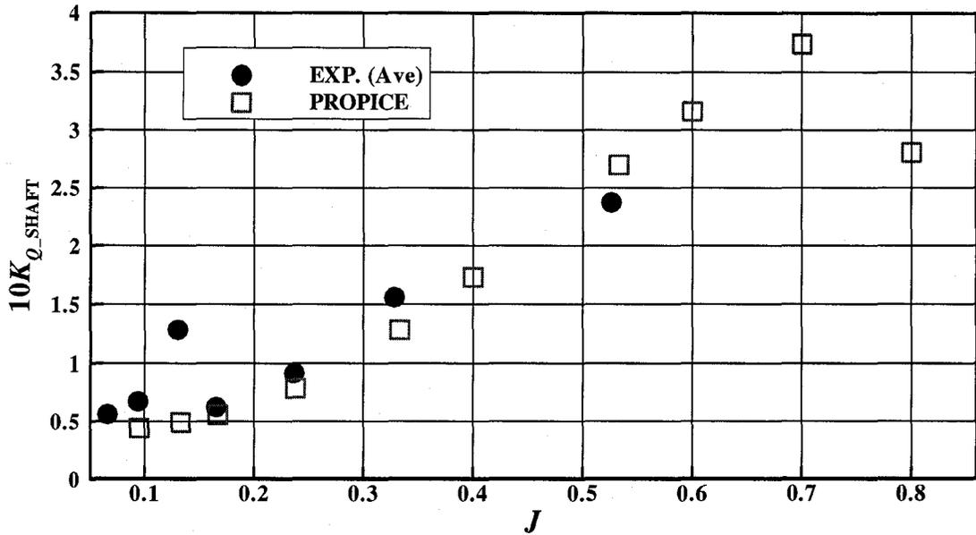
Figure 5-19:  $10K_{Q\_SHAFT}$  comparison (Total loads, azimuthing angle of 180 degrees, 35 mm depth of cut)
