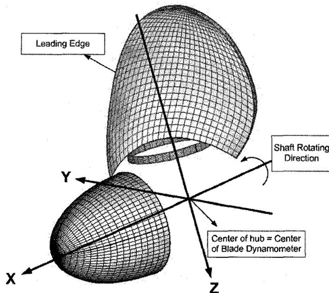
Figure 3-11: Axes for blade dynamometer
