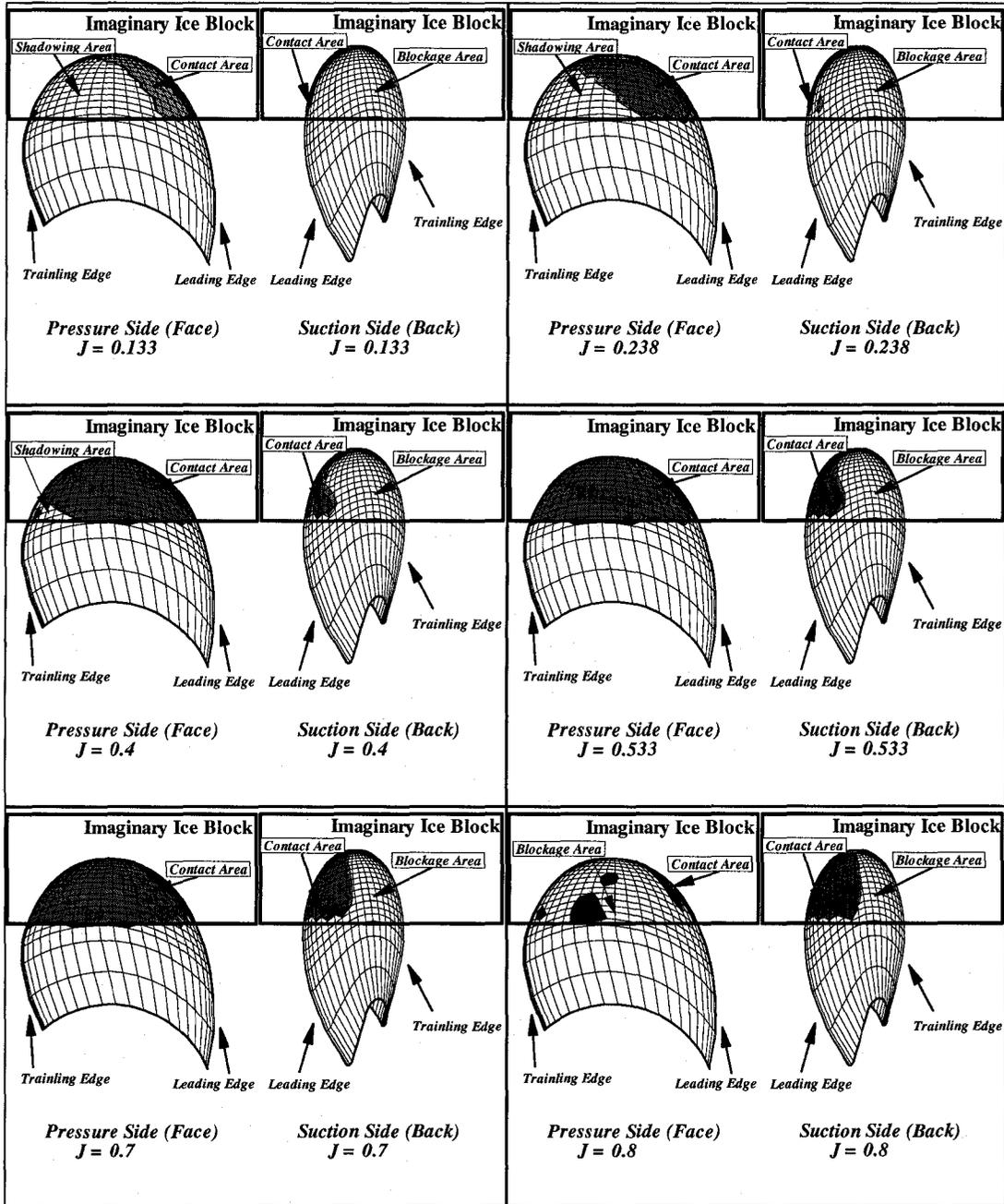
Figure 5-21: Calculated pressure distribution on the pressure and suction side of the blade (from top left,  $J = 0.133, 0.238, 0.4, 0.533, 0.7$  and  $0.8$ )
