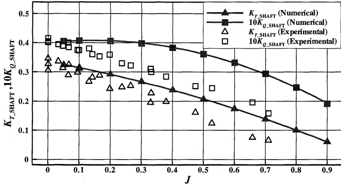
Figure 4-4: Comparison of results from panel method with those from the experiments in open water conditions
