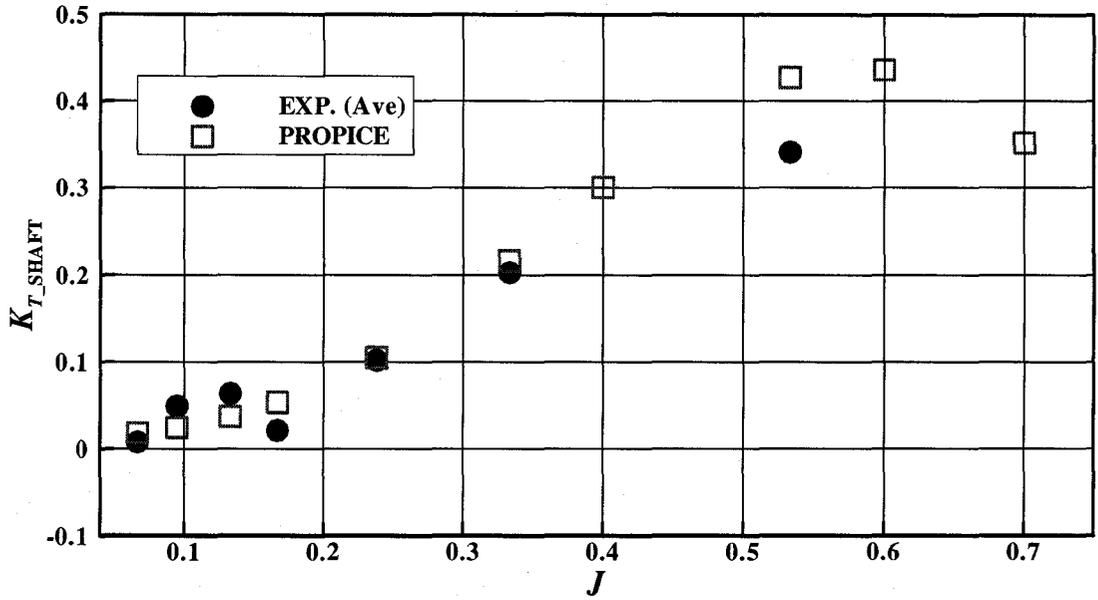
Figure 5-11:  $K_{T\_SHAFT}$  comparison (ice related loads, azimuthing angle of 150 degrees, 35 mm depth of cut)
