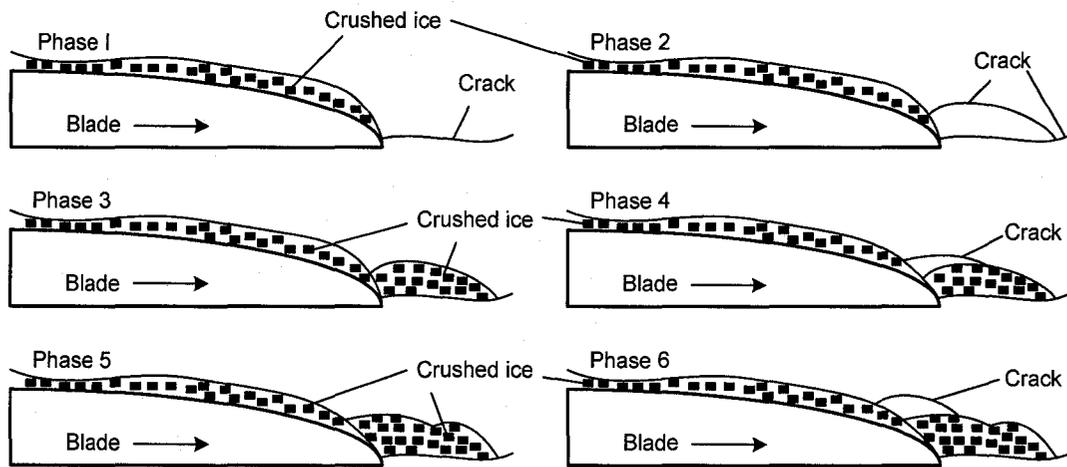
Figure 2-8: Ice crushing on back side (after Soininen, 1998)
