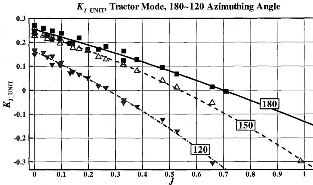
Figure B-8:  $K_{T\_UNIT}$  vs.  $J$  at various azimuthing angles (180–120 degrees) in open water
