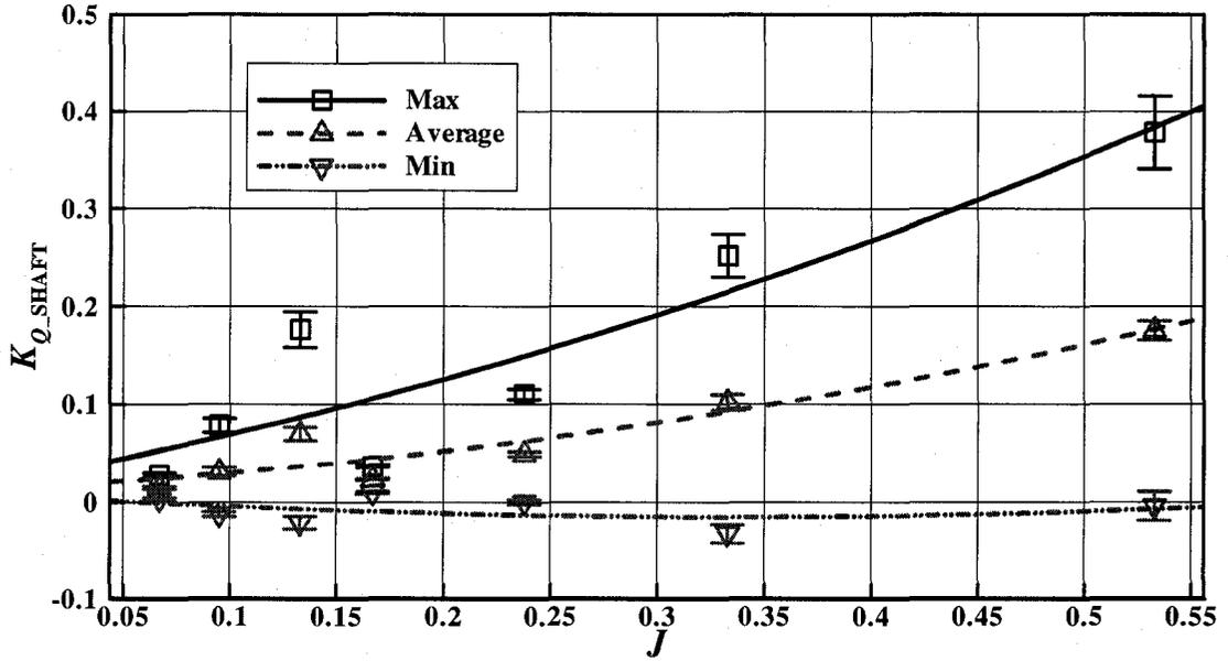
Figure 3-26:  $K_{Q\_SHAFT}$ , ice related loads at an azimuthing angle of 180 degrees (tractor mode)
