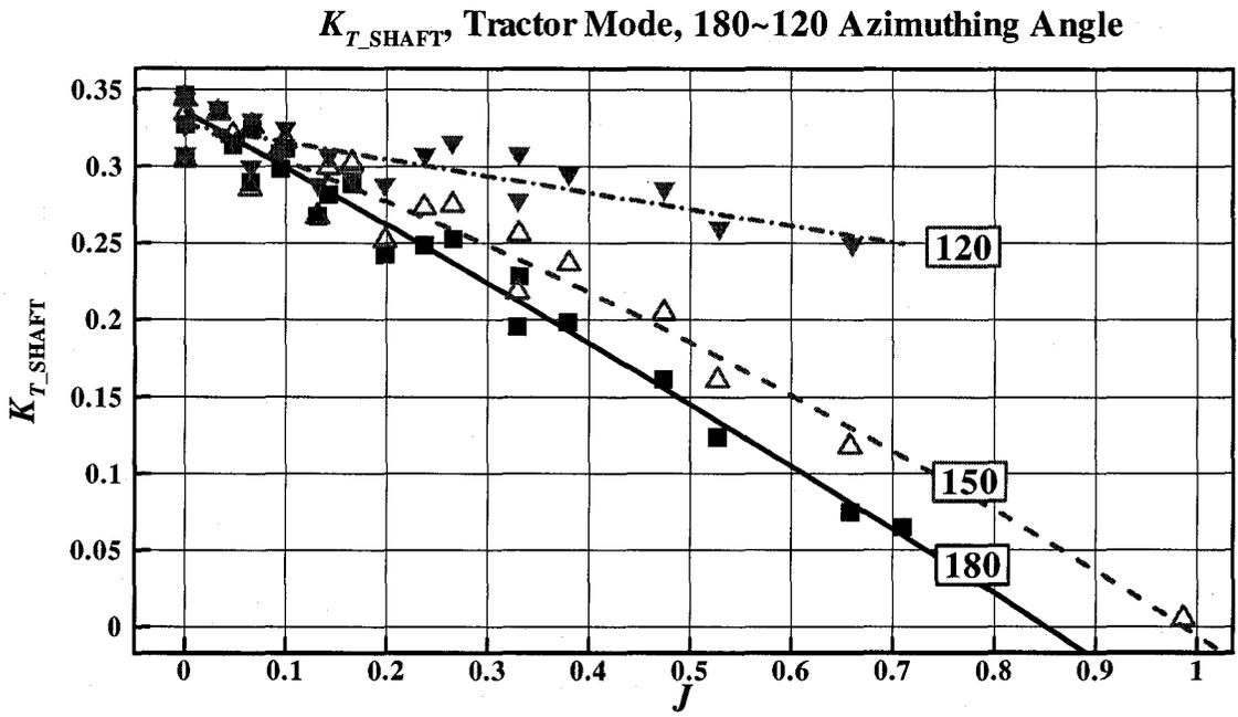
Figure B-13:  $K_{T\_SHAFT}$  vs.  $J$  at various azimuthing angles (180–120 degrees) in open water
