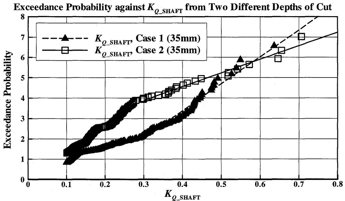
Figure 3-48: Exceedance probability against shaft torque coefficients at two Cases
