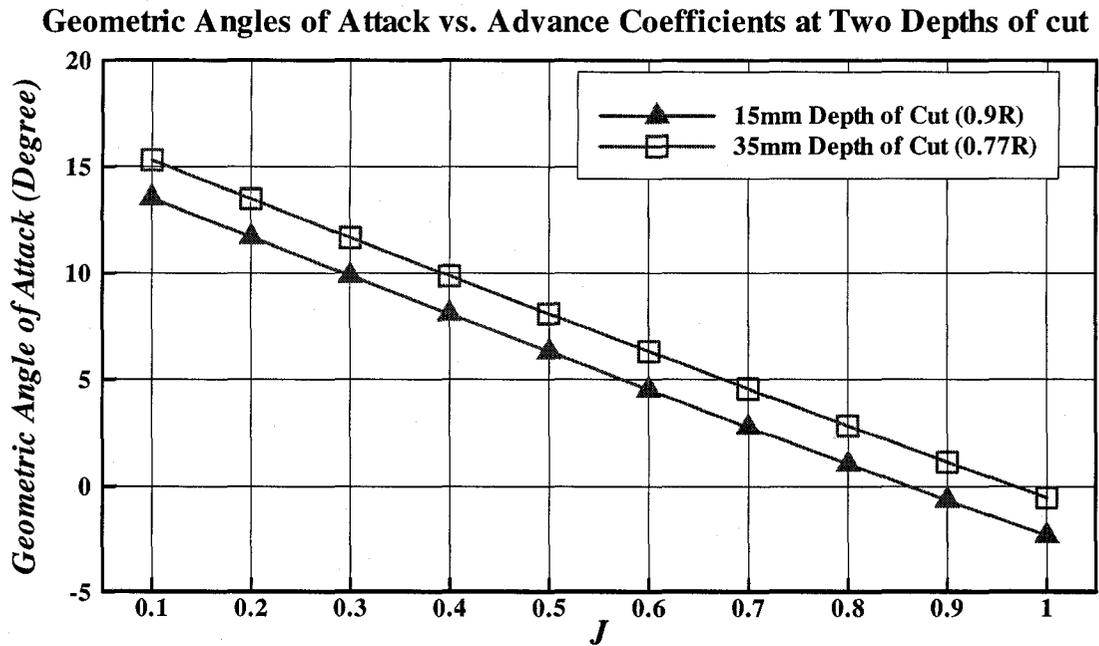
Figure 3-34: Geometric angles of attack vs. advance coefficients at two depths of cut
