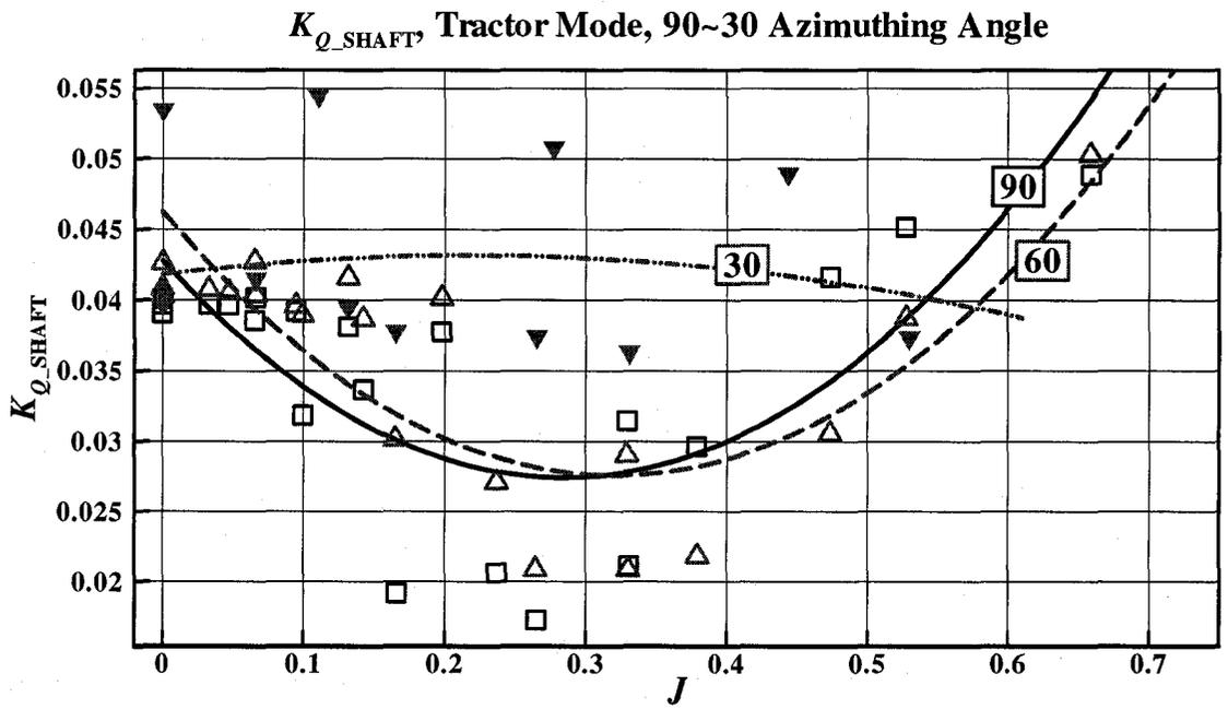
Figure B-16:  $K_{Q\_SHAFT}$  vs.  $J$  at various azimuthing angles (90–30 degrees) in open water
