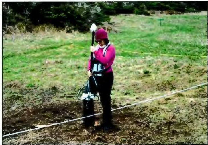
Figure 3.2: A proton magnetometer with two sensors. A continuous survey mode is employed (Image courtesy of PAC Project).
