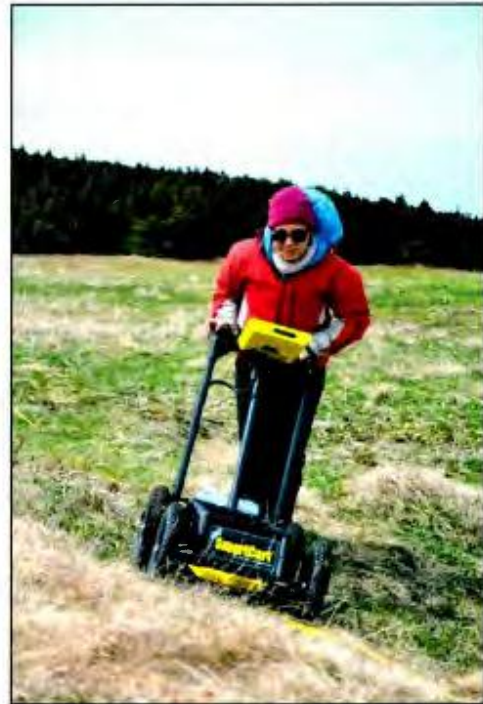
Figure 3.7: GPR with a 500 MHz antenna on a wheeled cart – the antenna is mounted on the bottom of the cart while the computer is mounted by the handle (Image courtesy of PAC Project).
