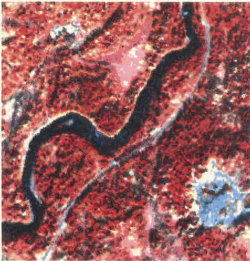
Figure 3-3(a): False Colour Composite (FCC) Image Band 3 (Blue) - Band 2 (Green) - Band 4 (Red) white/blue – no vegetation purple – wetland/shrub red – trees black - water
