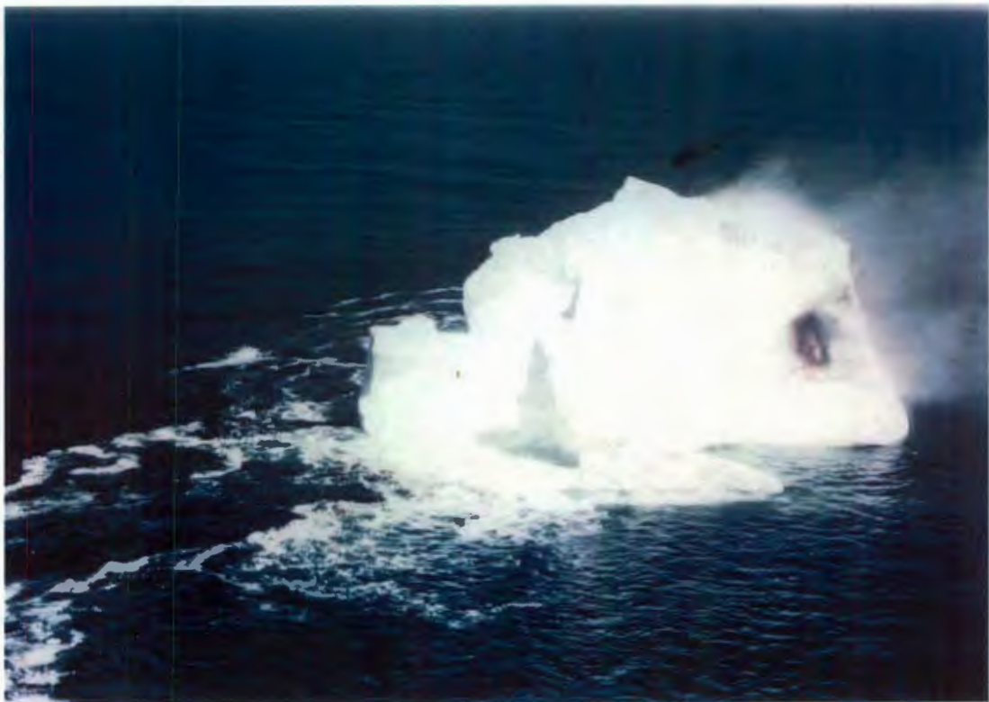
Figure 2.1: Thermite used on an Iceberg by the IIP
