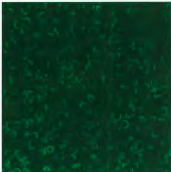
Figure 4.4: Confocal image of 0.99 \mu\text{m} spheres with the fluorescent dye (and p-xylene) not incorporated into the particles. In this case more ultrasonication is needed.
