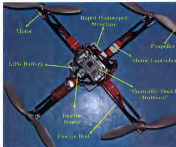
Figure 6.7: Photo of the Quad-rotor Platform
