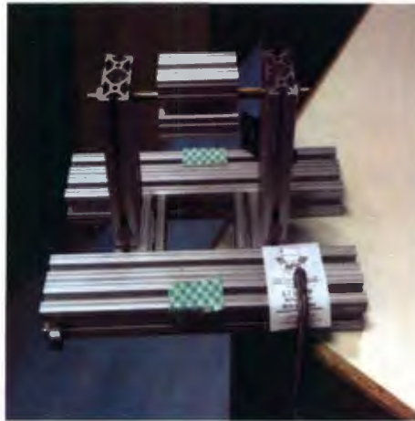
Figure 6.11: Test Bench Used to Tune Roll and Pitch
