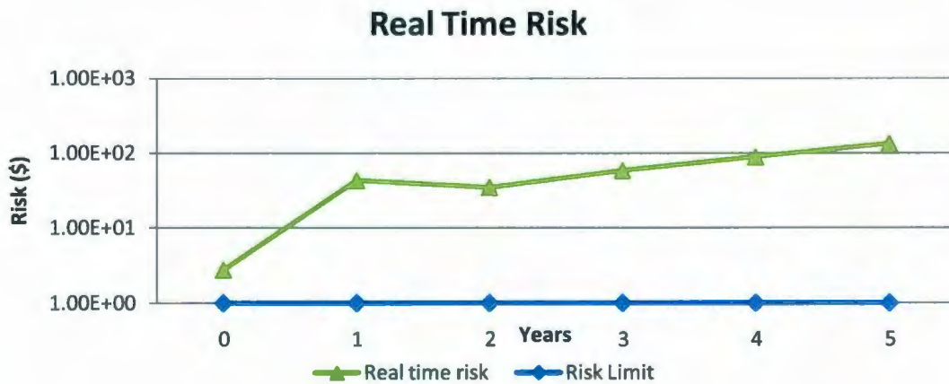
Figure 5-9. Posterior risk profile of the Flash drum unit over 5 years
