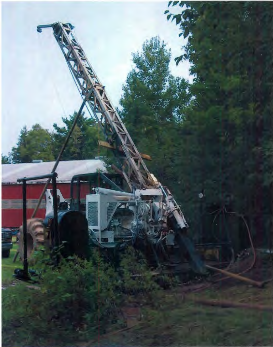
Plate C.1. Boart Longyear 538 diesel drill rig with an NQ / NW triple tube core barrel used for drilling the inclined boreholes.
