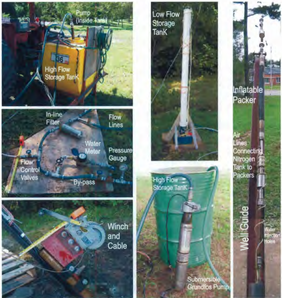
Plate C.2. Downhole packer test system set-up.
