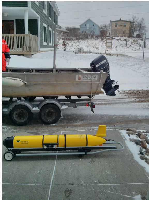
Figure 6.12: The Bonne Bay Marine Station's boat Freezy shown with the Slocum autonomous underwater glider during the parameterized trials in December 2013.
