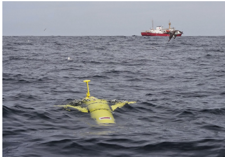
Figure 6.3: Launch of an autonomous underwater glider during the Labrador Sea experiments from the Canadian Coast Guard Ship Hudson's fast rescue craft. Image Credit: Robin Matthews
