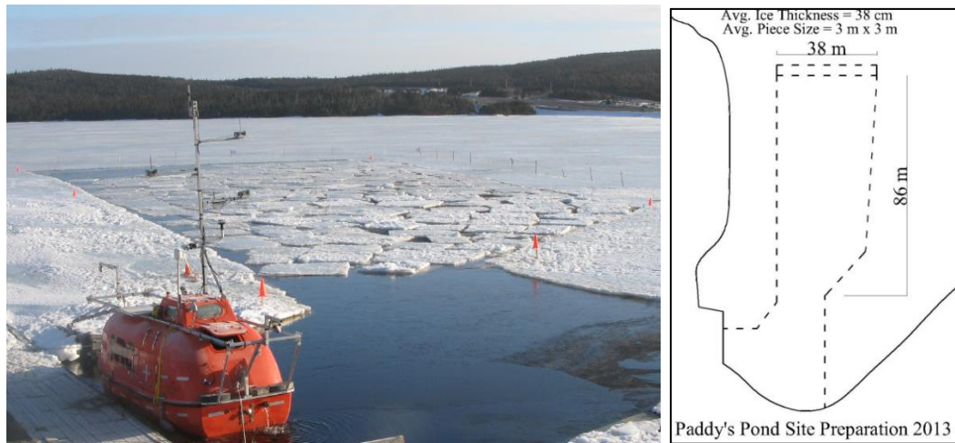
Figure 3.4: Prepared ice field for lifeboat trials
