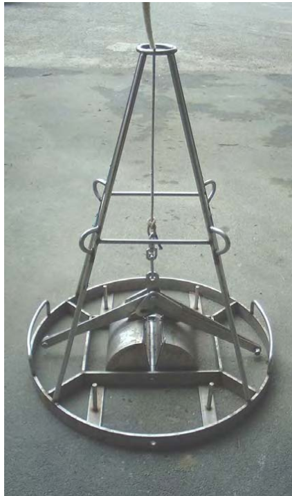
Figure 6.4 Example of spring-loaded grab sampler
