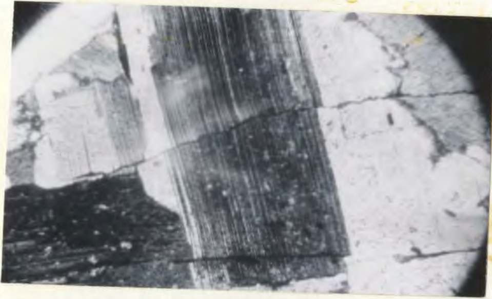
Fig. III: Fractured albite twin lamellae; note dragging of lamellae near fracture.
