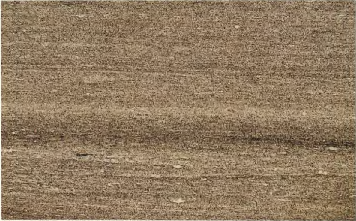
PLATE 4.3: Bedded pyrite from Schooner Cove. When undeformed the pyrite has this typical fine grained appearance. The dark layers are organic rich. x 2.5 magnification, reflected light.
