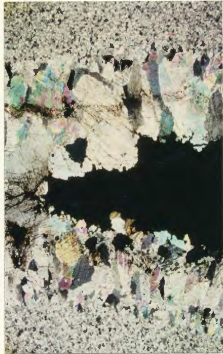
PLATE 4.10: Same field of view as PLATE 4.9 with polarizer in. Note the presence of pyrite on one side of the cavity which can be used to indicate way-up during mineralization.
