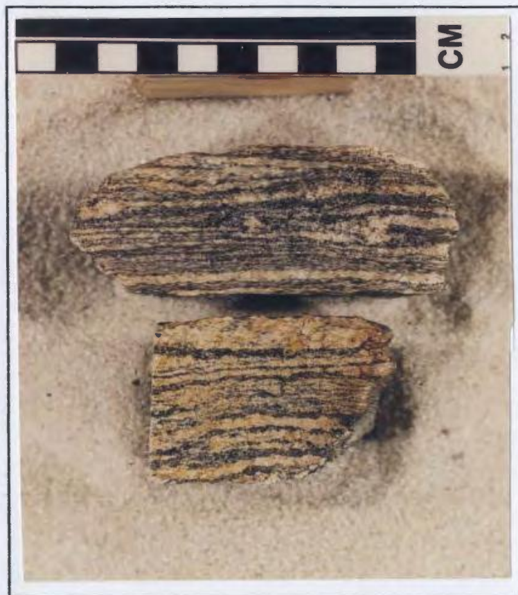
Fig. 3-2. Two samples of the metapsammitic rocks showing well-developed stromatic layering defined by alternating quartz + plagioclase ( \pm K-feldspar) + minor biotite leucosomes and biotite ( \pm garnet) + quartz + minor plagioclase melanosomes. Secondary muscovite and chlorite are common.
