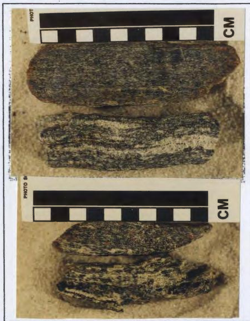
Fig. 3-6. Four samples of unshered leucosome-poor pelitic metasediments showing that generally the leucosomes are not as well-developed as those in the metapsammites (Fig. 3-2). Leucosomes are quartz + plagioclase + minor biotite + cordierite (in places) and melanosomes are biotite + sillimanite-rich in addition to garnet in places.
