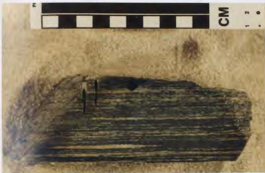
Fig. 3-8. Mylonitic fabric developed in shear zone rocks in the metapelite unit.
