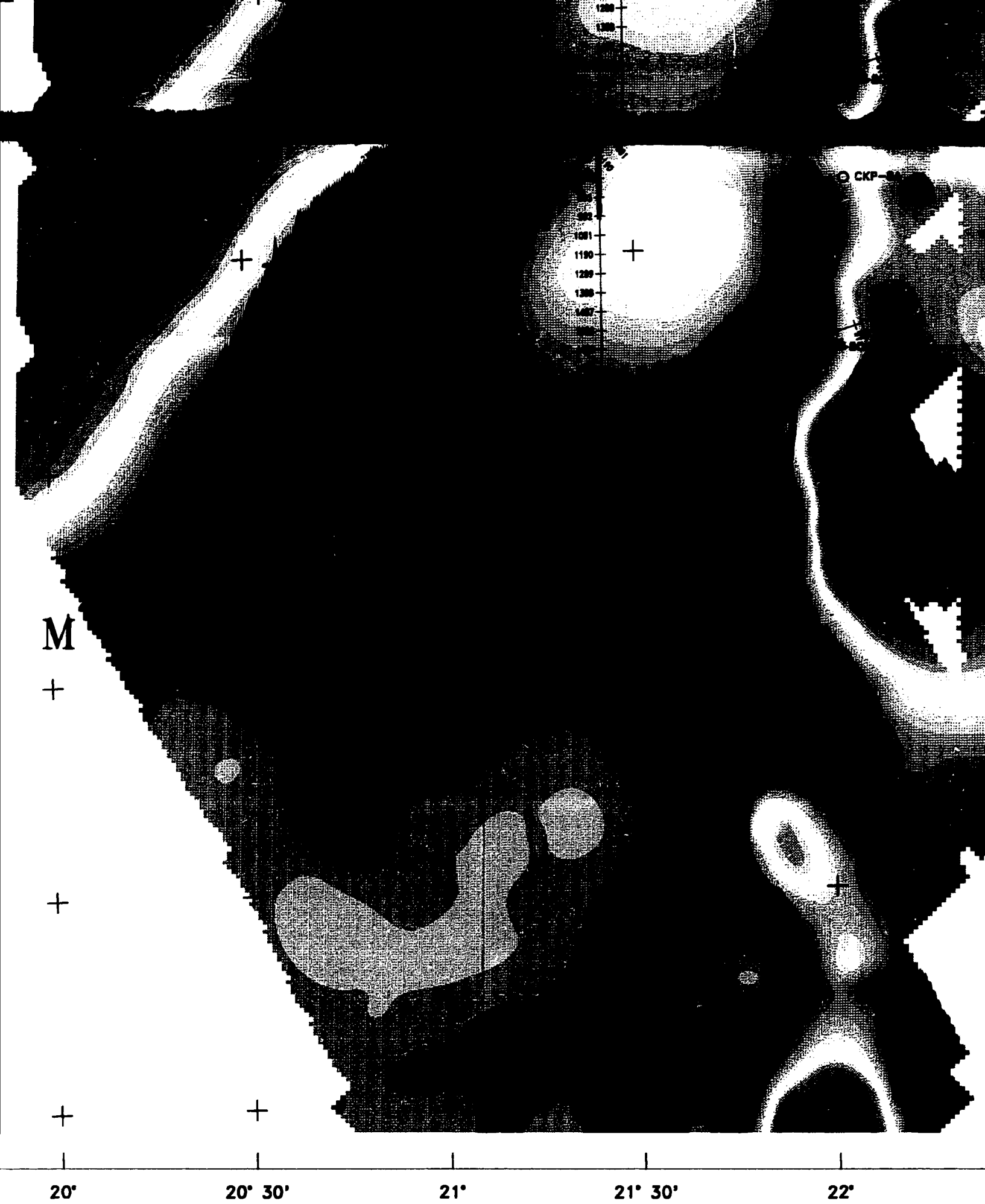
Figure 4.10 Bouguer anomaly map of the Nosop Basin, western Botswana (density = 2.67 g/cm 3 ).
