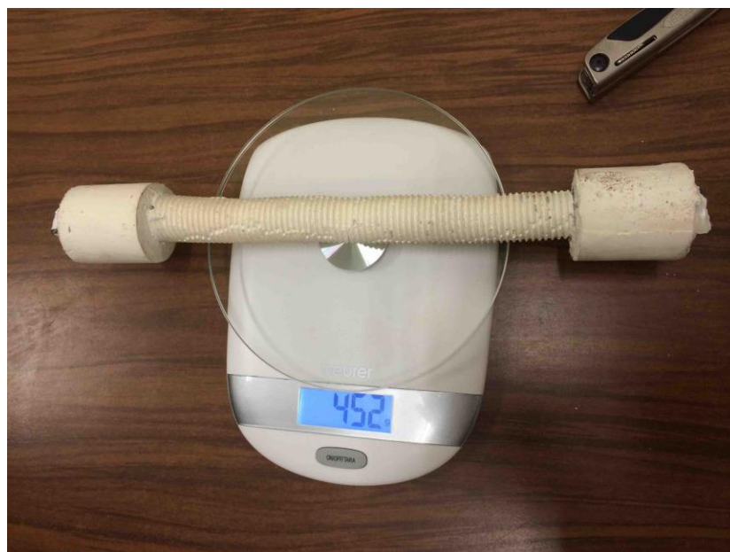
Figure 1. Weighing the E-Cat after the test (452 g). The ridges along the body of the reactor increase the dissipation surface for natural heat convection. The power supply cables run through the two cylindrical extremities (termed "caps"), and were cut prior to weighing.
