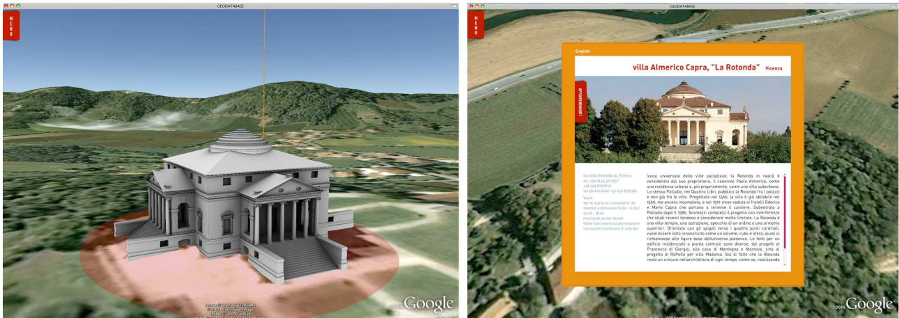
Figure 5: One of the models for the “Palladio 3D Geodatabase” and information card. The surfaces model - exported and displayed in GoogleEarth - has been highlighted by imposing an Ambient Occlusion shading.
