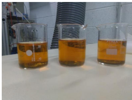
Figure 6.3: Photograph of the presence of iodide ( I_2 ) in the experiments without oscillations, with an acid concentration [H_2SO_4] = 1 \text{ mol L}^{-1} .
