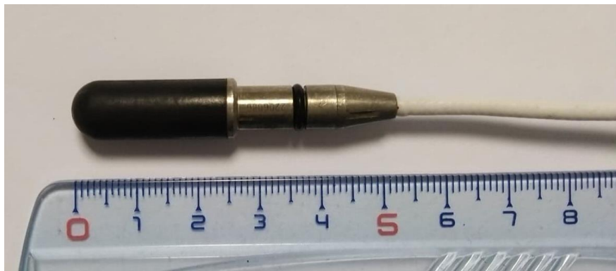
Figure III.12 : Photographie de l'hydrophone commercial B&K 8103
