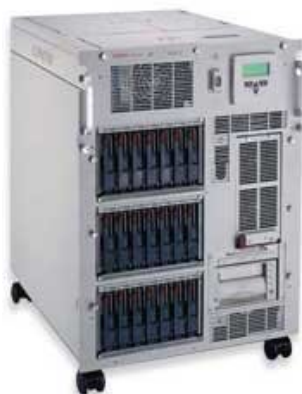
Figure 1. The Compaq Proliant 8000 SMP machine
