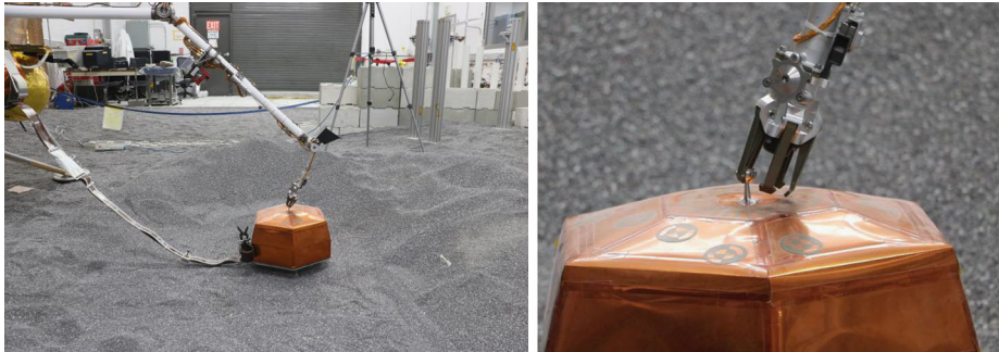
Fig. 29 SEIS Deployment (left) and grapple release (right)
