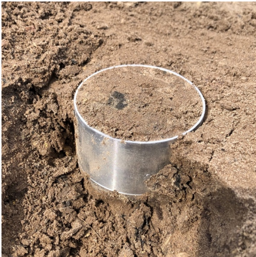
Figure 4. The cylinder in the soil after it was hammered down,
