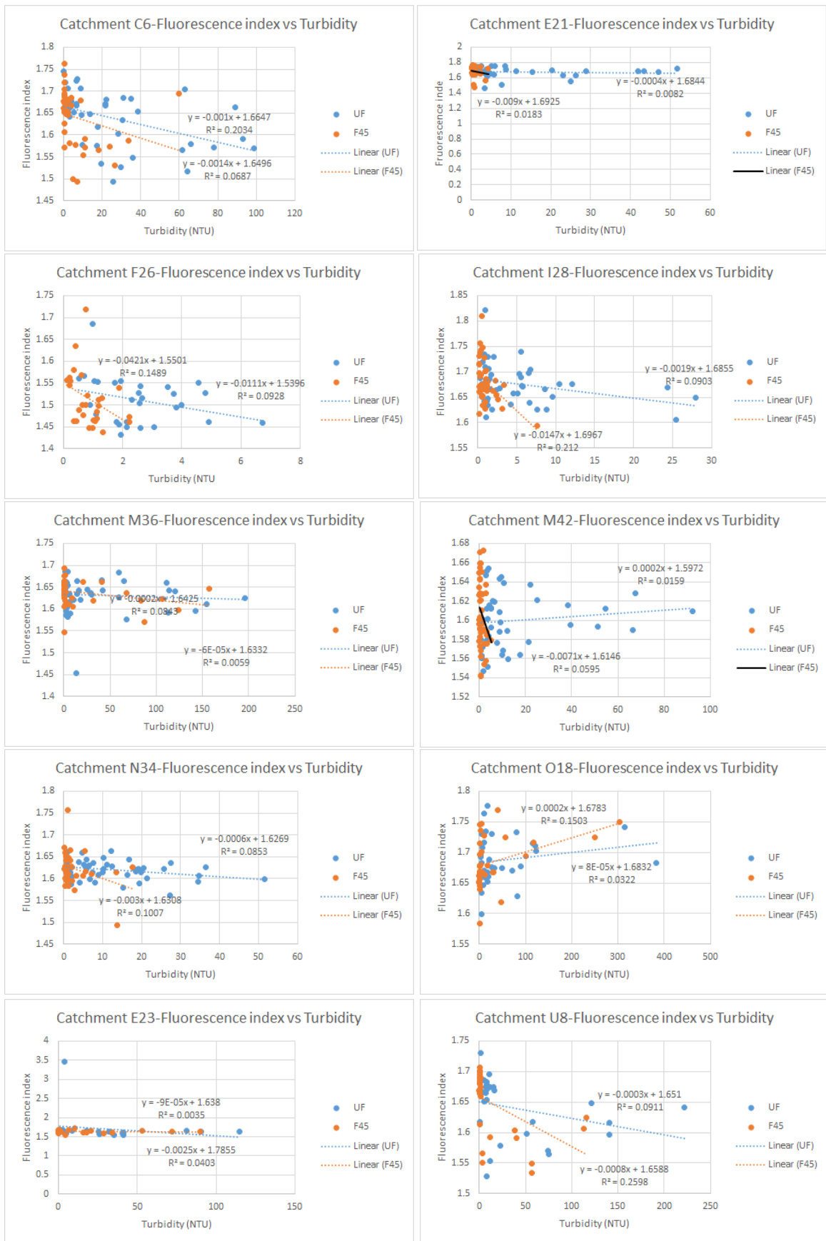
Figure 7. Plot illustrating fluorescence index vs turbidity for 10 study catchments, the graph shows a negative trend between turbidity and absorbance.
