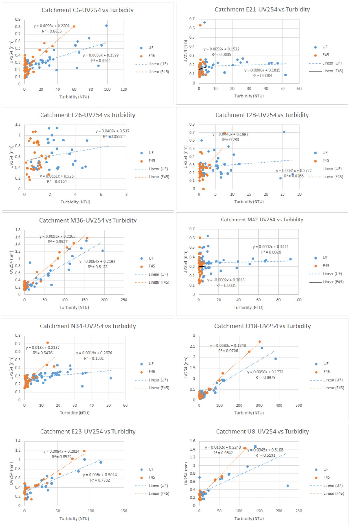
Figure 6. UV254 vs turbidity concentration for all 10 catchments, the graph shows a positive trend.
