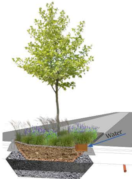
A rain bed construction.
