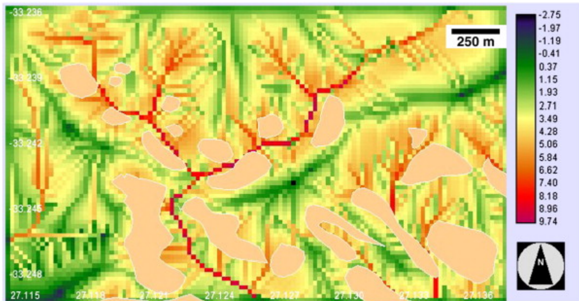
Fig. 7. An example of a gully vector layer overlaid on SPI surface. The solid rectangle in Fig. 1 shows the location of this area. Gullies lie predominantly in high SPI areas (legend represents SPI values).
