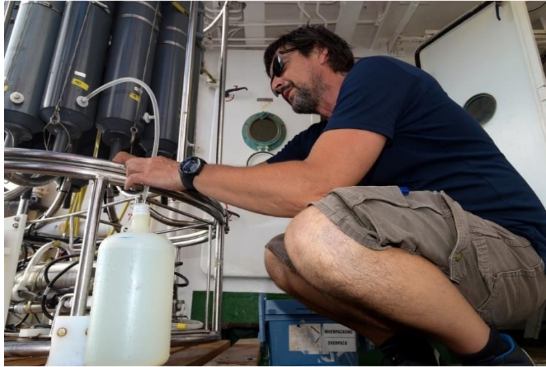
Figure 5.6-1 Samples of unfiltered seawater were collected along a depth profile in the upper 500 m of the water column by Niskin bottles that were mounted on the CTD. Photo: Mark Lenz.
