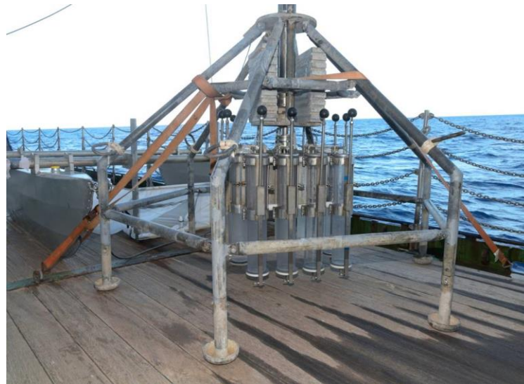
Figure 5.5-1 The multicorer on deck of RV Poseidon. Photo: Mark Lenz.
