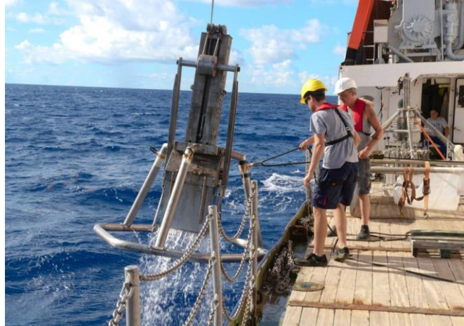
Figure 5.5-2 Recovery of the box corer after deployment to 3000 m water depth. Photo: Mark Lenz.
