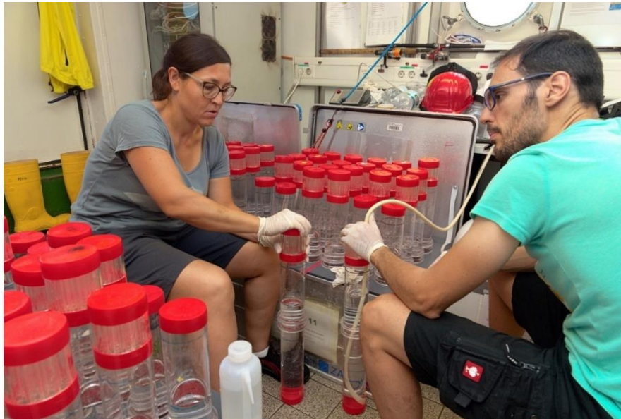
Figure 5.7-4 The seawater from the sediment traps was removed, while the brine fractions from 10 traps and the 2 blanks, which came from the same water depth, were pooled in one sample. Photo: Mark Lenz.
