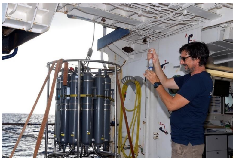
Figure 5.8-1 The CTD with the water sampler rosette. Photo: Mark Lenz
