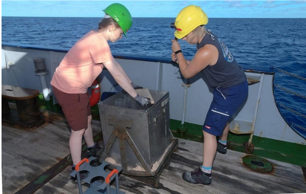
Figure 5.5-5 Taking liners from the box corer. Photo: Mark Lenz.
