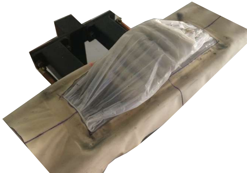
Figure 4-10: Detail on HDPE sheet and the latex sheet on top of the rods. When the oral cavity is filled with the fluid, the sheet is compressed against the rod's head.
