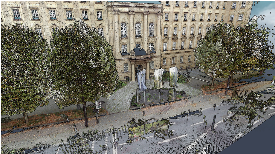
Fig. 2: Example point cloud from potree.org.
