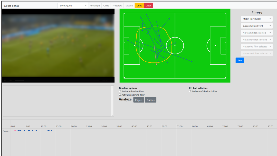
Figure 9.15 SportSense’s Web Client. The screenshot shows the result of a query for all successful passes which are kicked in the orange area. Each successful pass is visualized as an arrow on the field and listed in the time line. When a line or a point in the time line is clicked the video scene which shows the pass is played. The query has been performed while the match replay was still in progress (approximately after the first 15 minutes). The video area is blurred for privacy reasons.
