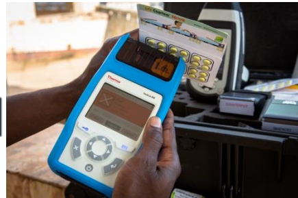
Figure 19 Raman spectrometer analysis of a Coartem ® tablet - Fail result and spectrum comparison with Coartem ® reference spectrum
