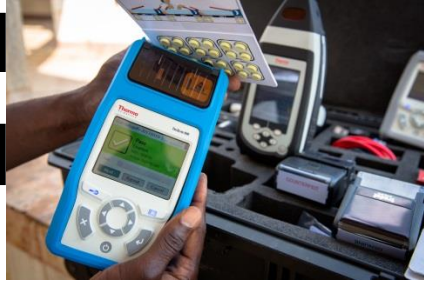
Figure 18 Raman spectrometer analysis of a Coartem ® tablet - Pass result and spectrum comparison with Coartem ® reference spectrum
