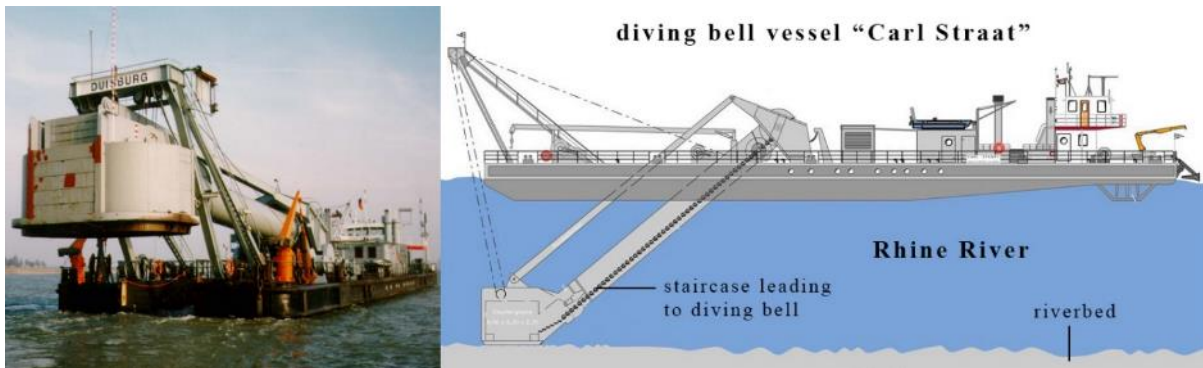
Fig. S1: Diving bell vessel “Carl Straat”. The riverbed can be accessed by foot through a staircase and diving bell that is open on the bottom. Water is kept out using a double door system and artificial adjustment of air pressure in the bell and staircase (0.1 bar per 1.02 m water depth). Images courtesy of the German Waterways and Shipping Administration (WSV), department Duisburg, modified.
