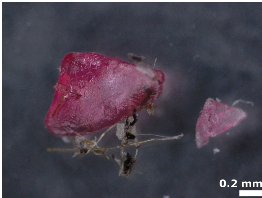
Fig. S5 Large (left) and small (right) PP particles after recovery
