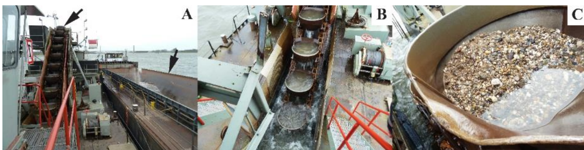
Fig. S2: Bucket chain (left arrow, A) vessel with accompanying transport barge (right arrow, A) with the Rhine River visible in the background at Rees, Germany (A). Bucket chain (centre) in action dredging riverbed sediments (direction of hauling: upwards, B). Close-up of sand-gravel riverbed sediment in the dredge bucket (C).
