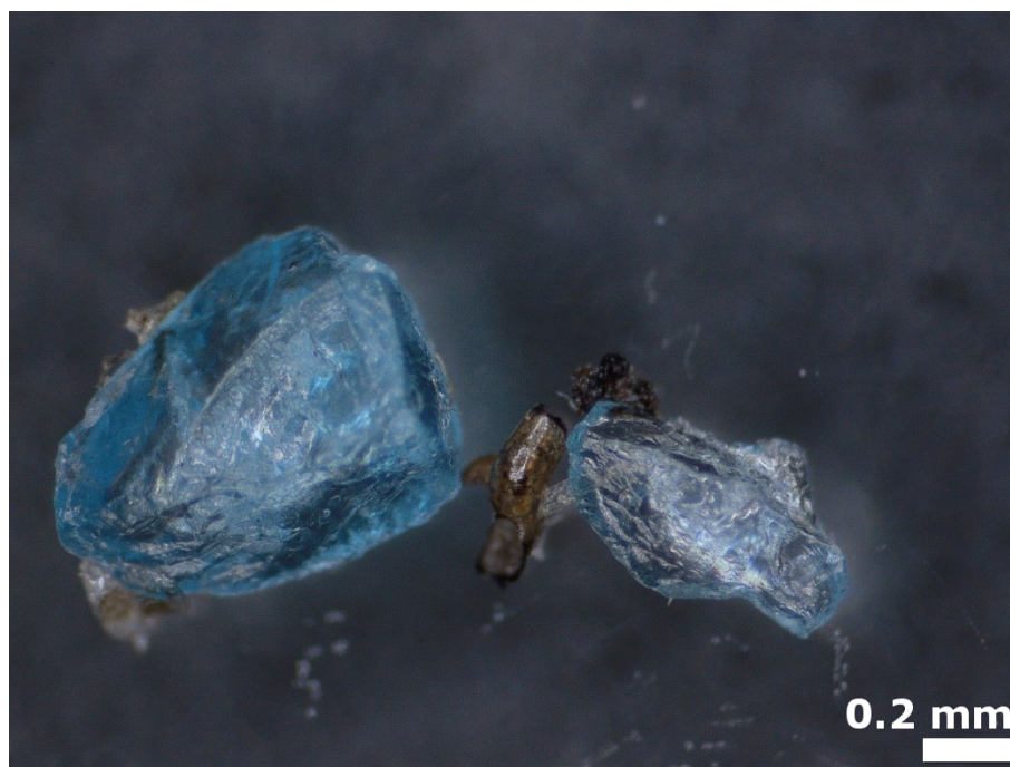
Fig. S7 Large (left) and small (right) PS particles after recovery
