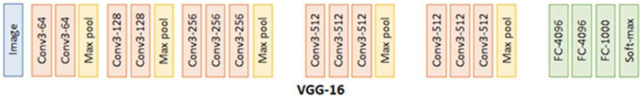
Fig. 1. VGG16 architecture. (modified from https://medium.com/coinmonks/paper-review-of-vggnet-1st-runner-up-of-ilsvlc-2014-image-classification-d02355543a11 ).
