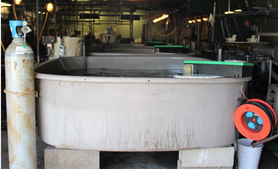
Figure 4: Adult fish keeping facilities at the PFOM-ARN, Ifremer Campus, Plouzané. Each tank is equipped with an automatic feeder and is connected to a seawater flow through system. Sea water pH is held constant by equilibration with pure CO 2 (bottle on the left).
