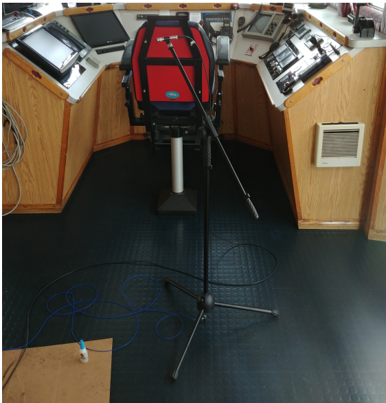
(a) Instrumentation setup to assess sound pressure levels L_{p,A} and velocity levels L_v during the sea-trials
