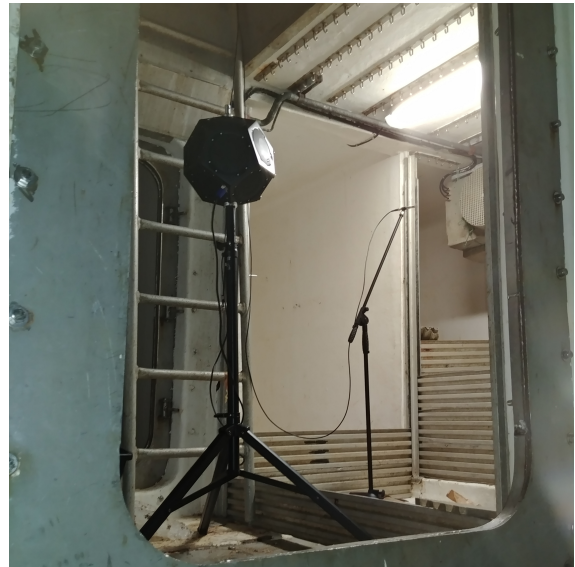
(b) Dodecahedron omnidirectional source and microphone during the measurement of the reverberation times
