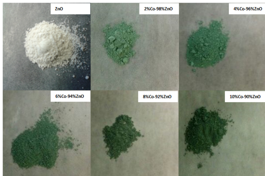
Figure 3.8: Color photos of ZnO and mixed phases of Co and Zn precursors heated at 200 °C.
